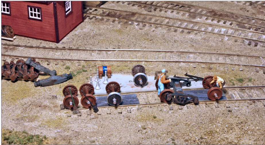
34. The scene with a wheelset replacement in progress. The two replaced wheelsets have silver wheel treads and oily black wheel faces. At left are some stored bolsters and side frames. Ties have been used to make “crossings,” where workmen can roll wheelsets on and off the rails. Note the shovel and broom resting against the new wheelsets at left, and brake beams at right.
