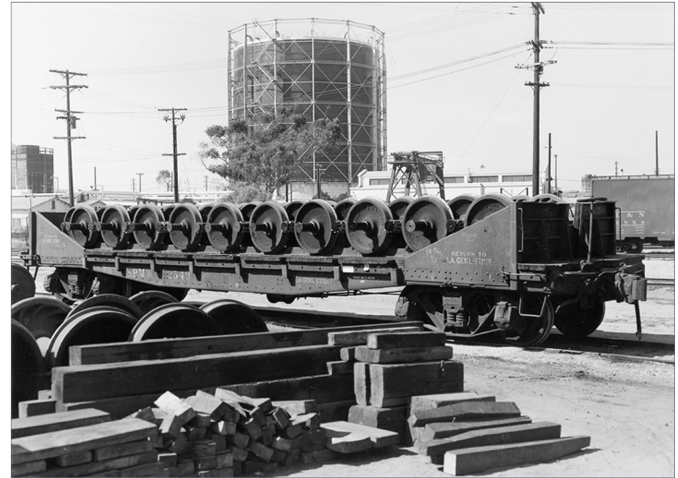
17. This Southern Pacific wheel car, modified from a Class F-50-3 flat car, has wheelsets staggered in two rows. There are about 20 wheelsets, making a total weight of about 47,000 pounds. The projecting journals are evident. The car, SPMW 2549, was converted to this service in 1943 from revenue car SP 40263. The photo was taken on September 19, 1954 at San Diego. Chet McCoid photo, Bob's Photo collection
