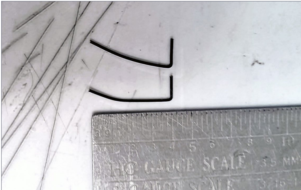
7. The sand hoses made from Details Associates 0.020" vinyl cable; actual length is about a scale 4'-6".
