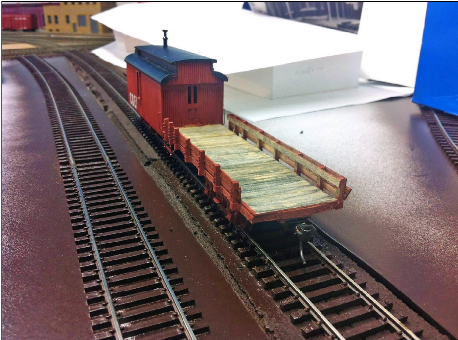
26-27. This picture shows the model on track to see how it performs on curves and through switches.
