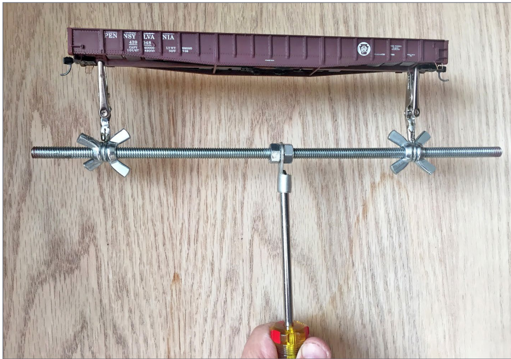
5. After using the handle, I made a modification. For my Mark II version, I added wing nuts to make it easier and quicker to adjust the spacing. It's shown here with an E&B Valley 65-foot mill gondola. ✓
