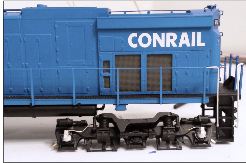
5. The completed side frame ready to remount to the trucks.
