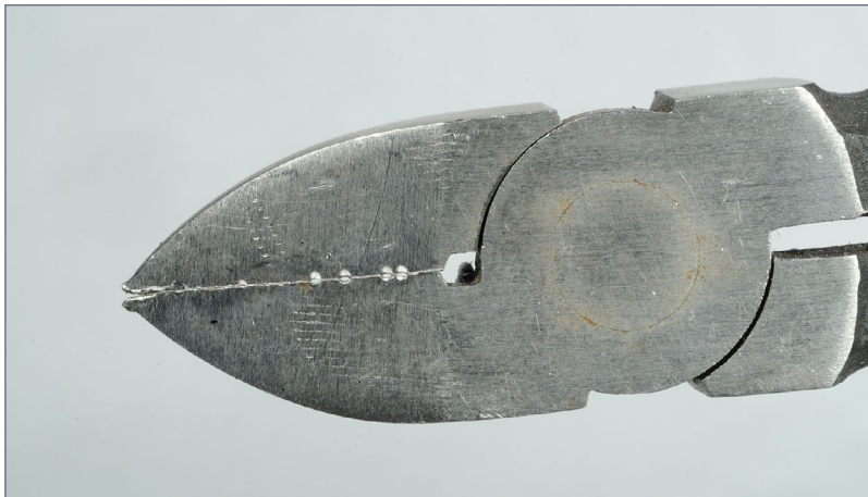
13. The flush side of my economically priced red-handled flush cutters shows what can happen if you use them to cut hard steel wire such as music wire. The jaws of flush cutters are too thin for such hard materials.
