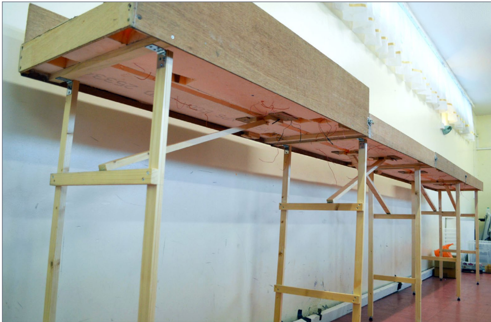
12. Here's the module in basic form: the integral legs fold up underneath the boards.
