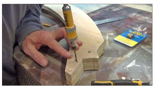
18. I drilled holes through the lift-out ends and the plywood that was cut to match the ends and would act as a base in the foam. These holes ensured that the magnets would match up.
