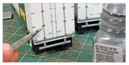
12. Before starting the weathering process, I need to address a minor detail item. The prototype photo shows the extra set of door latch rods on the rear doors required for trailers in TOFC service. To model these, cut .012-inch diameter brass rod and mount these to small styrene bits. Use a small brush to carefully paint the rods using classic Testors silver paint.
