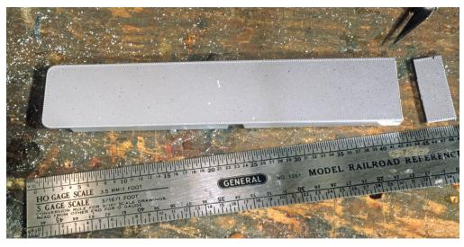
5. Next, remove the same amount of material from the rear of the roof piece.
