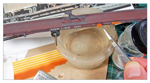
32. Now apply freshly painted patches on the 5593 and on the 5593. On the 5593, I decided that Reefer Orange will best capture this look. Use an airbrush to paint a scrap of Champ decal material. Use a #11 X-Acto blade to cut out the right size patches and apply these as a decal.
