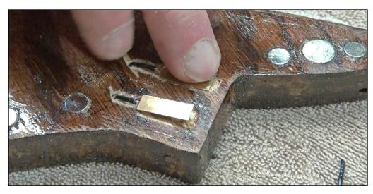
27. A piece of 1/32 x <sup>1</sup>/<sub>4</sub>-inch brass stock cut one inch long forms the power contacts to feed current to the rails in the lift-out section. These contacts were placed in a carved-out space to fit almost flush. I soldered wires to the contacts, then fed the wires through the plywood to the rails.
