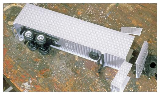
4. After removing this section, sand the edges for a square joint before using liquid cement to re-attach the body pieces.
