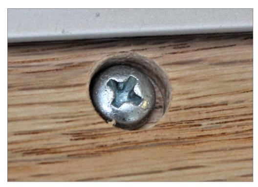
2. One of two screws holding the handle to the body. It is recessed to prevent marring the material being cut.
