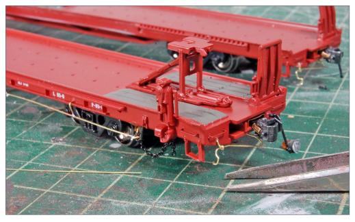
25. Use .012-inch brass wire and bend and cut coupler pin lifters.
