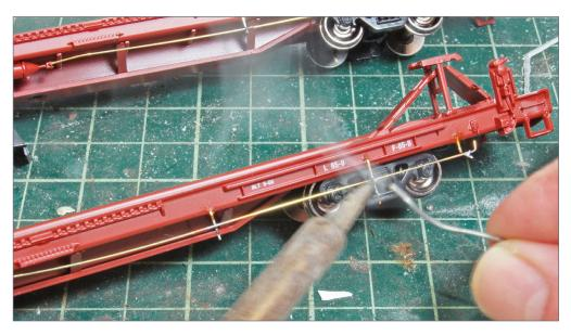
23. Follow the prototype photo of Soo 5583 to install the handbrake linkage detail. For this, use .015" brass wire. Solder this 30-foot length of wire to three short sections of wire which are glued into #76 holes. After soldering the horizontal length of wire to the hangers, cut the hangers flush. Soldering makes for a sturdy and realistic looking installation.
