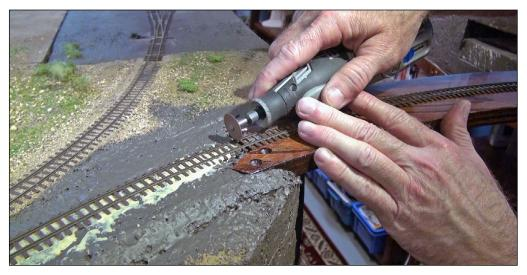
26. I cut the track on each end with a Dremel cut-off wheel. I left an overhang of 1/16 of an inch to ensure a clean lift-up.
