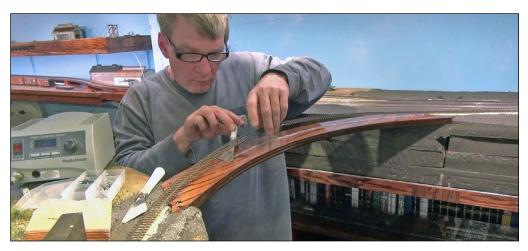
25. I glued Code 70 Micro Engineering track to the foam with Liquid Nails. I attached the track to the plywood lift-out with clear silicone caulk, using a painter's knife to spread the glues. The fact that Micro Engineering flex holds its shape after being curved made it easy to match the ends to where it would join my main lines on both layout approaches.
