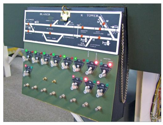
7. Bob uses localized CTC-like control panels for switch routing and occupancy indication.
