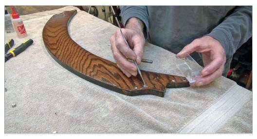
21. After staining the wood and applying polyurethane, I mixed 5-minute epoxy and placed this in the holes where the magnets would be glued flush in the wood.
