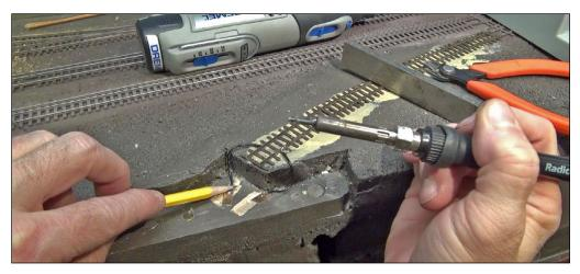
28. I also placed contacts in the base plywood in the end that adjoins my around-the-room home layout. These contacts were soldered to wires that pick up current from the rails.
