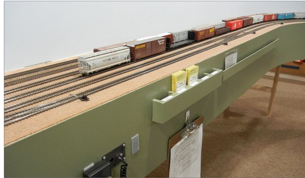
4. Rob Spangler installed cork rolls with contact adhesive intended for laminate countertop material. Here's one area before ballasting. The cork provided a nice, smooth surface for laying track compared to plain plywood. Rob Spangler photo
