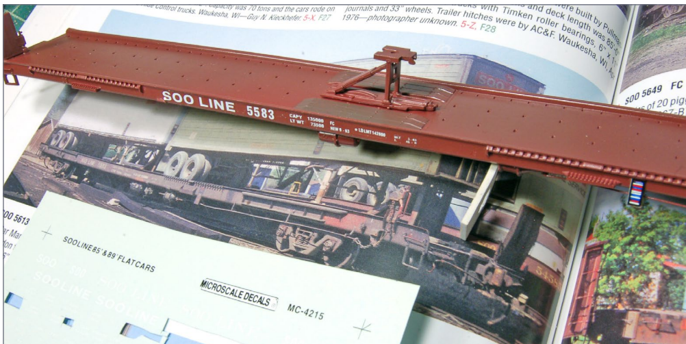
29. Study the photo of the 5583 and apply decals to match the prototype. To faithfully capture the correct look of the prototype car, I simulate the areas where data has been patched out and re-applied on these newly painted areas. Before attempting to capture this look, weather the cars.
