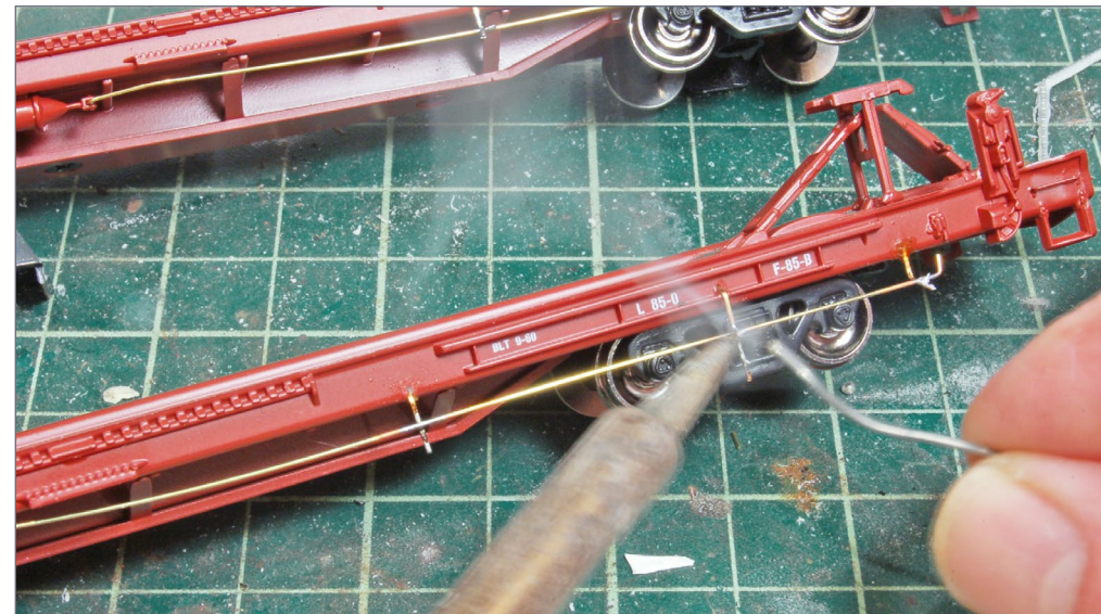
23. Follow the prototype photo of Soo 5583 to install the hand-brake linkage detail. For this, use .015" brass wire. Solder this 30-foot length of wire to three short sections of wire which are glued into #76 holes. After soldering the horizontal length of wire to the hangers, cut the hangers flush. Soldering makes for a sturdy and realistic looking installation.
