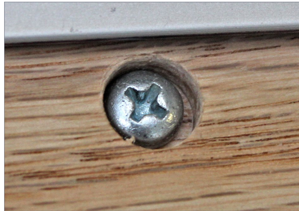
2. One of two screws holding the handle to the body. It is recessed to prevent marring the material being cut.
