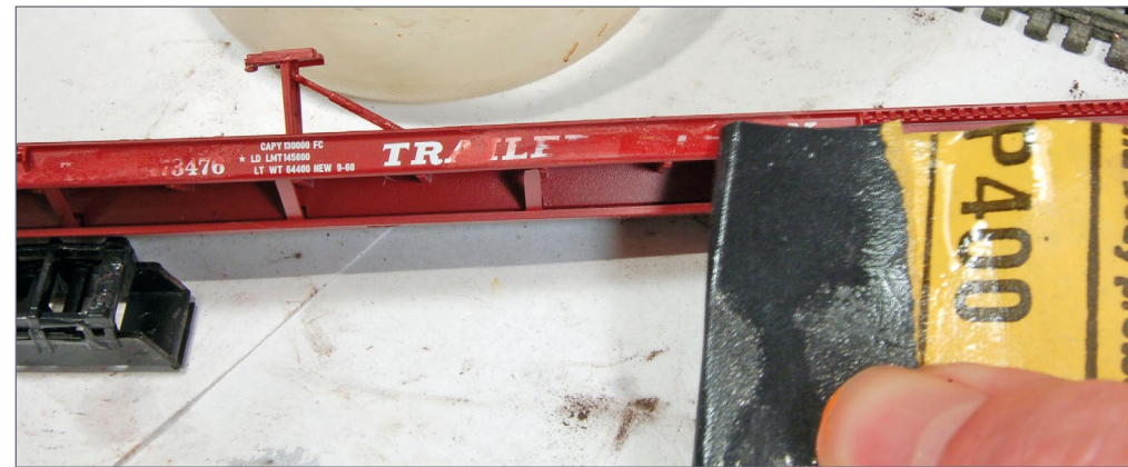
22. Remove the lettering using wet/dry 400 grit sandpaper.
