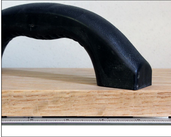
3. Side view showing the handle and the double-side foam tape that affixes the yardstick sections to the body.
