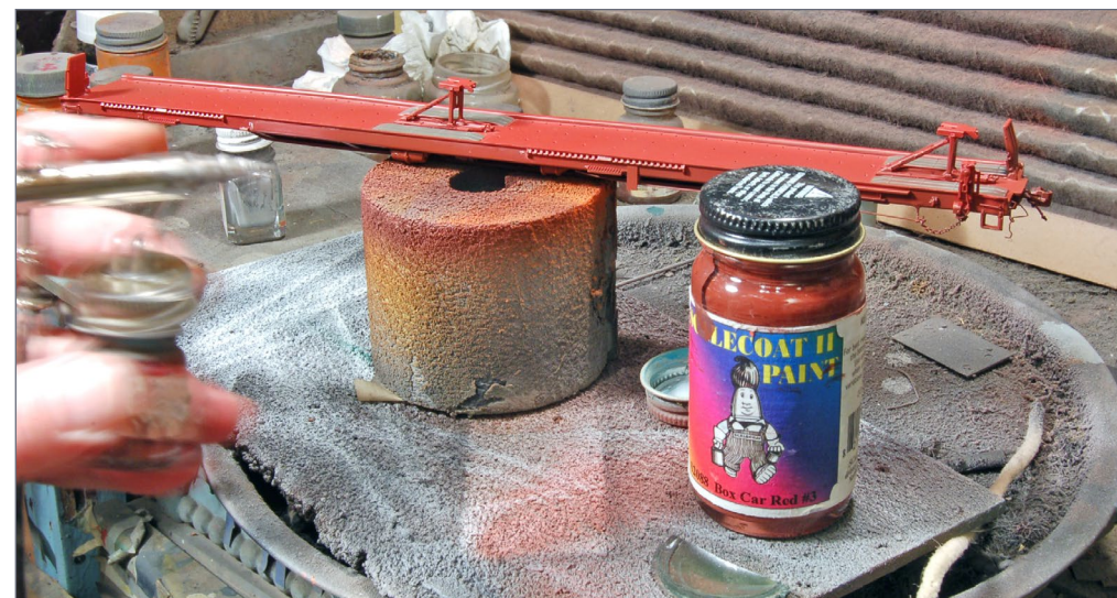
27. Scalecoat II Boxcar Red paint is the perfect paint for this project. When dry, the gloss finish provides the ultimate surface for applying decals.
