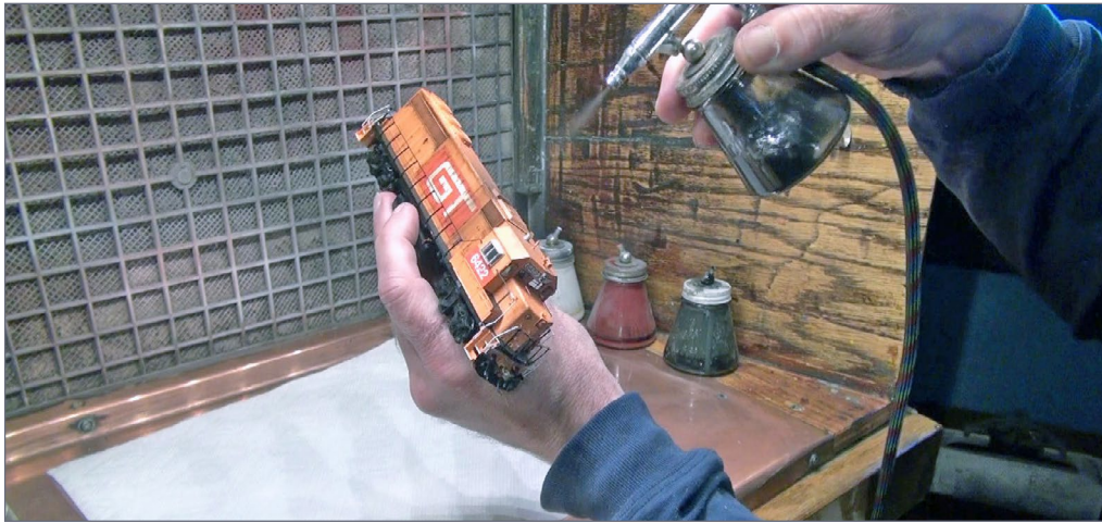
12. Finish the roof of the model with a thin coat of locomotive exhaust. Thin Model Masters black paint 90 percent, then use an airbrush with 20 psi pressure to slowly build up paint.
