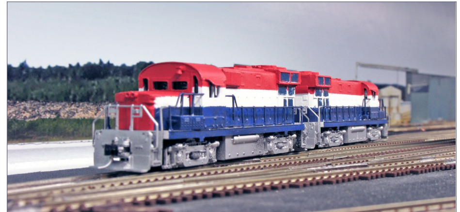
26. Original RS-11 fuel tanks are too wide and require modification.
