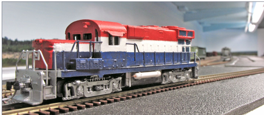
29. Cylindrical air reservoir mounted on left and right side of underframe. Angular waste oil retention tank is mounted on right side only (see 30a, 30b).
