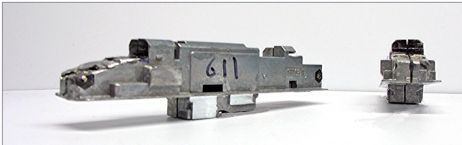
22. Reduce width of frame fuel tank area by filing it down. Original width illustrated on right.
