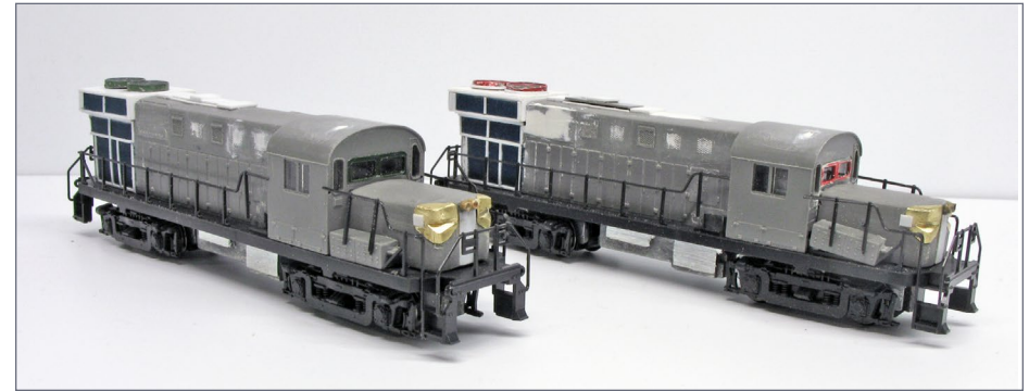
23. Nose modifications included removing molded details, filling corner notches, adding headlight housing, access door and site hatches.
