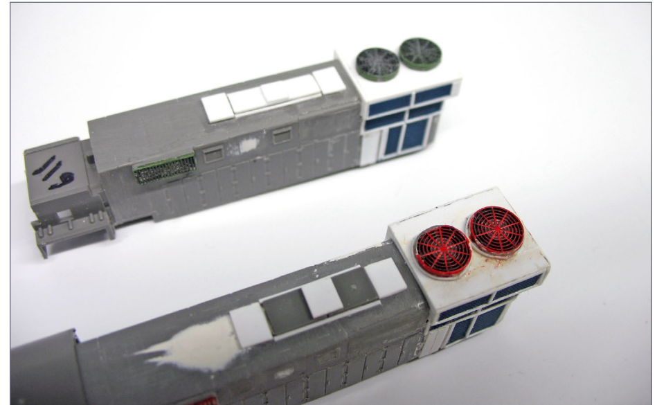
9. Form roof hatch detail from removed RS-11 details and strip styrene. Top unit has roof hatch detail built entirely from styrene. Bottom uses a combination of salvaged RS-11 hatch detail and styrene.
