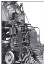
Boiler tube with widely spaced handrails
