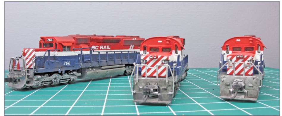
32. The final detail. Original RS-11 front and rear handrails (right) were replaced with EMD-style ones (center) as on SD40-2 #766 (left).
