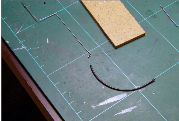
14. I used AWG 24 copper wire to form the piping. For pipe flanges, I used small pieces of wire insulation.
