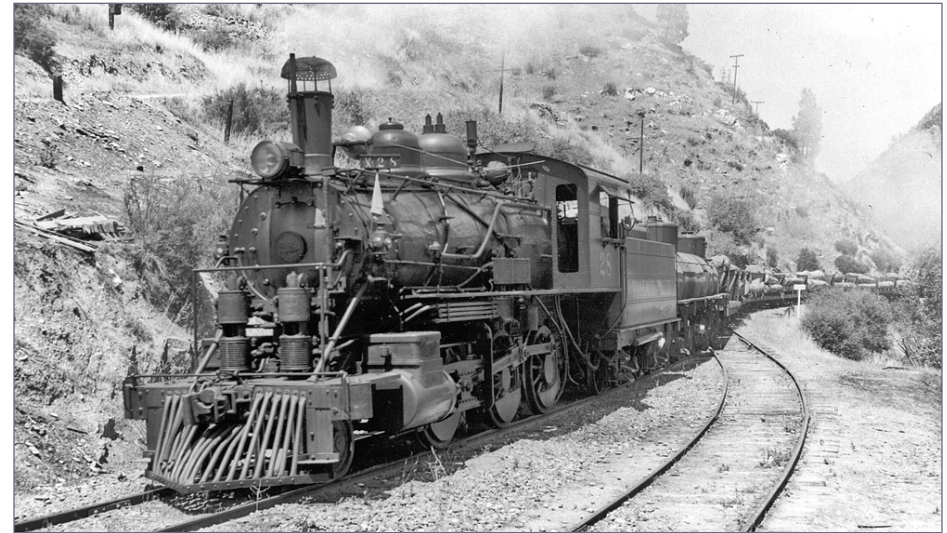
29. Extra 28 drifts past the siding at Briceburg with white flags and indicator board inserts indicating that it was an extra. The train indicator boards, typical of those used on the SP, were internally lit, although those on the YV had room for only four characters while the SP boards had space for five. The crew had a set of inserts which included the locomotive numbers, train numbers, 2nd and 3rd for sections, and an "X" for extras.
