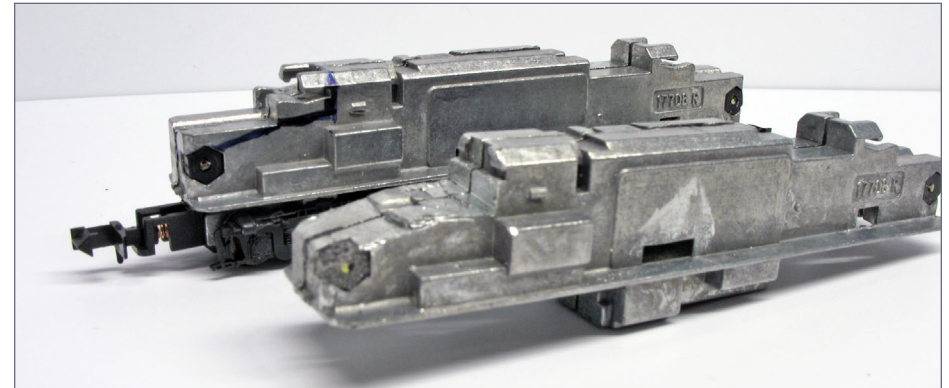
18. Original RS-11 frame marked for cutting (rear) and after cutting down the nose profile (front).
