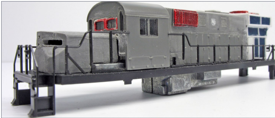
20. Nose section should fit firmly over modified frame.
