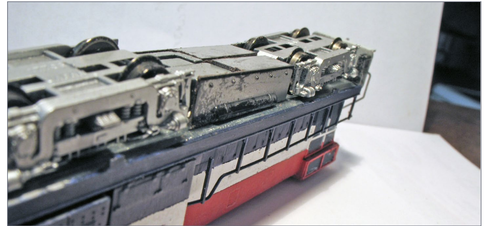
28. Fuel tank halves glued to frame.
