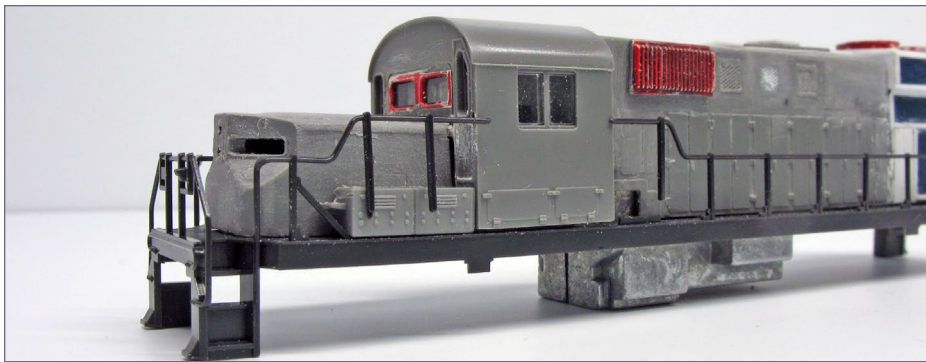
21. Battery boxes should remount over frame as shown.
