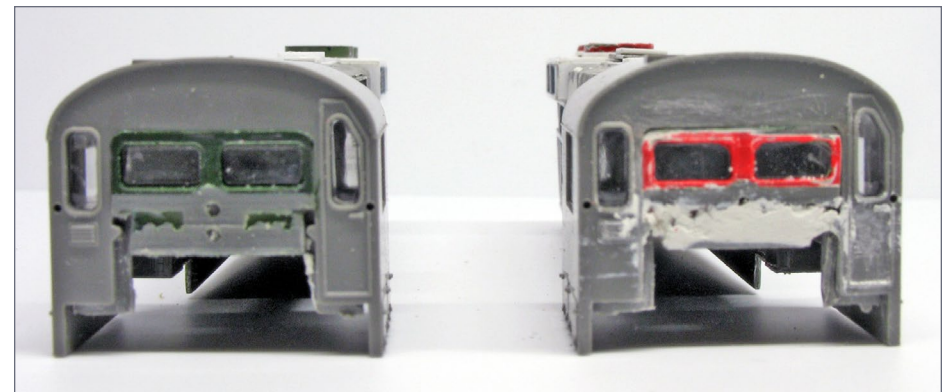
16. Kato SD40-2 cab window frame sections are mounted into the cab face.
