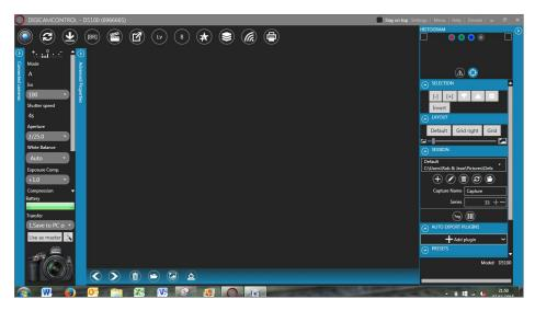
7a-b. (Top and bottom) Digicamcontrol is an example of software that allows you to control your camera from your laptop. It's also great for taking automatic multiple focus shots for still photography "focus stacking."
