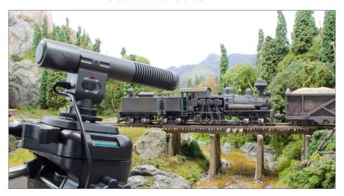
9. An external microphone is preferable to using the camera microphone. This directional condenser microphone was very inexpensive.
