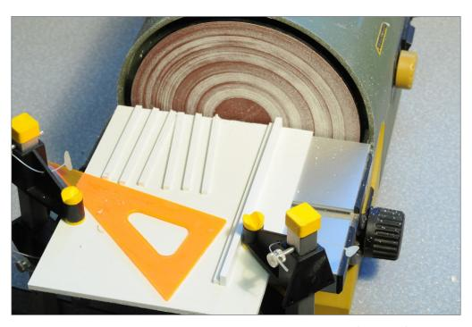
9. This simple jig makes it easy to produce a set of posts for a framed-bent trestle. The YV trestles used four posts and the jig has slots for two vertical posts and two battered posts. Putting the slots for similar posts next to each other saved room on the jig.
