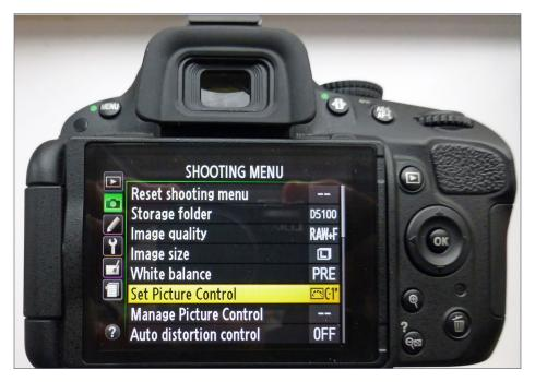
2. I recommend using "custom" picture control. Note that sharpening and contrast are set to minimum and saturation one notch above minimum. You may need to experiment using your own camera.
