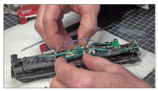
19.... and replaced it with the TCS decoder, plugging this into the 9-pin harness.
