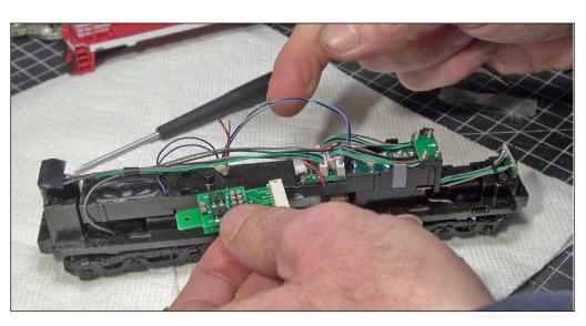
18. I pulled out and removed the locomotive's DC circuit board attached to the 9-pin harness . . .
