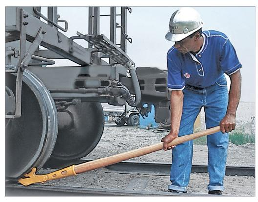
2. A manual car mover, sometimes called a railcar jack, allows a worker to move a car on level track. Shove the tool in between the railhead and the wheel, and push down. The joint at the head of the tool multiplies worker's efforts through compound leverage. *Aldon Company Inc. photo*
