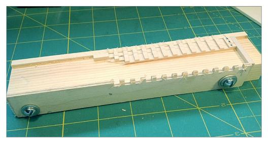
13. This wooden jig was clamped to a milling machine table so that notches could be milled into the guard timbers. All of the guard timbers were milled at the same time—four of them are still in the jig.
