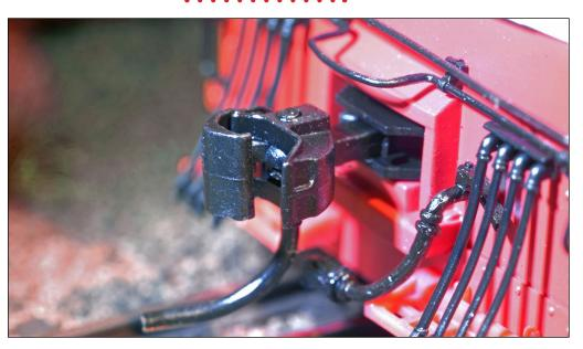
21. One thing I noticed while putting the shell back on the locomotive was the new-design metal coupler with the knuckle spring built into the assembly. Pretty neat!
