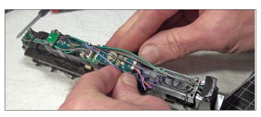
20. I plugged the speaker and keep-alive in to the decoders rear harness. That was it! Simple plug and play with no soldering. It took nine minutes from start to finish. I did the second locomotive sound and decoder installation in six minutes. Totally true.
