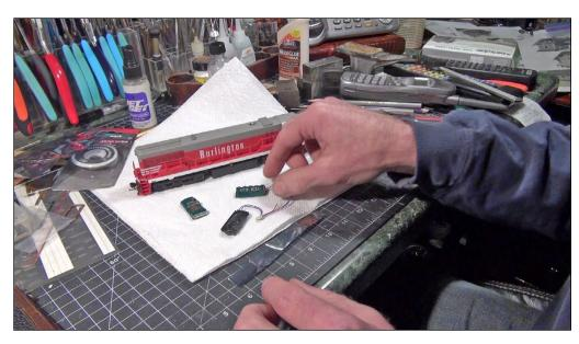
15. Korea Brass USA sent me locomotives without sound so I could demonstrate what goes into the sound decoder installation. Here you see the three components necessary for the conversion: a TCS WOW Sound 101 decoder, a keep-alive module, and a 16x35mm WOW speaker.
