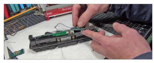
16. I removed the spring lighting contacts to install the keepalive in the locomotive's front speaker enclosure, then reinstalled the lighting contacts.
