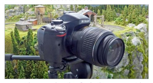
1. I use a Nikon D5100 shown here fitted with 18-55mm VR Kit lens which is very versatile. I also use a Nikkor 35mm f/1.8G prime (no zoom) lens, for better light capture in more challenging situations.
