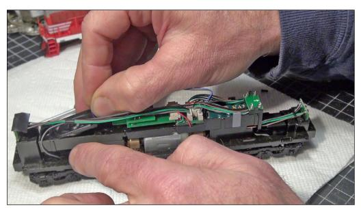
17. Using a little Walthers Goo, I installed the WOW sound 16x35 speaker into the locomotive's rear speaker housing.
