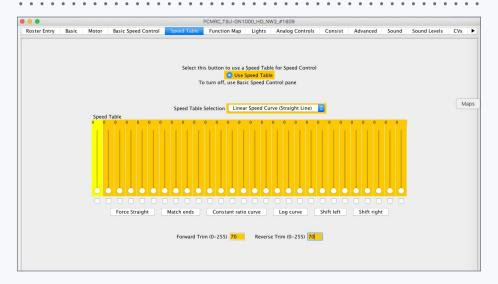
9. DecoderPro Screen shot - limiting top speed to 70 (out of 128), or about 60%
