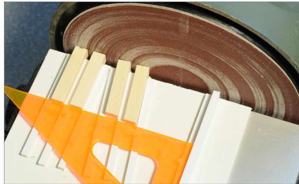
11. All four posts are then turned end-for-end and reinserted into the slots in the jig.
