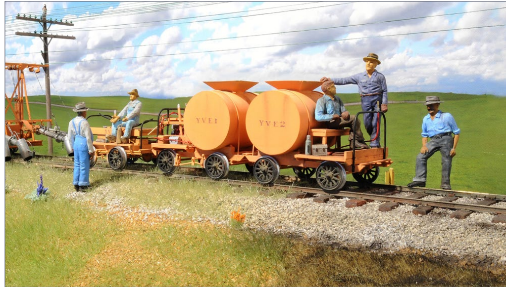
24. From left to right, the Fairmont ST2-D speeder, the T27 extinguisher car, and the T28 trailer. All of the figures are from Buffalo Landing.
