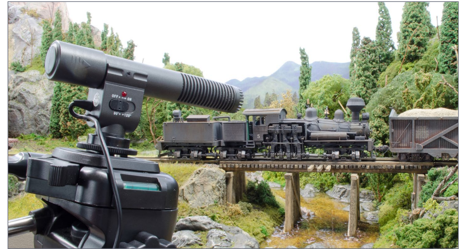
9. An external microphone is preferable to using the camera microphone. This directional condenser microphone was very inexpensive.
