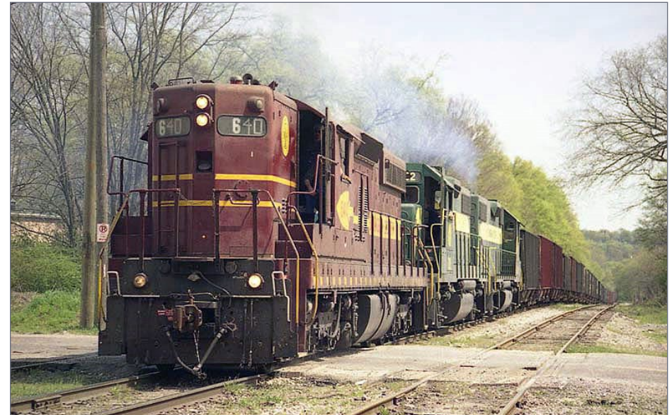
7. BSRR Northbound taconite train BS1 General has just departed BNSF'S East Thomas Yard after BNSF interchanged a U-SEMBIR taconite train with the BSRR. The BSRR takes the taconite trains to Flint Ridge for U.S. Steel. On the point is SD9 640 still in DM&IR Paint with BSRR patches. Second locomotive is BSRR 702, a GP38-2 in Birmingham Southern green and yellow scheme. William H. Davis collection. Posted on rpicturesarchives.net
