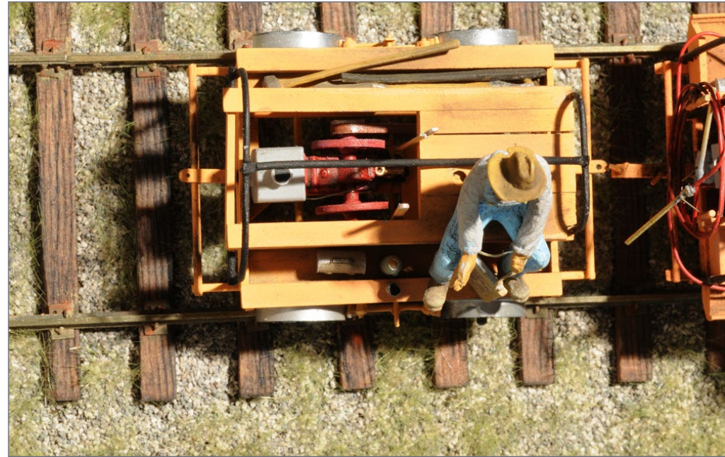
20. The Fairmont single-cylinder engine and radiator on the T27 extinguisher car were made using rapid prototyping technology. Together, they measure about 5/8" long. The same technique was used to make the vintage Thermos bottle and lunch box barely visible in the storage well to the left of the operator's leg.
