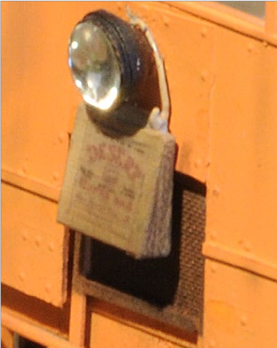
21. This Desert water bag measures about 1/4" square and is another detail made using rapid prototyping. Wire was added for the rope and the part painted before adding a decal made from a photo of a real Desert water bag found on the Internet.
