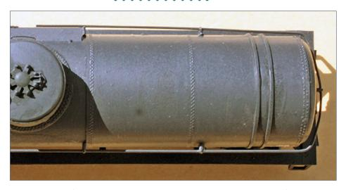
5. The top of an Athearn tank car, converted to circumferetial double-row rivets using Archer set AR 88031. That set was designed to reproduce exactly this kind of double-row rivets.
