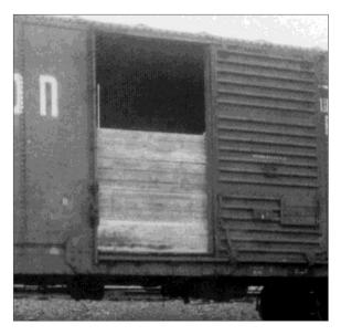
53. Boxcar fitted with boards for hauling grain.
