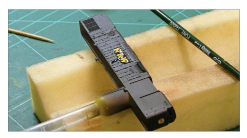
24. Applying more Micro Set helped the decal flow on the engine body for easy alignment.
