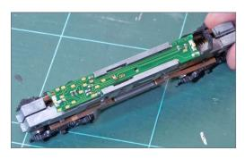
6. The decoder now fits in tightly. The motor contact is provided by the two long-hole notches on the decoder board.
