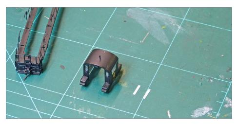
7. I cut to length .010" x .060" styrene strips. The molded gutter helped align the sun shades at the proper angle.
