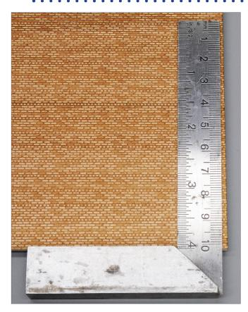
5. (Top) After removing the misaligned row of brick, you must reestablish a square end on the sheet. It is a good practice to verify that all sheets are square with the mortar lines.
