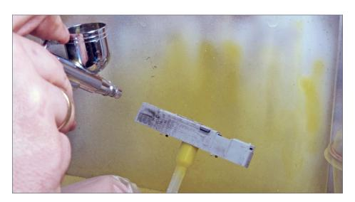
19. The engine body in the paint booth. A disposable plastic pipette helped as a holder.
