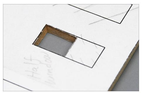
26-27.Use the fabricated half-window to mark the bottom of the sill, and then cut out the opening.
