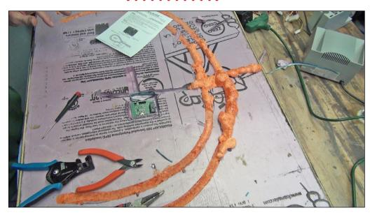
12. Another groove in the bottom of the diorama carries power wires to the turntable's microphone jack in the center of the pit. I installed a Digitrax AR1 power reversing module in line to the pit to keep the bridge from shorting out when spun around, reversing the polarity of the locomotive.
