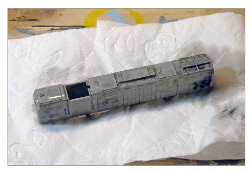
17. The still-wet body after the paint was removed. The black areas needed to be rubbed with a brush to remove all of the paint, but for repainting in black, it is sufficient to leave it.
