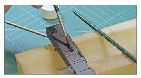
22. I applied some Micro Set to the decal's location. This helps in aligning the decal.
