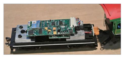
3. BlueRail Trains' first board is plug-compatible with DCC locomotives using a 9-pin JST connector.
