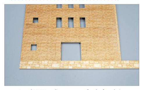
52-54. I used MMW medium cut stone for the foundation on the 1890 building. Slice off a strip of the appropriate width foundation. Use a machinist's square to mark the end at a 45° angle. Using a sharp razor blade, rough-cut to the line and then finish by sanding. Then determine the length of the foundation and bevel the next end.
