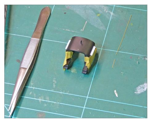
10. Cut-to-length brass wire. To make the straightened wire, I picked up a piece of rolled wire with two pairs of pliers, and gently pulled it apart until it stretched a bit.
