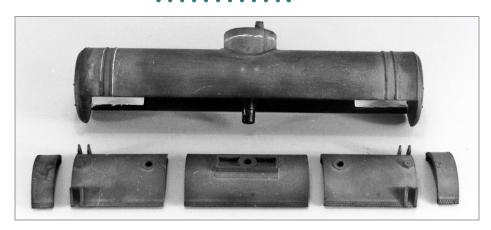
18. The cut-down tank parts for Richard Hendrickson's model. The top has already been reassembled and dome height increased as in [3]; the modeling putty at joints alongside the tank hold-down bands is visible. The bottom sheet had to be cut into five pieces also. "Fins" on bottom sheet were removed. (Richard Hendrickson)
