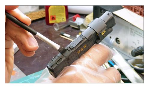
30. I used a medium-soft brush to put some of the black powder around the exhaust, streaking it outward to the roof edge.
