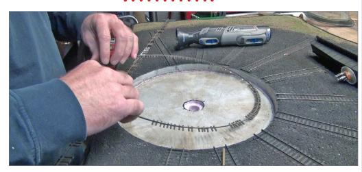
11. A piece of flex track was fed through the band saw to form the rail and tie strips for around the pit walls. I simply bent this around the pit and glued it in place with wood glue.
