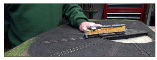
16. Now it was time to test run a locomotive on and off of every track, spinning the bridge around. The AR1 worked well as the locomotive ran smoothly and did not short out when the polarity was changed as the bridge rotated. So, when you see this scene at the Athearn booth you will know a little about how it was built.
