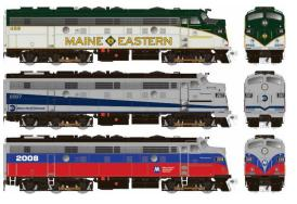
were rebuilt for HEP service in the 1980s. Rapido's version will reflect all of the changes including correct HEP roof details, front and rear HEP receptacles, and optional operating ditch lights. Air horns will be appropriate to road
