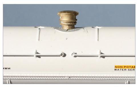
9. With the Athearn bonnet removed, the Precision Scale brass bonnet (part 31005) can be placed. It's scale size.
