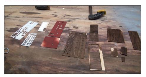
23. This month we build a B.T.S. McCabe Rail Facility Office laser kit. Here you see all the parts painted or stained before assembly. I find this speeds up the building process.
