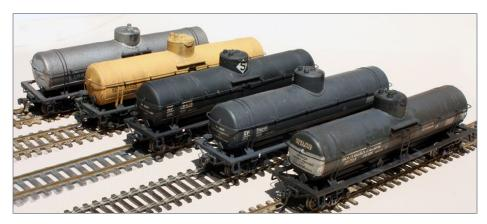
4. Here are five completed SP tank cars, five different paint schemes (the front and back cars are diesel fuel schemes of different eras, the yellow car is a gasoline scheme, the car with the "S" in the diamond on the dome is equipped for liquid sugar service, and the plain black one is in general service). Most are converted from Athearn plastic models.
