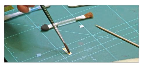
21. I used a good amount of Microscale Micro Set to lift the decal-film from the backing paper.
