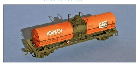
10. This Athearn "chemical" tank car has a replaced valve bonnet of correct size, and a platform around the bonnet made from an Atlas tank car part (see text).
