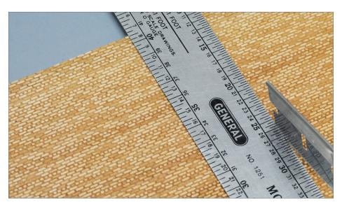
10. Transfer your wall width measurement to the stock sheet. Work in such a way that your straightedge protects the wall face from a wandering blade. In this photo the wall face is on the left, waste is on the right.
