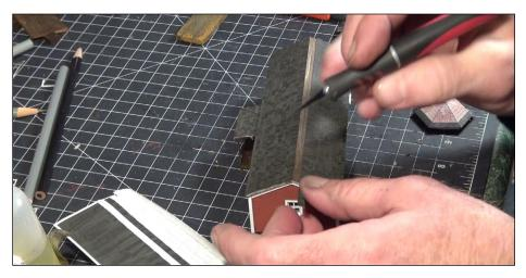
27. I decided to use shingles for the roof rather than the tar paper that came with the kit. I colored the shingles flat black, then used gray colored pencils to add further shading before applying the strips to the roof.
