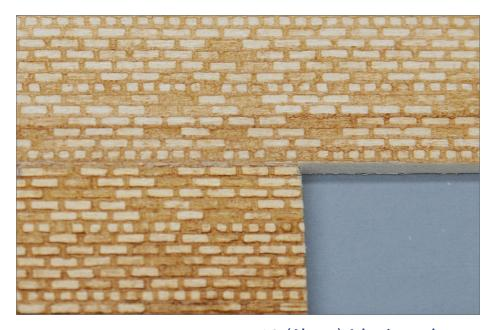
12-15. (Left) Tip 2: The bass-wood substrate allows you to correct inadvertent cuts. On the upper-left is a cut about 1/32" deep that needs to be corrected. First press the wood back into the cut along both edges. I find my fingernail works well for this. To swell the wood, apply a few drops of water along the cut and allow it to soak in. The photo on the bottom-right shows the repair, after painting it will never be seen.
