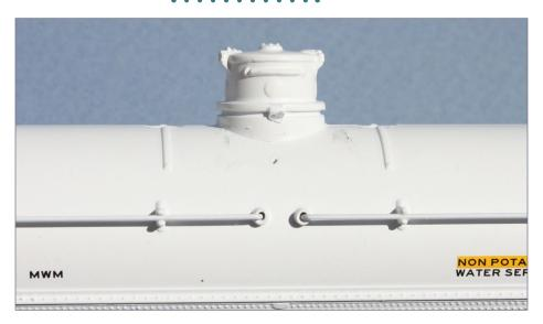
8. The stock Athearn valve bonnet on the "chemical" tank car. It's seriously oversize, as is the platform which goes with it.
