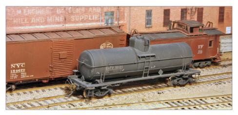
19. The completed 10,000-gallon tank car built by Richard Hendrickson from an Athearn tank car kit. Note that the tank bands at bolsters have been redone as separate bands. I inherited this model from Richard.
