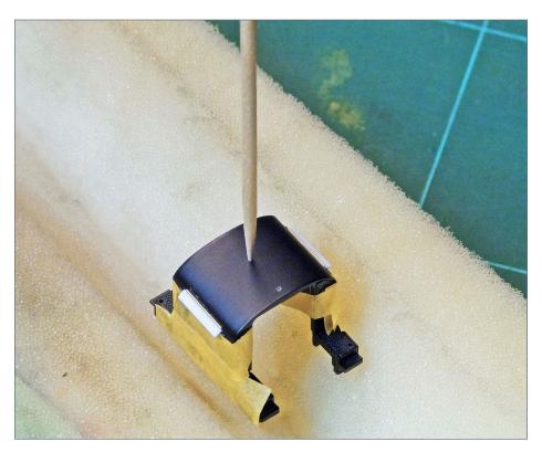
11. A wood skewer was inserted into the antenna hole and cut off flush with the cab roof after the glue dried.
