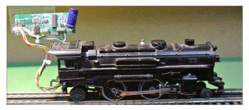
4. Box Car Willie Version 1, BlueRail Trains' first prototype board connected to a Lionel 3-rail locomotive.
