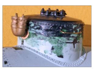
6. The Owl Mountain double safety valve on an elbow mount. The dome height of the Athearn car has been corrected.
