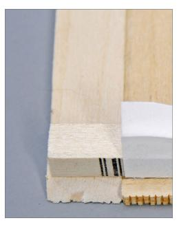
59-60. Cut and fabricate the foundation strip as in method one. Bond the foundation to the bottom of the wall section, aligning the ends of the bevel with the wall edge. After adding the side walls to the face wall, cut and fit the side foundation sections. Bond the side foundation at both the wall and the bevel joints.
