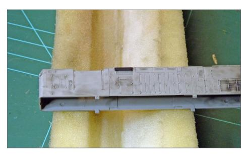
18. The air intake hood glued in place.
