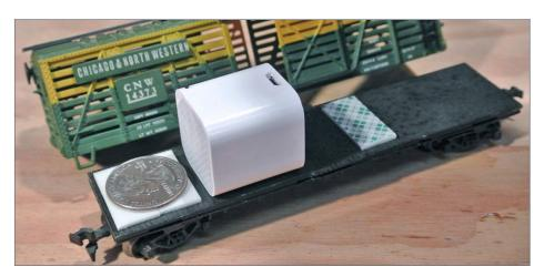
6. Bluetooth (Groove Cube) speaker installed in a stock car to be pulled behind the loco. Sound added for under \$20.
