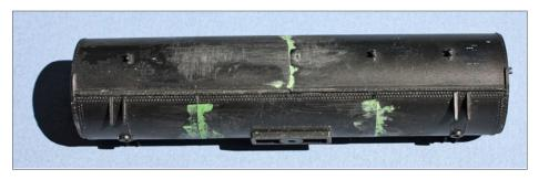
14. An Athearn insulated tank body, shortened to fit the Inter-Mountain frame, and reassembled. Cuts in the top and bottom pieces are differently located (see text). Longitudinal rivets seen here are incorrect and were removed.
