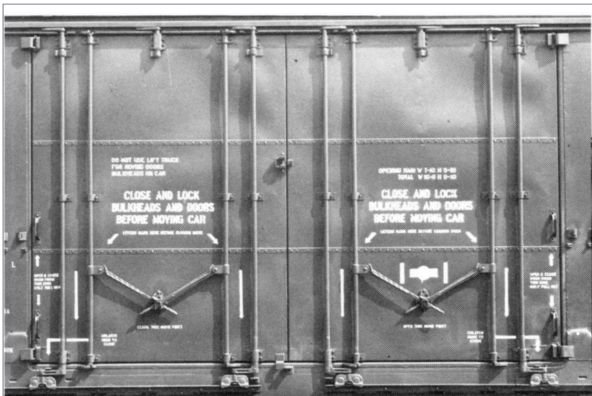
45. Evans double sliding plug doors circa 1980s. Note the paired locking rods at the side of each door.
