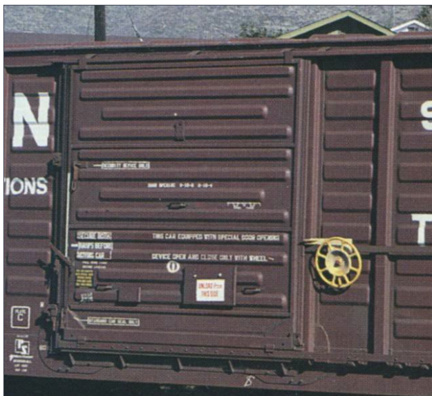
22. Pullman-Standard waffle-design sliding door with corrugations of different lengths.
