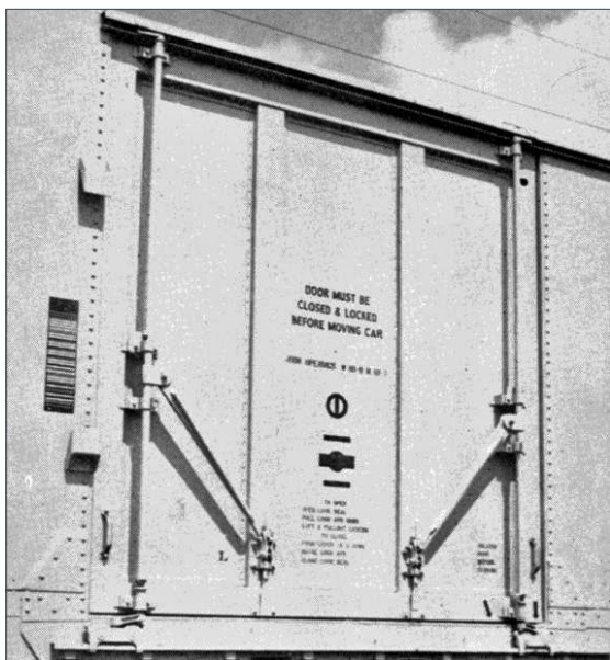
49. Pullman-Standard 10-foot insulated sliding door from the mid-1960s.
