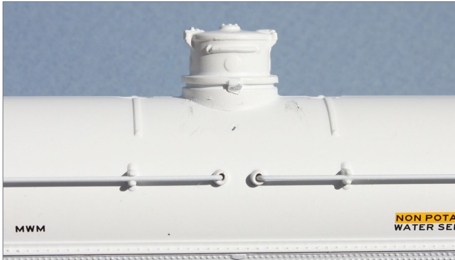
8. The stock Athearn valve bonnet on the “chemical” tank car. It’s seriously oversize, as is the platform which goes with it.
