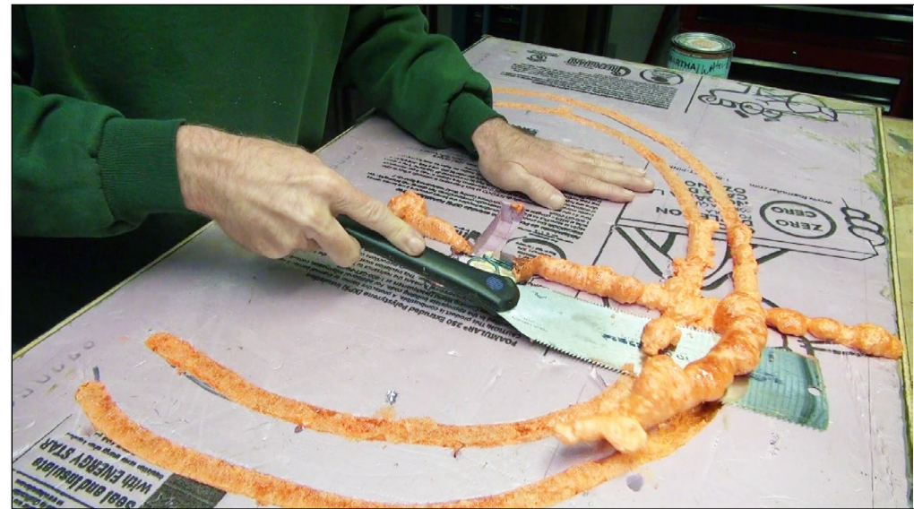
13. After covering the remaining wires with foam, I used a flush cutting saw to trim the expanded foam smooth on the bottom of the display.
