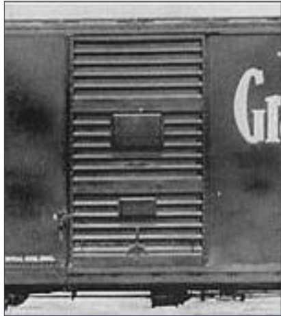
17. A Santa Fe car built in December 1945 by Mount Vernon Car Manufacturing Company has the interim version of the Youngstown door with wide horizontal joint panels and centered door opener at the bottom.
