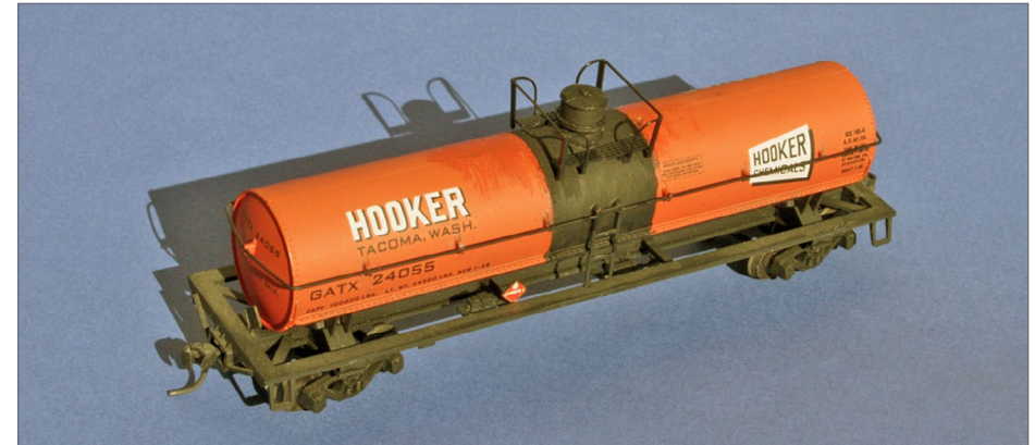
10. This Athearn “chemical” tank car has a replaced valve bonnet of correct size, and a platform around the bonnet made from an Atlas tank car part (see text).
