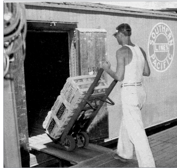
40. To limit the escape of chilled air some reefer doors were just five feet in height.
