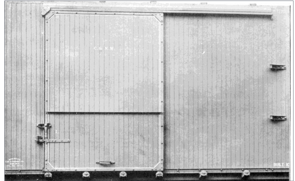
8. National wood door with Camel hardware.
