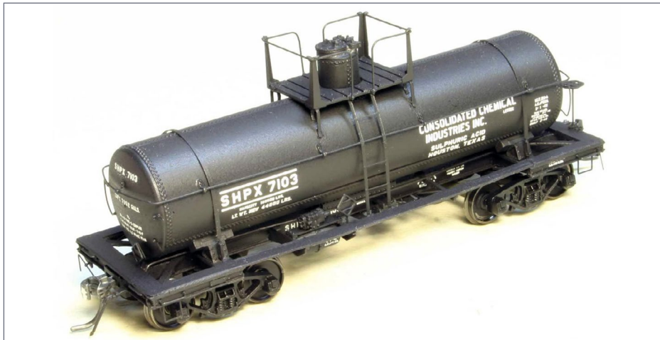
26. A riveted 7000-gallon acid tank car from a resin kit produced by Resin Car Works. As was typical before 1948, the dome platform is wood planks. (Eric Hansmann photo)
