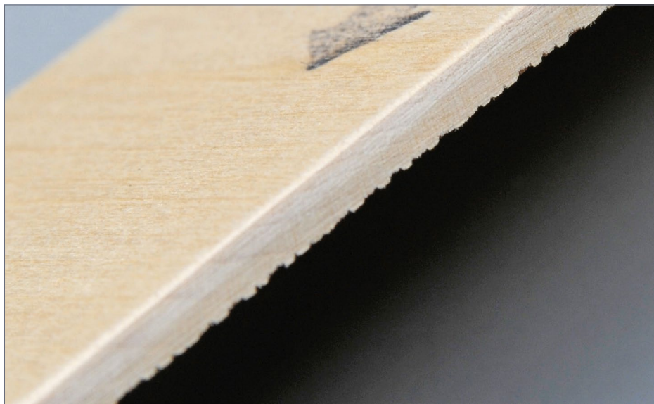
64-65. On the edge of the side that butts against the corner post, do the following: sand a slight bevel that slopes backward with respect to the brick face, then chamfer the back edge. This helps achieve a tight fit against the corner post.
