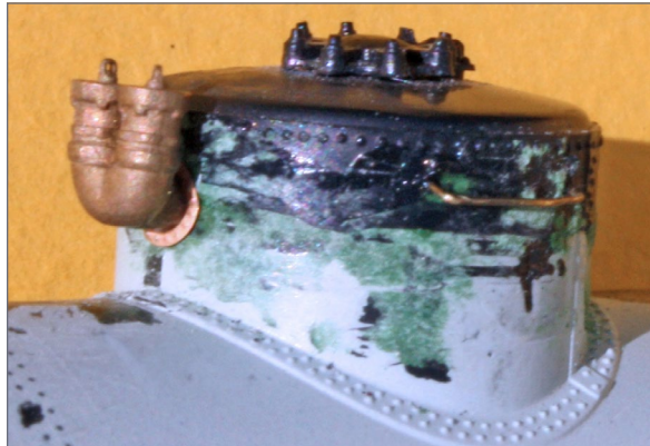
6. The Owl Mountain double safety valve on an elbow mount. The dome height of the Athearn car has been corrected.
