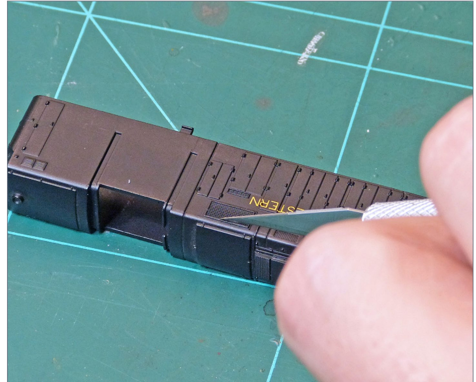
13. Cut on the inside of the upper grille frame.
