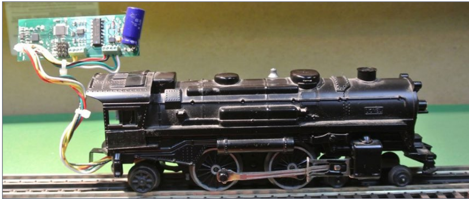
4. Box Car Willie Version 1, BlueRail Trains' first prototype board connected to a Lionel 3-rail locomotive.
