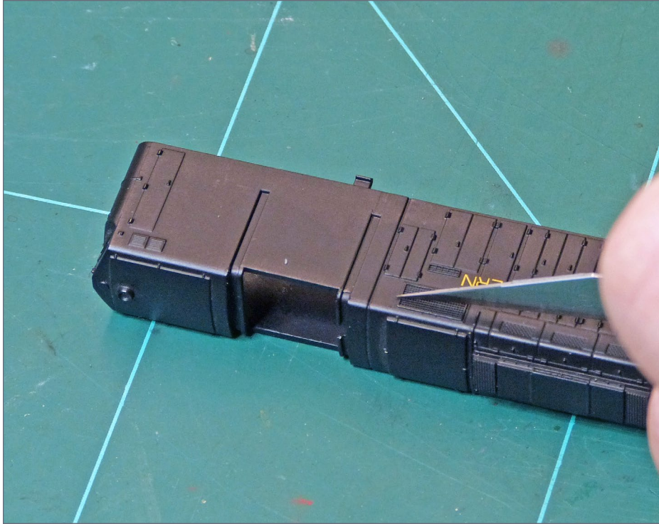
12. Cut through the upper half of the grille frames.
