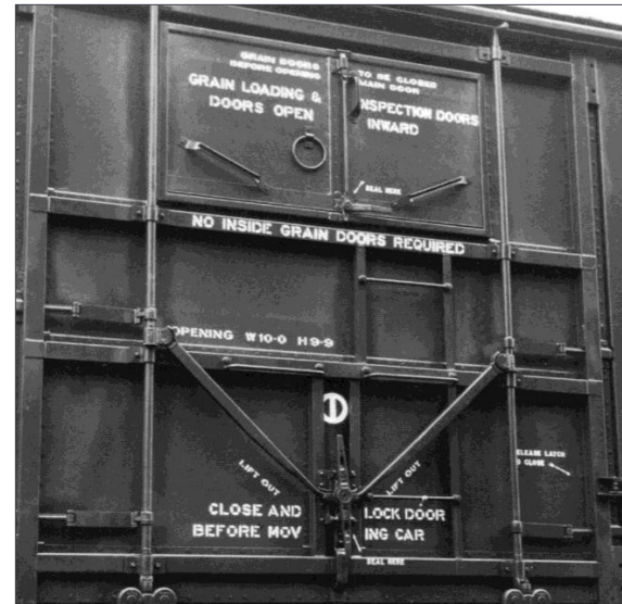
55. Soo Line 10-foot plug door with two small grain doors at the top.
