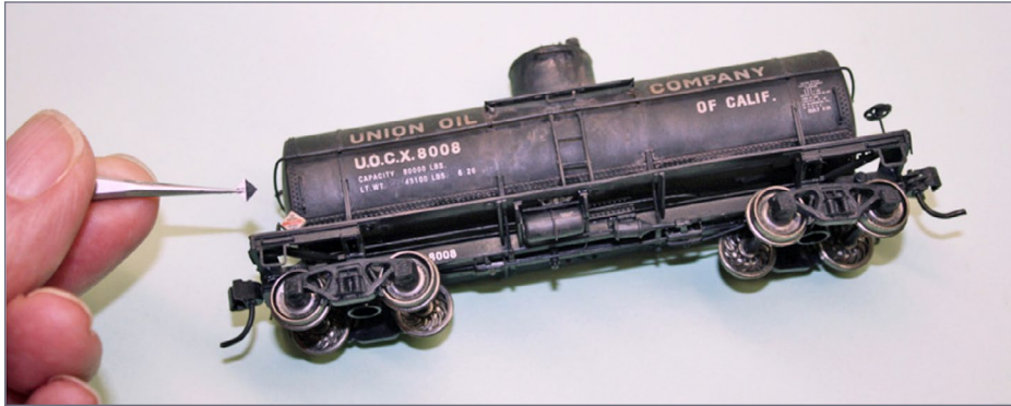
33. In this photo, an “EMPTY” placard is being placed over the placard supplied on this ready-to-run tank car from the Proto2000 line (now sold by Walthers). I usually use canopy glue for this application.
