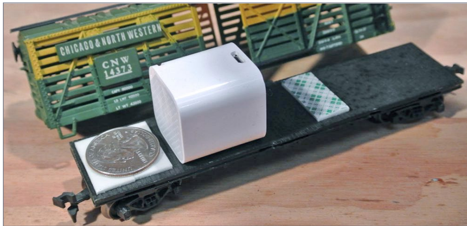
6. Bluetooth (Groove Cube) speaker installed in a stock car to be pulled behind the loco. Sound added for under $20.
