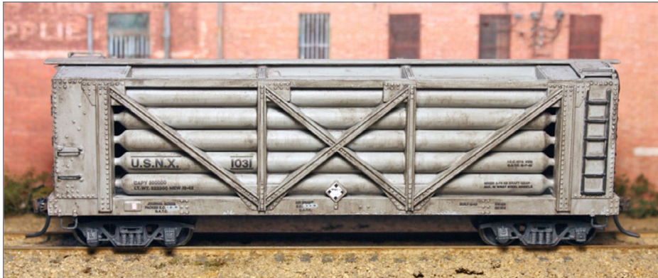
34. This AHM model helium car, with upgraded trucks and details, carries a “COMPRESSED GAS” placard. As explained in Part 1, it’s an ICC-107A tank car.
