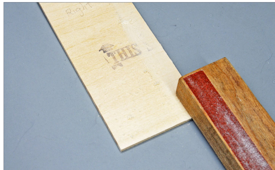
66-67. Test-fit the wall. If it protrudes beyond the corner post, sand the back until it is flush with the post, and make the chamfer if it has been removed.
