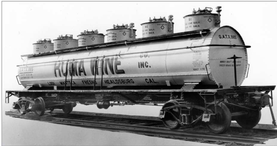
27. This GATX tank car, built in 1926 and leased to the Roma Wine Company, is Class AAR-203 and has 6,600-gallon capacity, divided into six compartments of about 1,100 gallons each. The individual domes all have approved manways, and their frangible-disk safety vents are on an elbow off of each dome. (General American photo, author’s collection)
