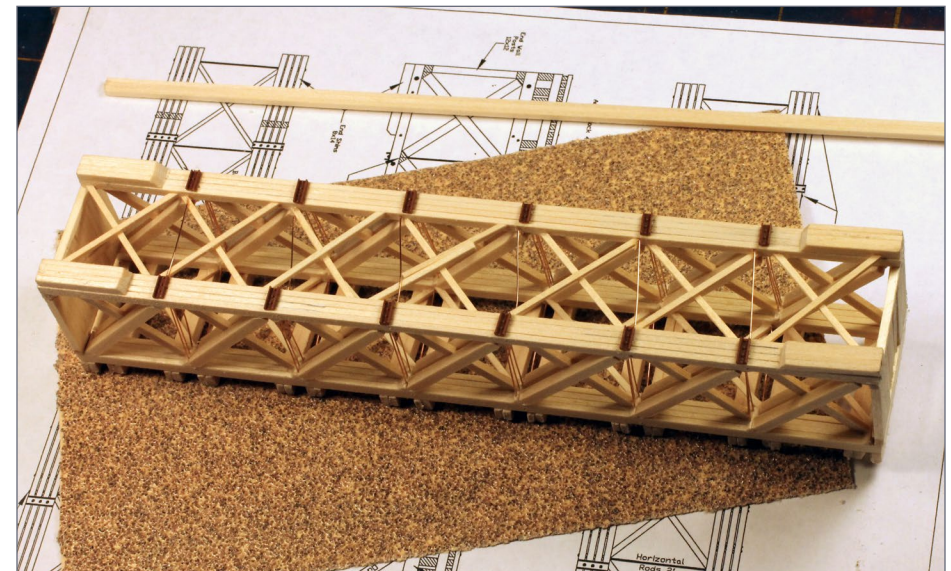
16. Make sure the deck supports are absolutely flat before gluing on the decking.
