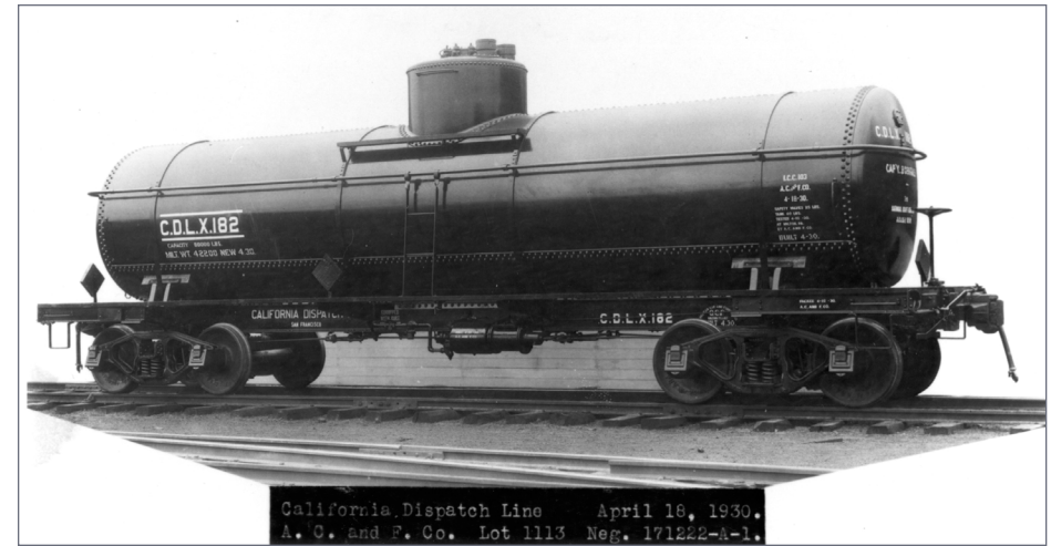
13. Typical tank car construction by 1930. All tank sheets are longitudinal, safety valves are atop dome, tank proportions are relatively long and slender (compare [6]). This nominally 8,000-gallon car, owned by leasing company California Dispatch Line, has 40-ton trucks and shows characteristic American Car & Foundry construction, having end sills as well as stub side sills from bolster to end sill. The photo date is April 19, 1930. (AC&F photo, Richard Hendrickson collection)
