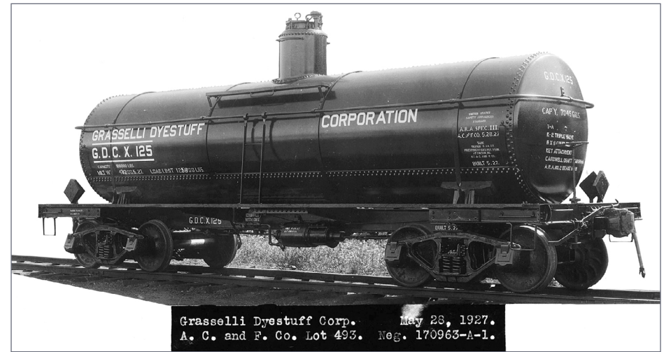
25. A typical acid tank car, Class ICC-103A, with its distinctive dome shape and appliances. The car was built in 1927 and has 50-ton trucks and 7045 gallons capacity, typical for cars carrying dense acids. (AC&F photo, courtesy Edward S. Kaminski)
