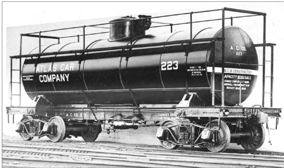
4. This 8,000-gallon Class II tank car was built in January, 1911 by American Car & Foundry. It was designated “Type 7” for the year of its underframe design, 1907. Longitudinal tank seams are double riveted. Note the white band on the car end, lettered “MCB CONSTRUCTION,” as was required until about 1918. (ACF photo, Edward S. Kaminski collection)
