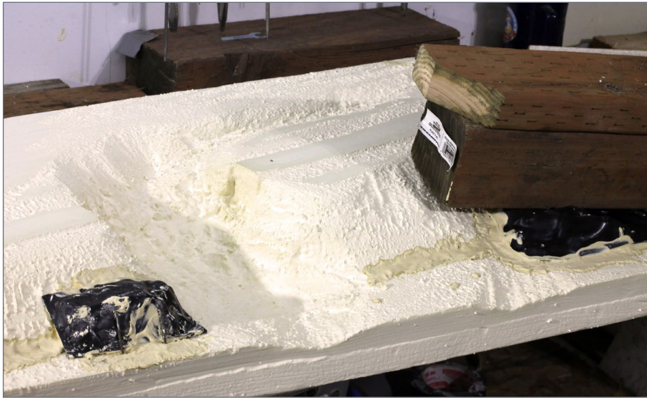
27. Rock molds are flexible, and some times the mold needs a little "help" to stay in place during set-up time.
