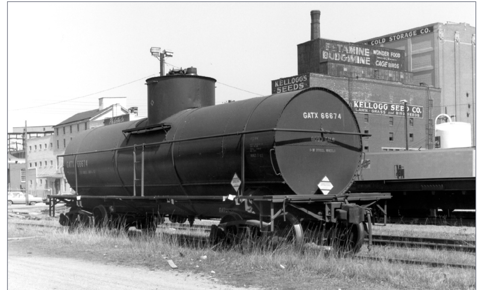
26. This tank car, General American-built GATX 66674, is an 8,093-gallon car of ICC-104 classification. Its insulation jacket is thicker than the normal two inches, likely intended for a specific cargo and specified by the buyer for a particular lessee. This undated photograph was taken at Milwaukee. (Richard Hendrickson collection)
