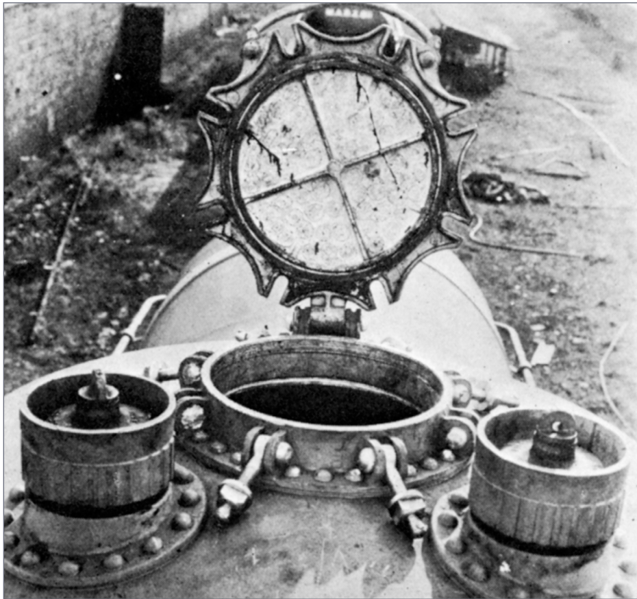
10. A clear photograph of an “approved” bolted manway in the open position, with restraining bolts pivoted away from their working position. (American Car & Foundry)
