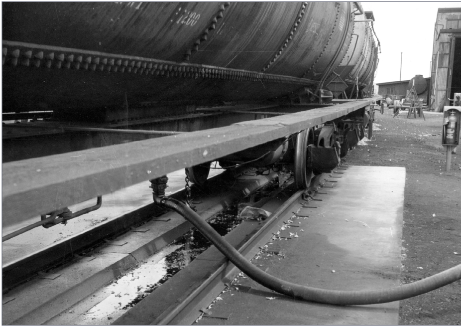
12. Gravity unloading of a tank car, by attaching a hose to the bottom outlet. Photo at the diesel fuel spot in Alturas, California. (SP photo, Shasta Division Archives)
