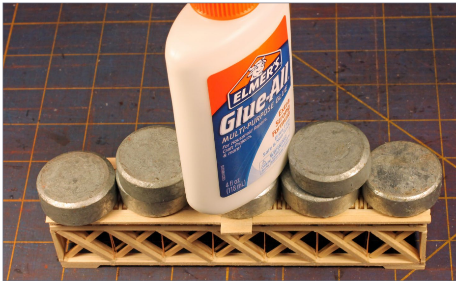
17. Gluing on the decking.
