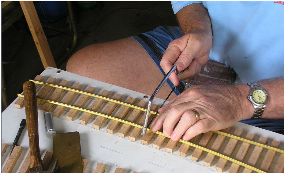
7. I use a small hacksaw to cut the rails where the rails move to switch routes.
