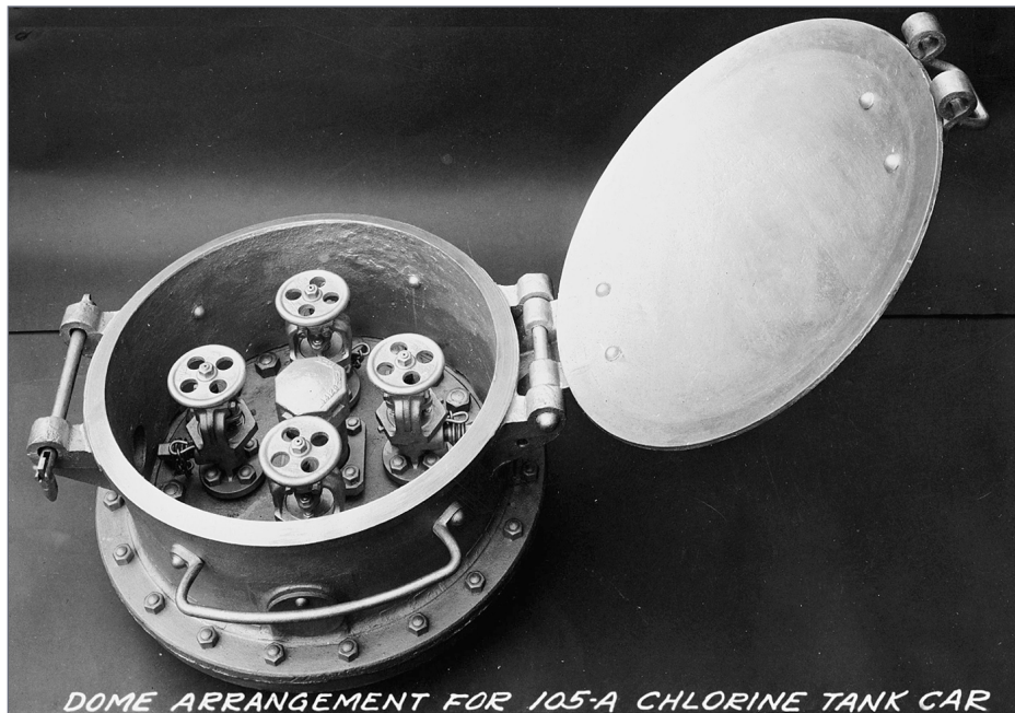
18. Interior of a valve bonnet for a chlorine car. Valve handles control openings for sampling, temperature measurement, and venting, as well as loading and unloading. The shell of the bonnet has openings for hose connections, for example nearest the camera, just below the grab iron. (AC&F photo, courtesy Edward S. Kaminski)
