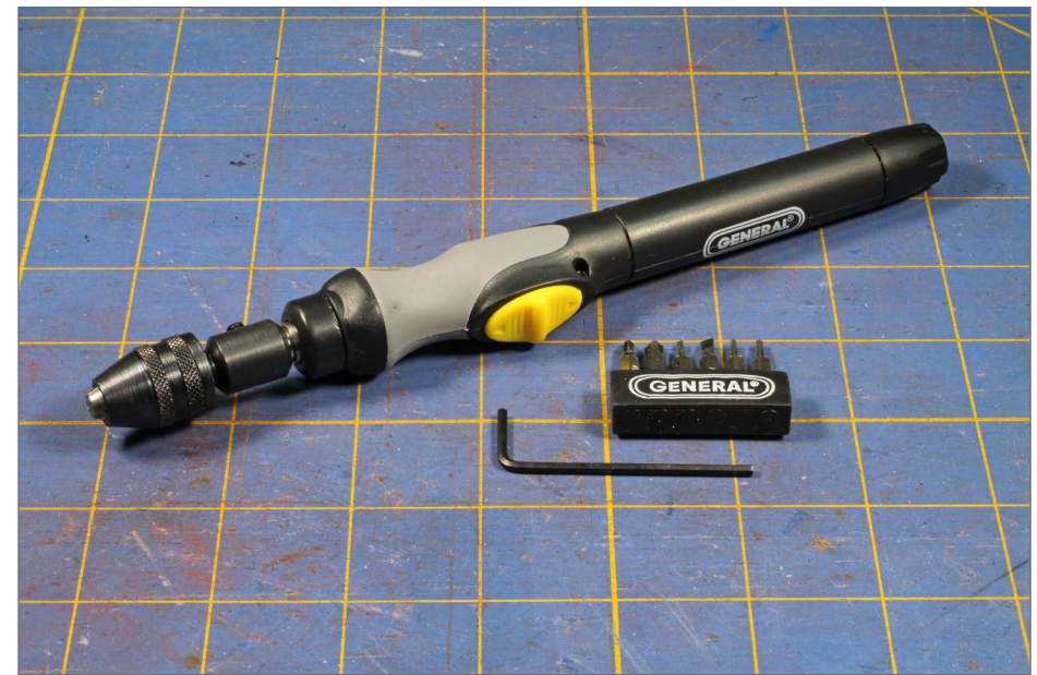
8. A great new tool. A power pin-drill driver.
