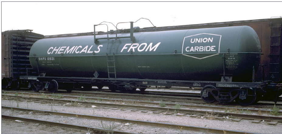
24. The late 1950s changes in ICC requirements led to major changes in tank car appearance. This large car, SHPX 12831, is ICC Class 111A100-W-1, has 20,000 gallons nominal capacity. Photo at Los Angeles in 1960. (Morris Abowitz)
