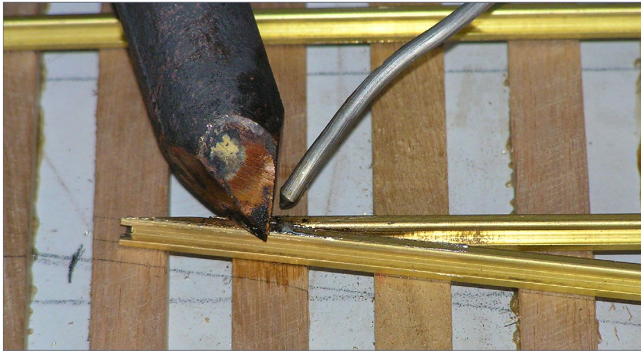
13. With large rail, a large soldering iron is required to generate enough heat for proper soldering.
