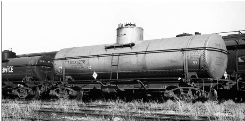
14. This 8,053-gallon Tidewater Associated Oil Co. tank car, built by General American in 1925, has 40-ton trucks and was photographed in lighting that clearly shows its absence of side or end sills, typical General American features. The walkways are supported entirely from the center sill. Photo at Kansas City, 1954. (George Sisk photo, Charles Winters collection)
