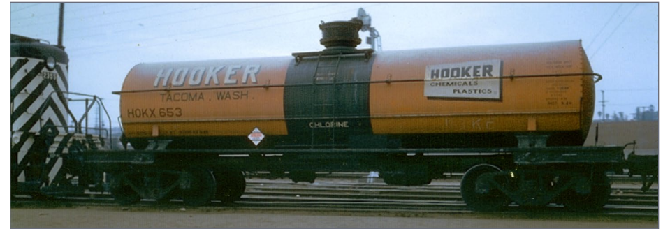
19. A typical high-pressure tank car, in this case a Hooker Electrochemical car carrying chlorine. It is a 5,907-gallon car, a common size for chlorine, and has 40-ton trucks. Photographed on the Santa Fe in the Los Angeles area in 1959. (Morris Abowitz)
