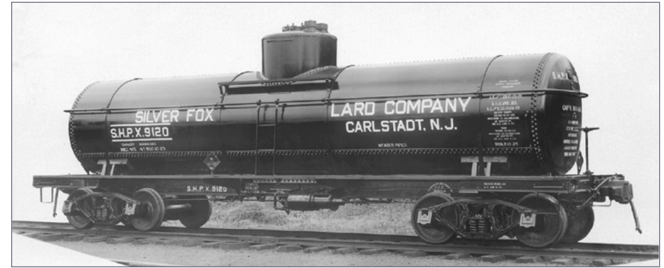
28. Tank cars were used for a variety of foodstuffs, as this 8,111-gallon car shows. It is an ICC-103 built in 1929. (AC&F photo, courtesy Edward S. Kaminski)
