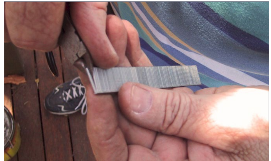
3. The spikes are cut from a strip of nails that are used in my nail gun.
