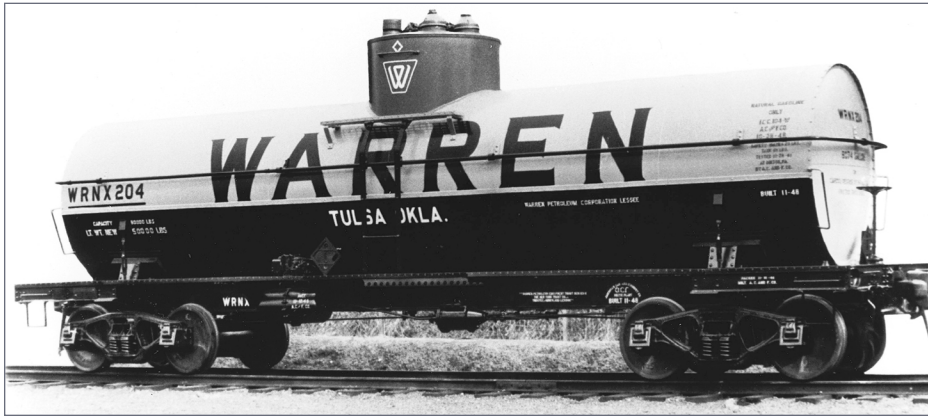
15. This Warren Petroleum car is a good example of an ICC-104 class of car. It's an 8,074-gallon insulated car built in 1948 by AC&F with 40-ton trucks. Atop the dome is visible one of the safety valves, but also visible are some stubby conical appliances. These are the covers for air vents (during unloading) and siphon valves for sampling. A close-up view of these parts is presented in [16]. (ACF photo, courtesy Edward S. Kaminski)
