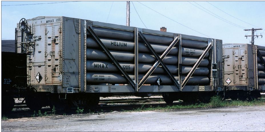
23. This is a helium tank car, ICC-107A, photographed about 1975. Loading and unloading is accomplished with fittings inside the end doors of the car. Note the empty placards on the car. (Richard Hendrickson collection)
