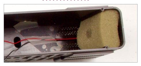
4. Close-up view of the interior, showing "magic" tape holding the bulb wires down. Also, notice the holes that the owner had drilled through the front fan grille.
