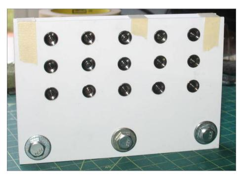
14. Wheels inserted into wheel mask ready to paint, front view.
