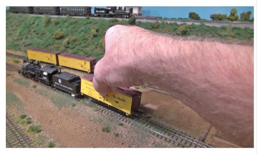
31. To test that the Current Keeper is working, simply pick up the car from the layout. If everything is right, you will hear the sound effects for as long as 10 to 15 seconds without track power. ☑
