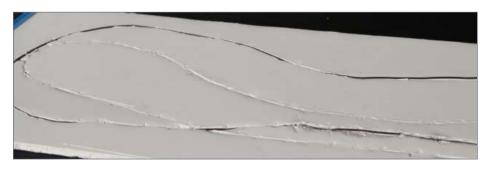
65. Embedded wire in the foamcore base guides the crane on its route.
