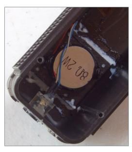
5. The 28 mm square highbass speaker is mounted inside the shell under the drilled-out fan grille. It is sealed to the shell with clear caulk. The caulk is currently white, as it was applied just before this photo was taken. Note the white caulk plugging the mounting holes in each corner of the speaker. This keeps the sound confined to the side of the cone that generates it.
