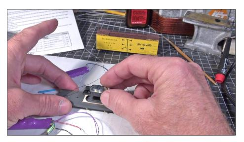
23. I mount the speaker gasket to the floor of the car, then press-fit the speaker on top of that.
