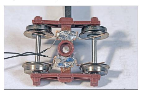
19. I cut the coupler box spring just beyond the punch hole and solder very fine stranded wire to these wipers.
