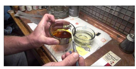
4. I use a pair of tweezers to remove the metal from the acid and place it in a bowl of water to stop the process. If you let it boil for more than 30 seconds the metal will dissolve completely.
