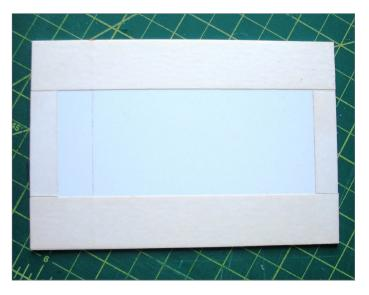
3. Doublestick tape applied to one sheet, to be attached to the other.
