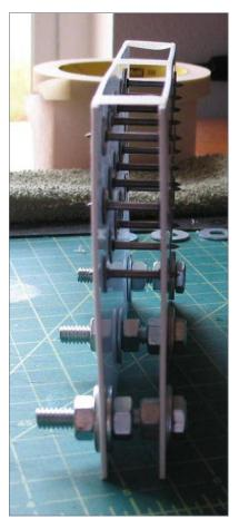
15. Wheels inserted into wheel mask ready to paint, side view.
