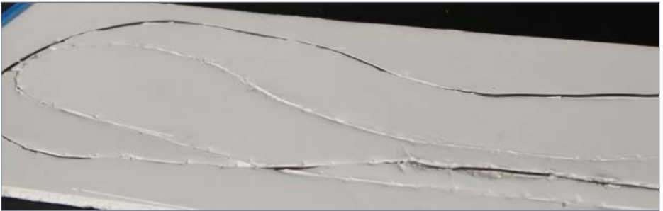
65. Embedded wire in the foamcore base guides the crane on its route.
