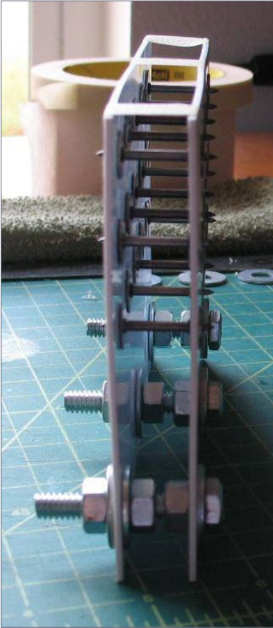
15. Wheels inserted into wheel mask ready to paint, side view.
