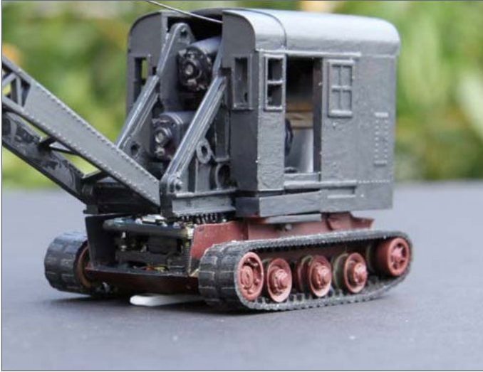
62. The shoe that guides the crane can be seen between the tracks.
