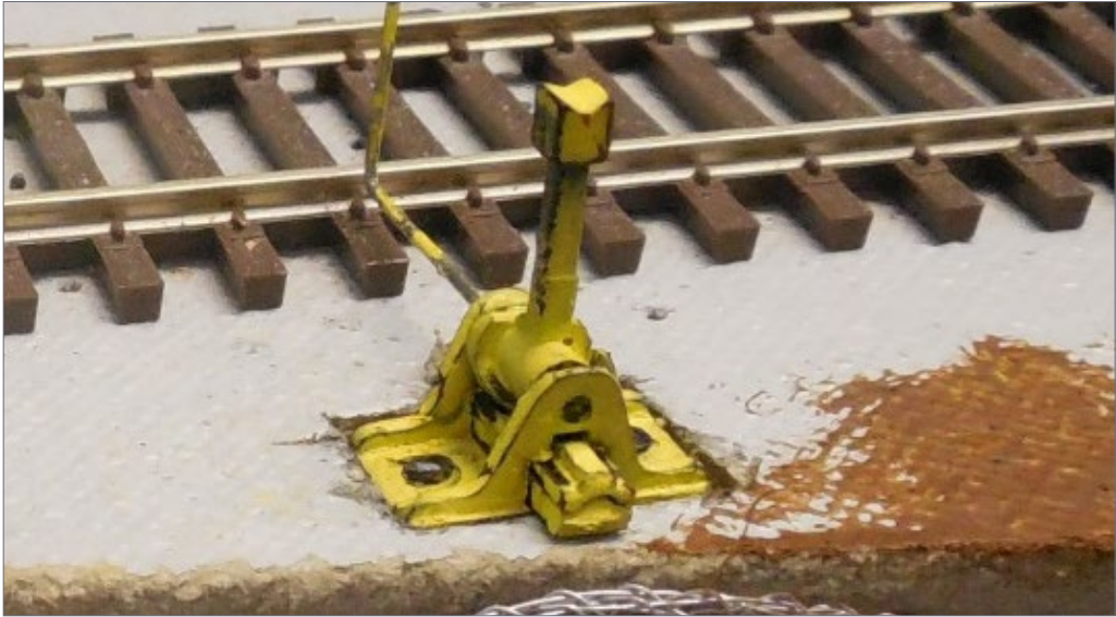
4-5. Here is a car holder built using a Caboose Hobbies ground throw. Ray Schofield photo
