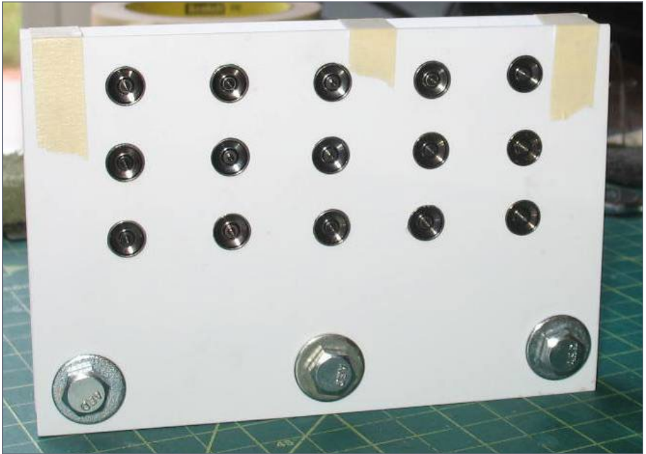
14. Wheels inserted into wheel mask ready to paint, front view.
