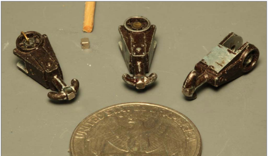
95. Magnet-equipped hooks. The quarter gives you a good idea how small the magnets are.
