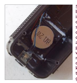
5. The 28 mm square highbass speaker is mounted inside the shell under the drilled-out fan grille. It is sealed to the shell with clear caulk. The caulk is currently white, as it was applied just before this photo was taken. Note the white caulk plugging the mounting holes in each corner of the speaker. This keeps the sound confined to the side of the cone that generates it. LokSound L -Premium Quality Low Cost DCC and Sound in O Scale!
