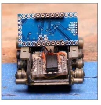
75. Hand-built driver placement in the chassis.
