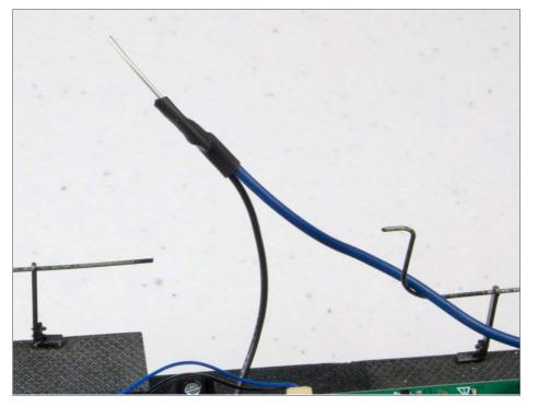
8. Truck wires twisted and soldered to a 20 AWG solid wire for connection to the decoder screw terminals.
