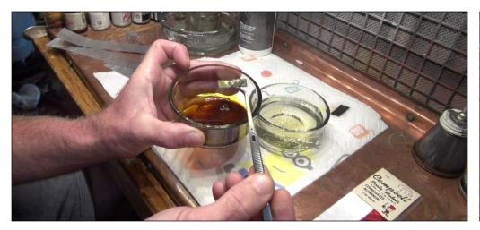
4. I use a pair of tweezers to remove the metal from the acid and place it in a bowl of water to stop the process. If you let it boil for more than 30 seconds the metal will dissolve completely.
