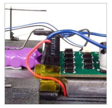
9. Side view of decoder with track wires attached. Kapton (yellow) tape was used to keep the wire in the groove while the shell was installed.
