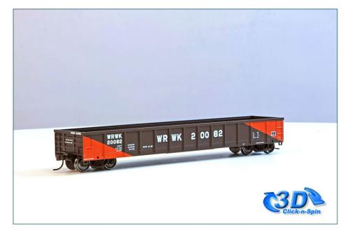
3. In 1975, the Southern Iron and Equipment Co. started building a 52'6", 100-ton gondola. Evans took over SIECO and continued building the cars through December 1981. A total of 1,730 cars were built with three minor body variations. This model represents the second version, and the most common.
