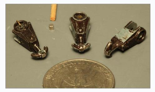
95. Magnet-equipped hooks. The quarter gives you a good idea how small the magnets are.
