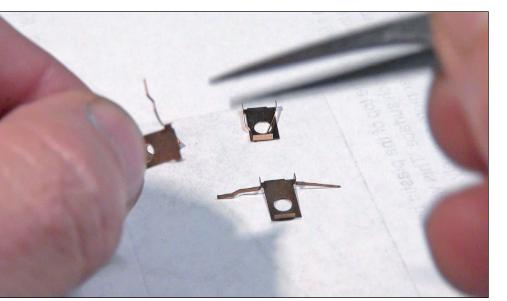
18. I bent Kadee HO scale #5 coupler box springs as shown in this photo to form the power wipers.
