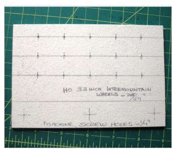
4. Top of one side of sheet set, covered with masking tape, measured and marked for drilling. Note small dimples at center points.
