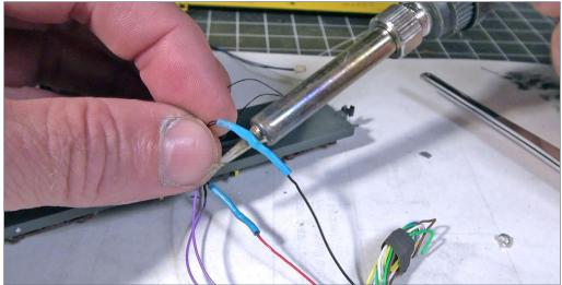
24. I use shrink tubing to insulate the solder joints as I solder the decoder to the truck power feed wires, red wire to the right side of the car and black wire to the left power pick-up wire of the car, as per the decoder instructions.
