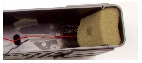
4. Close-up view of the interior, showing "magic" tape holding the bulb wires down. Also, notice the holes that the owner had drilled through the front fan grille.
