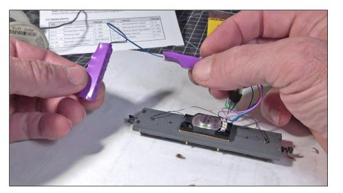
26. Installing the Current Keeper is easy. Simply plug it into the jack on the end of the Soundtraxx sound car decoder. This will ensure constant sound even when the power to the car is interrupted on dirty track.
