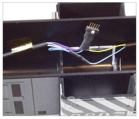
11. 5-pin connector in the shell to connect LEDs and speaker to the main frame. Note white dot to denote polarity.
