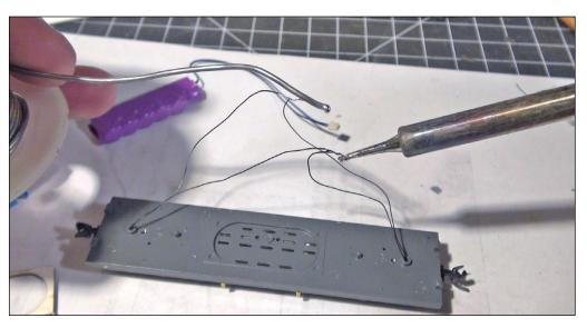
21. After reattaching the trucks to the car bottom, pull the wires through the holes next to the coupler boxes in the floor of the car. Solder the right side power feeds together, and then solder the left side power feeds together.
