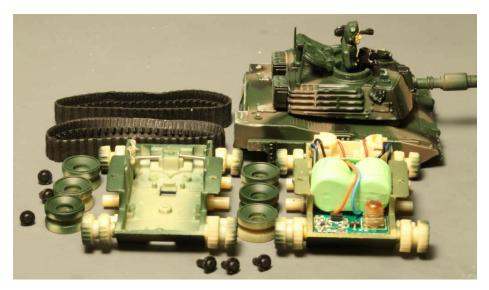
55. The RC mini-tank used for the chassis of the crane.
