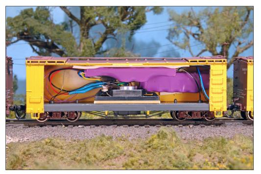
29. A cutaway view of the car shows the decoder and Current Keeper installed along with the speaker. It all fits perfectly. I programmed the car to run a few times with flange squeal and rail joint sounds in combination. Then I programmed it to run with just joint bar click-clack sounds so you can hear the difference in the video.
