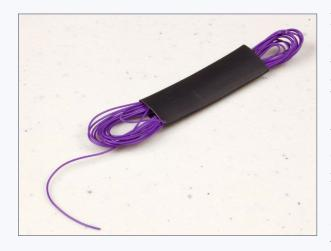
I wrap the wire around my hand and tuck the resulting hank into a piece of shrink tubing. I find that the 3/8 inch diameter gives a nice fit. I keep them in a storage tray and have all the colors together when I need them.
