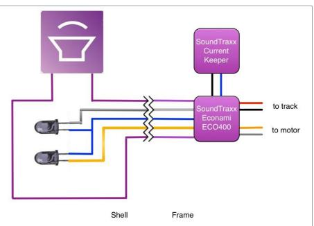
12. Wiring diagram. Connect the female side to the decoder. Note that reversing the connection only exchanges the front and rear lights. No ill effects will happen if you rotate the connector this way. However, offsetting the connection by one position may damage the decoder, speaker or LEDs.
