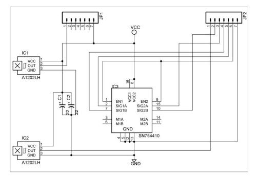
69. Dual motor driver schematic.
