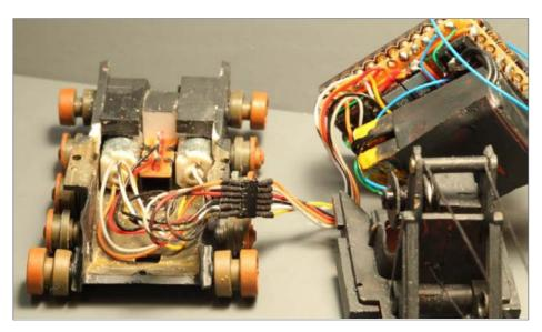
88. Crane 3 motors and wiring harness.
