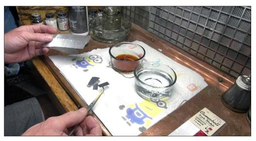
2. The corrugated metal is cut into 3x8 scale foot sections for HO. One bowl is filled with the etchant, and the other with water. The water stops the process.
