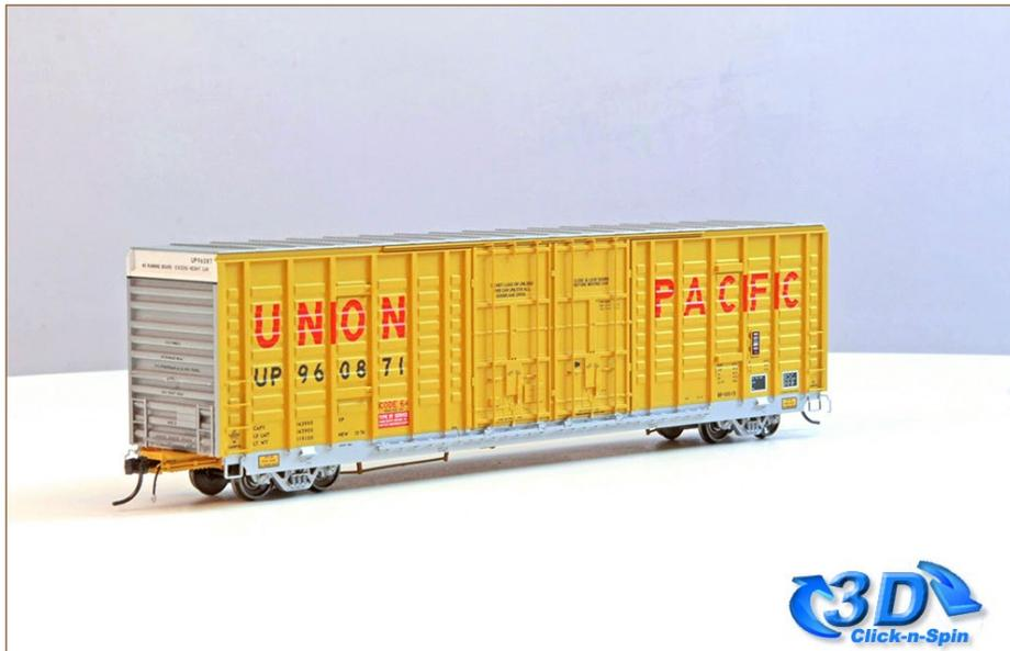
4. In 1974 Pullman-Standard's Bessemer, Alabama plant began to manufacture the 7315 cubic capacity "waffle" boxcar for the Norfolk and Western Railway. Production continued with additional deliveries to the Santa Fe, Milwaukee Road, Union Pacific and Detroit, Toledo and Ironton. The P-S Waffle Box Car continues to serve Class 1 railroads to the present.
