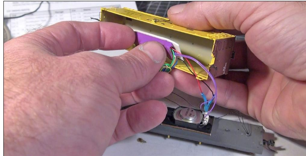
27. I use two-sided foam sticky tape to mount the decoder to the roof of the reefer, and more tape to mount the Current Keeper to the side of the car.
