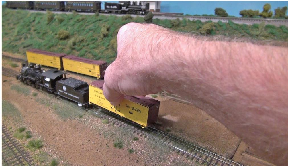
31. To test that the Current Keeper is working, simply pick up the car from the layout. If everything is right, you will hear the sound effects for as long as 10 to 15 seconds without track power.
