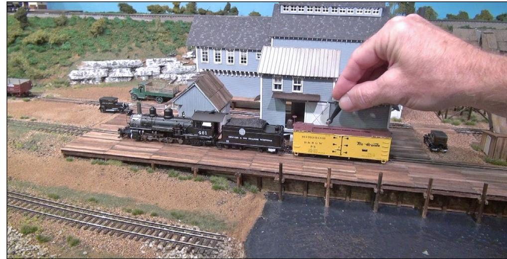
30. To test the sound car on the layout, I waved a magnet along the roof of the car so the decoder could find the locomotive's address and automatically consist with it as I pushed F8 on the throttle four times. Now the car is consisted with the locomotive and will run and give sound effects that match the speed of the locomotive. Don't forget to click on Reader Comments and rate this month's edition of What's Neat.
