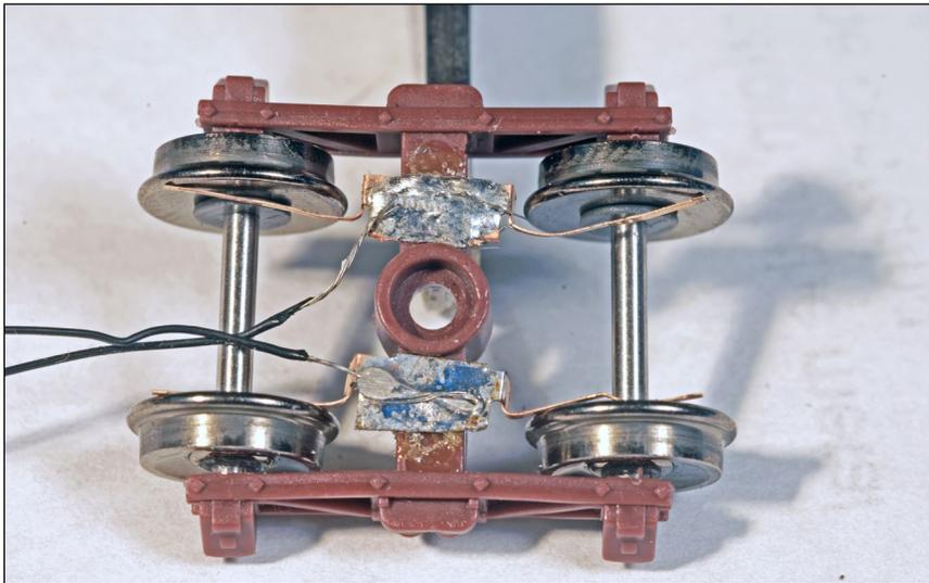
19. I cut the coupler box spring just beyond the punch hole and solder very fine stranded wire to these wipers.
