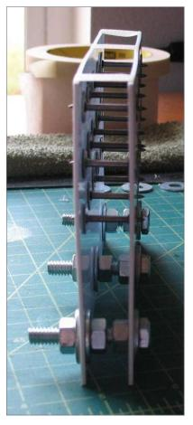
15. Wheels inserted into wheel mask ready to paint, side view.
