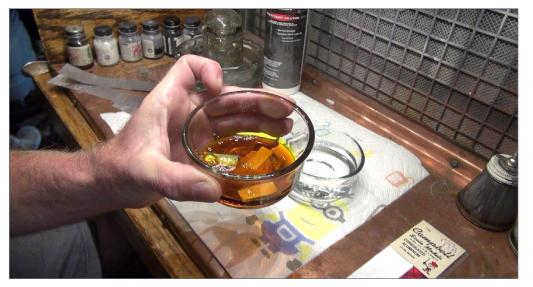
3. I place the metal in the bowl of etchant, and in 20 seconds the boiling process begins. Here you see the violent bubbles as the acid eats away at the metal's surface.
