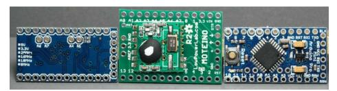
83. Arduino Pro Mini (left) vs. Moteino (right), bottom view.
