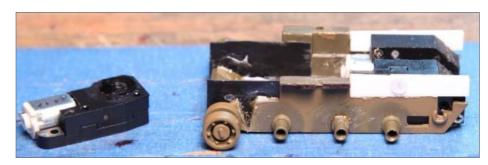
57. Chassis side-wall preparation for the motor drives.
