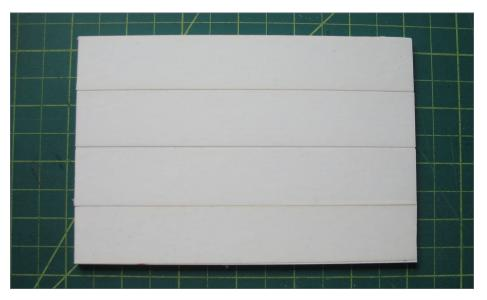
5. Double-stick tape applied to full face of plastic sheet set, to be attached to scrap wood base.
