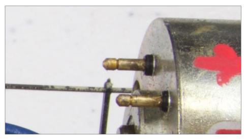
7. Motor polarity mark: A red + mark next to the motor terminals that connect to the right rail when wired for DC.
