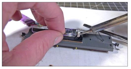
25. I solder the decoder speaker wires to the solder pads on the speaker.
