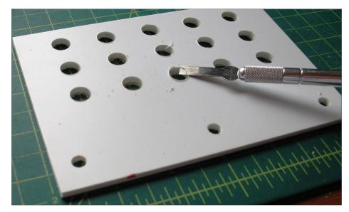
9. Removing drill ridges from holes with chisel-tip hobby blade.
