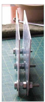
12. (Left) Assembled wheel mask side view.
