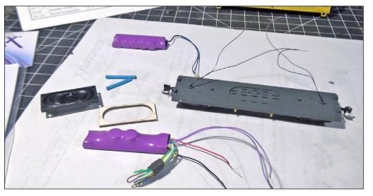
22. Here are all of the parts: the SoundCar decoder, the Current Keeper, the 35x16 mm speaker, and the foam self-adhesive speaker gasket. All of this is available from Soundtraxx.
