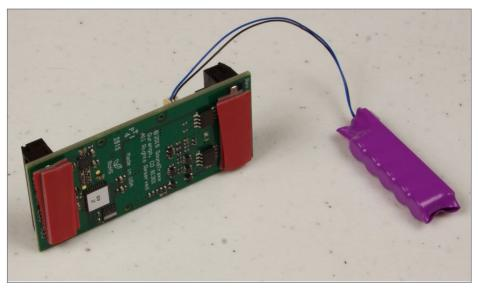
6. A double layer of gray tape (with red backing) on the decoder screw terminals raises decoder up from baseplate so chips don't contact the metal plate. The tape also insulates the screw terminals.
