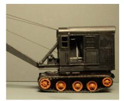
60. (Above) Level the cab bottom by filling in the raised portion under the door and window.
