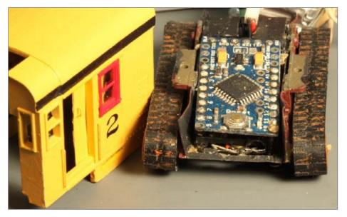
79. Pro Mini and sensor mounting in the chassis.
