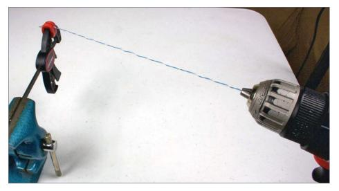
10. LED light wires being twisted with drill. LED is in a clamp attached to a vise on the left.
