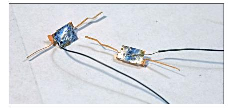
20. I glue the new wipers to the top of the truck bolsters with contact cement. This glue is flexible and will stick to the Delrin material the trucks are made from. Notice that I have good wiper contact with all four wheels.
