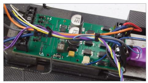
13. Close-up of decoder area. Note routing of CurrentKeeper wires (small blue and black) to allow clearance for shell. Lacing cord is used to bundle the other wires together.
