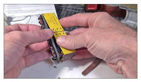
28. I reassemble the car, taking care to not pinch any of the wires. It is now ready for a test on the layout.
