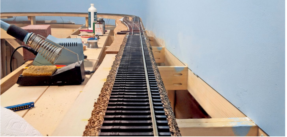
49. A piece of rail was set on the CV ties and used as a sight line to make sure that the CV ties are straight.
