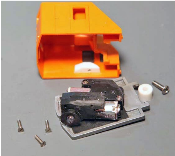
27. The motor drives have been mounted on cab floor.
