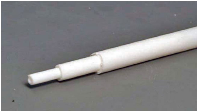
18. Forming the drive hub from tube styrene.
