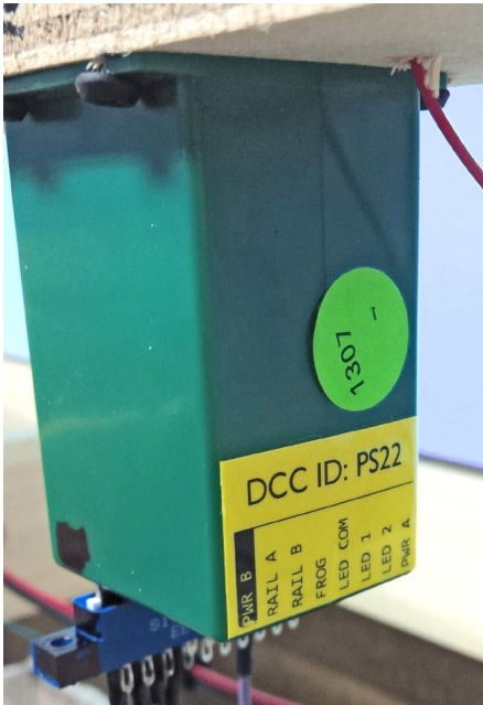
52, 53. I apply a label on the Tortoise marking the purpose of each connection and then duplicate the labeling at the terminal strip.
