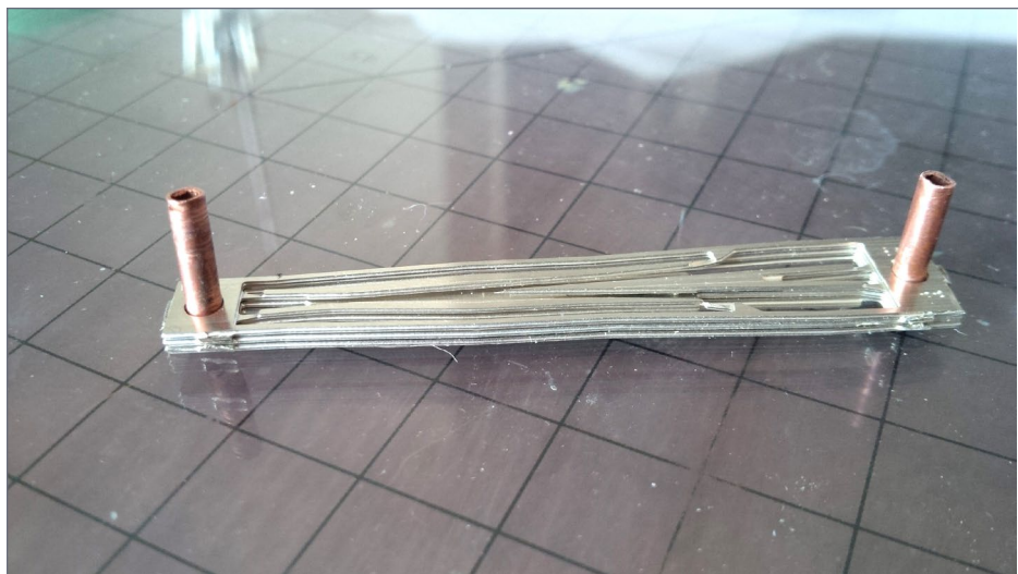
16. Frog parts assembled and ready to be soldered.
