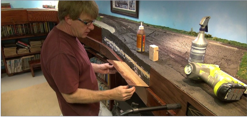
35. Quarter-inch oak plywood cut to shape and stained with red oak stain covers the sides. It is finished with three coats of polyurethane varnish, sanded between coats with 1500 grit wet sandpaper.
