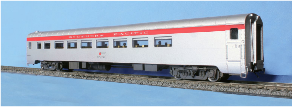
2. Former Daylight parlor car as rebuilt to chair car 2243 with flat stainless sides, vestibule end.
