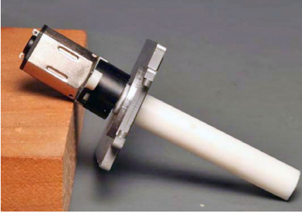
41. Hub cut and screwed to the motor shaft.
