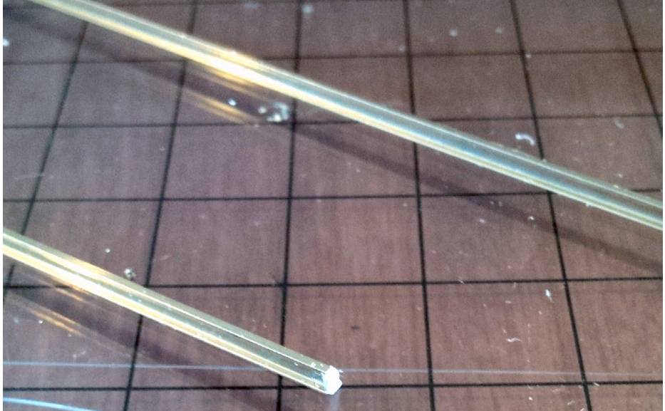
30. Styrene is added to the ends of the rails to electrically isolate the frog from the closure rails.
