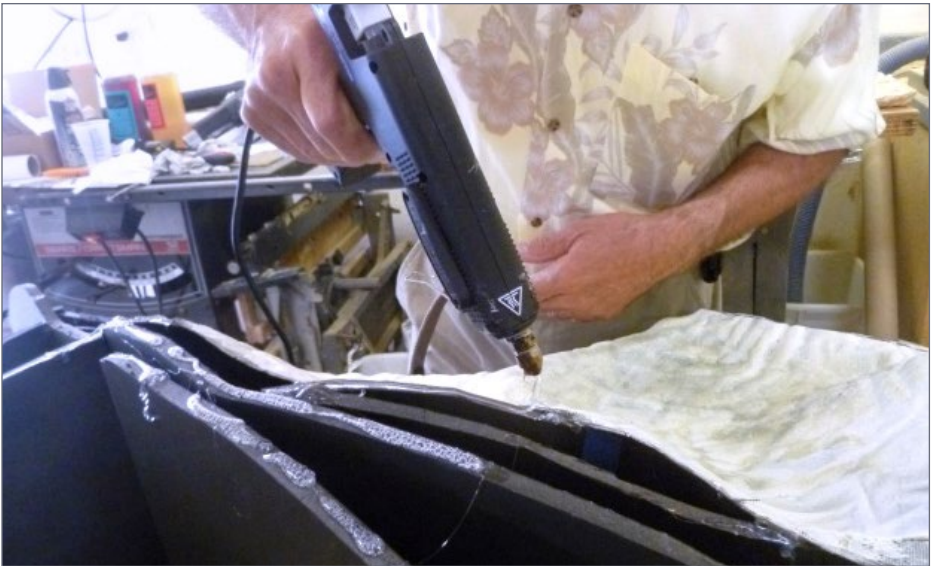
20. Attaching the panel with hot glue.
