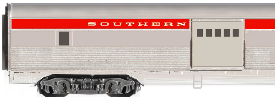
ATHEARN DROP EQUALIZER TRUCKS SHOWN - CAR HAD TRIPLE BOLSTER TRUCKS
