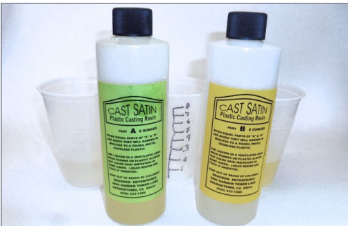
28. Cast Satin polyurethane casting resin.
