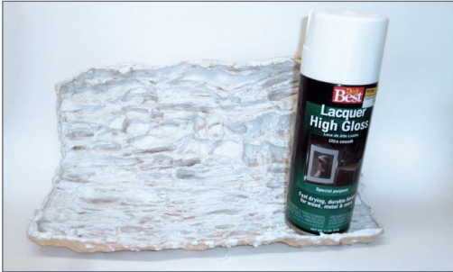
27. Spray the mold with white lacquer paint.
