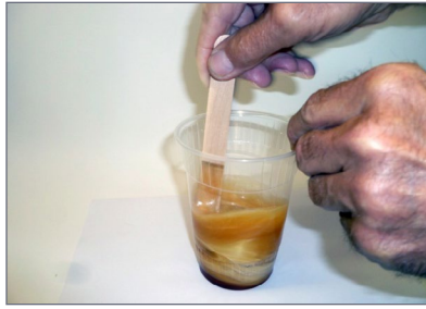
15. Stir the resin quickly.
