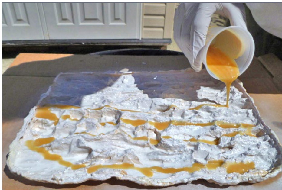
32. Drizzle the mixed foam over the mold.
