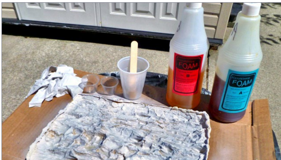
31. Foam part A and part B ready for mixing.
