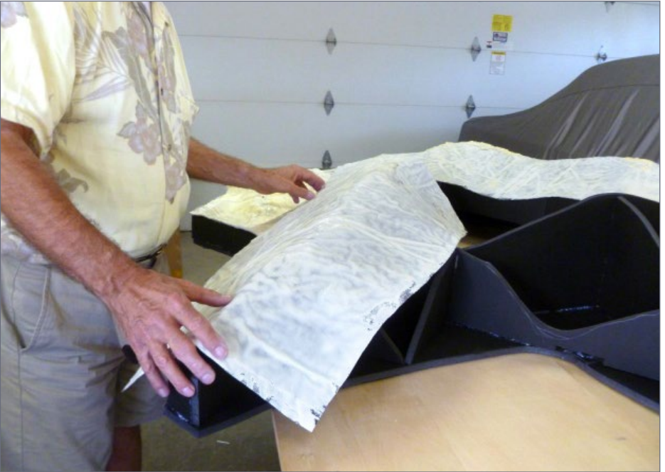
19. Molding the panel to shape.
