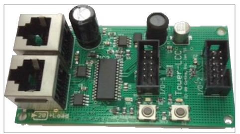
3. A basic LCC node: bus connections on the left and external hardware connection on the right.
