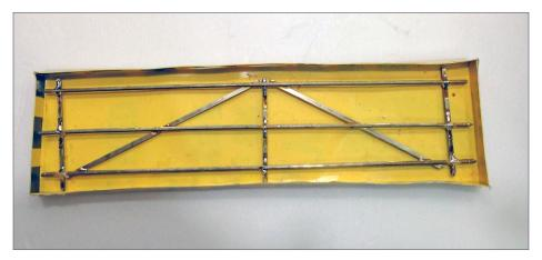
2. The mold and scrap rail for the dam. I filled the mold with plaster and once it set, I carved the stonework with an X-Acto knife. I soldered the scrap rail together and didn't worry about being too neat. In fact, the whole mold need not be all that pretty, either.
