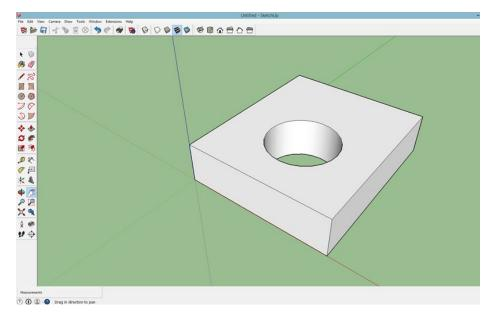
5. If you go completely to the bottom of the cube, the hole will extend completely through the cube.
