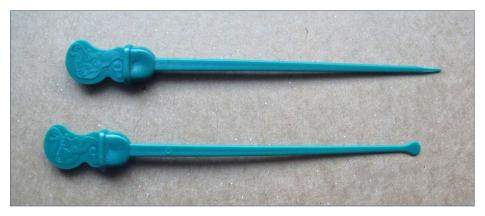
3. Shape a point on a Starbucks "stopper" to make a useful uncoupling tool.
