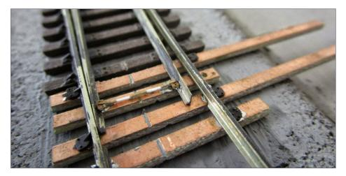
13. Greg used Micro Engineering (ME) turnouts, but replaced the throw bars and headblock ties with copper-clad PC board ties. Greg will add ME and Proto:87 Stores turnout detail to the turnouts to enhance their realism.
