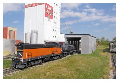
27. Tank cars could bring fuel oil for the boiler house, molasses, fish oil, or linseed oil. The feed-mix oils were stored in tanks next to the blending tower. The mill would want to know how much product had been removed from a tank car after each workday, so the switch crew would weigh each tank car on the scale in the unloading shed and replace it. It usually took three days to empty a car of molasses. This means a car could be weighed and re-spotted twice before being pulled as an empty.
