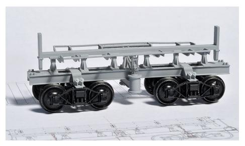
23. Here is the printed frame resting on the trucks. The bed itself will be built up with stripwood and the end levers and other small parts reproduced using photo-etching. As of this writing, the model is still under construction. But getting this far would have been impossible without using 3D printing.
