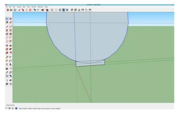
17. When one shape overlaps another shape, as in this case, it results in three parts which are 1, the large part of the circle; 2, the remaining small part
