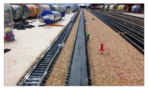
2. R. Seiler uses a 5/8" steel bar on straight HO flex track to help straighten it and to weight it down. *R. Seiler photo*
