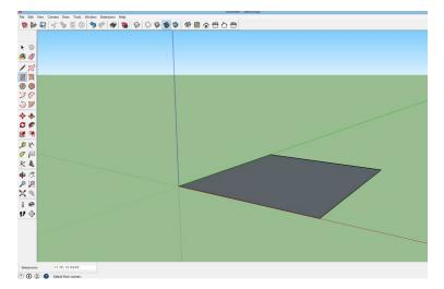
1. Here is the basic sequence used to draw something in 3D using SketchUp. Begin by using the Rectangle Tool (high-lighted in the Tool Bar along the left side of the screen) to draw a rectangle.
