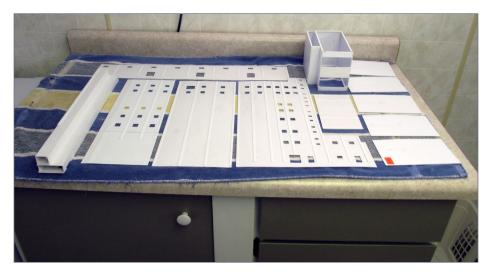
7. Here's the building "kit." All windows and doors have been cut out. I've glued strips of styrene on the walls to represent the extra support columns. I also cut out interior warehouse bulkheads. Finally, I've collected the other structure pieces needed for the complete assembly.
