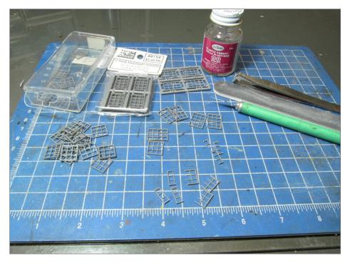
3. Here's the window assembly line. I'm using the knife to remove one vertical sash from the Tichy rectangular masonry windows. Trimming is done with sprue nippers or nail file, and then I'm gluing the pieces back together. I kept the finished windows in a fishing lure box.
