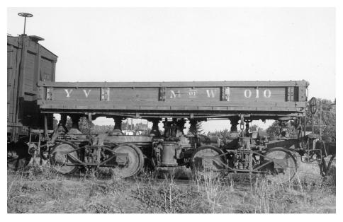
21. At first glance, scratchbuilding a model of this side dump car appears to be nearly impossible given the complex design of the frame, the pedestals which allow the bed to be tipped to either side, the U-shaped supports for the bed, and the complex rods and levers which actually tip the bed. However, with experience and by working methodically, it is completely possible.
