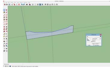
this view. Right click the remainder of the circle to open an Entity Info box. In the entry for Segments, backspace over the number and type in a larger number such as 24 in this case for just the remainder of the circle. If you are drawing a full circle, increase the number of segments to 96.
