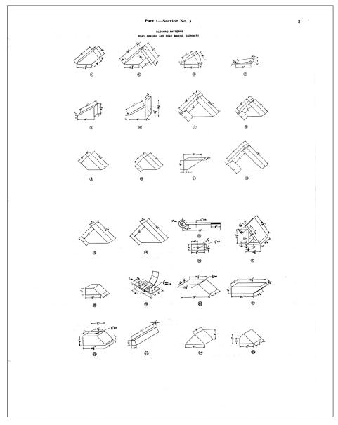
25. Blocks 2 & 3 are needed for the road grader. Note how it shows the dimensions.
