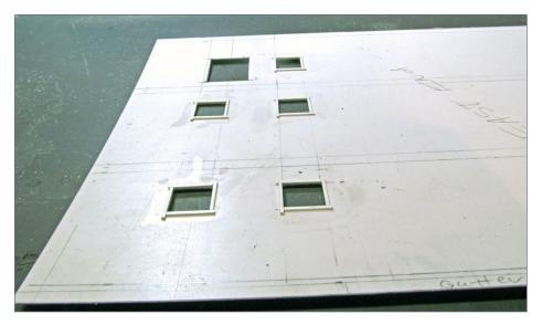
8. One of the drawbacks to using .015" styrene for the walls is the lack of gluing surface for the masonry-style windows. I overcame this by building a crude frame on the inside of the wall. I placed a window in the opening (it protruded through the .015" styrene) and pushed the .030" square styrene strips against it and applied glue to the wall. I immediately removed the window, since I was only using it to position the strips for gluing – I was not ready to install the windows.
