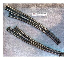
Atlas has announced plans to produce code 83 nickel silver curved turnouts. The HO turnouts have die-cast points and an isolated, die-cast frog with a power contact to optionally energize the frog and prevent momentary loss of contact when a powered model is passing through
