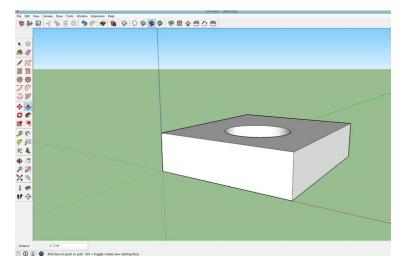
4. Click on the circle with the Push-Pull Tool and then move the mouse downward to create a hole.
