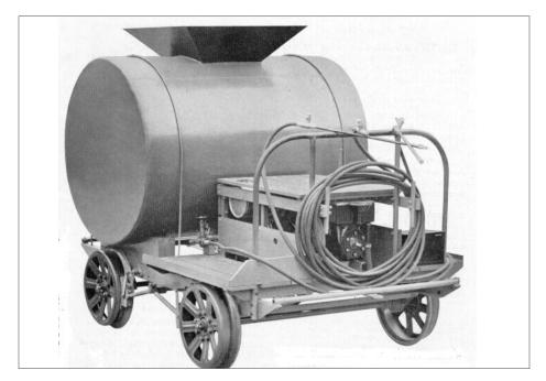
10. A Fairmont Motor Company photo of a T27 extinguisher car. The wood tank supports can be seen between the water tank and the frame.
