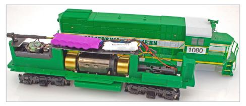
6. ECO-100 diesel and CurrentKeeper installed in a Walthers HO scale GP15-1, using a 16 x 35 mm 8-ohm speaker in a baffle arrangement.
