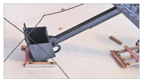
21. The bracing around the shovel. The threads are used to string the cables used to operate the shovel.
