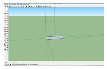
will result in another guideline 48 inches above the centerline of the rectangle. That is where we need to draw the circle representing the 48-inch-diameter water tank.
