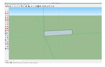
rectangle. "Hesitate" near the top center of the rectangle and the tool will snap to the vertical center of the rectangle, creating the first centerline.
