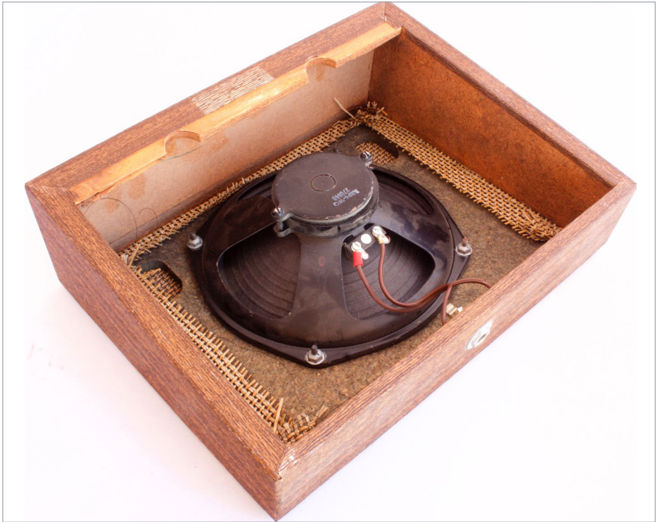
2. Eight-inch 8-ohm speaker in a public address wall baffle that I used for the initial sound quality test.
