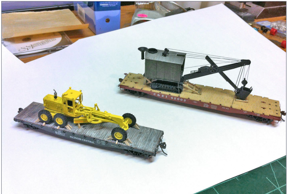
35. This is the final product. Here you see the wires that go from the crane to the flat car. There are two at the front and two on the rear.
