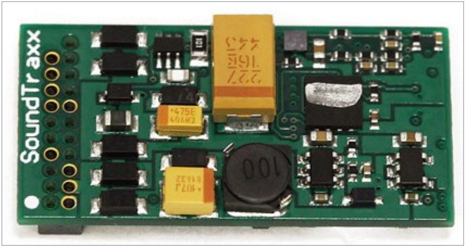
7. ECO-21, 21-pin connector version of the 1-amp model with a 2-watt amplifier.
