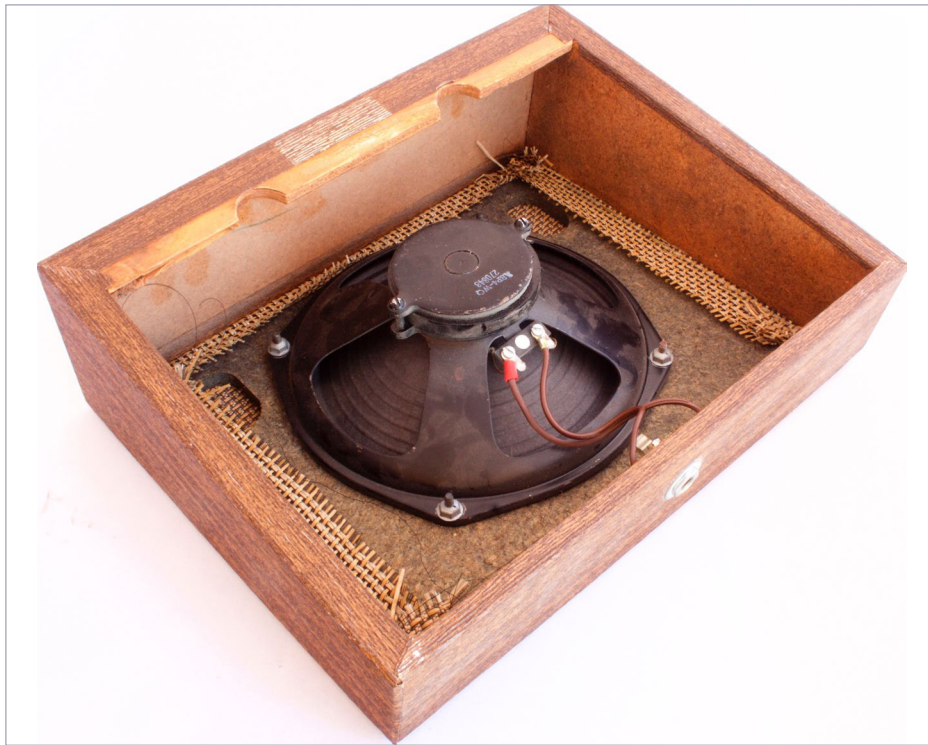
2. Eight-inch 8-ohm speaker in a public address wall baffle that I used for the initial sound quality test.
