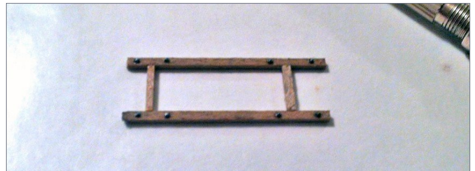
15. This shows the nut/bolt castings in place. I spray-painted them black, and then dry-brushed the heads with silver hobby paint. Then I cut them off and glued them in place with CA.
