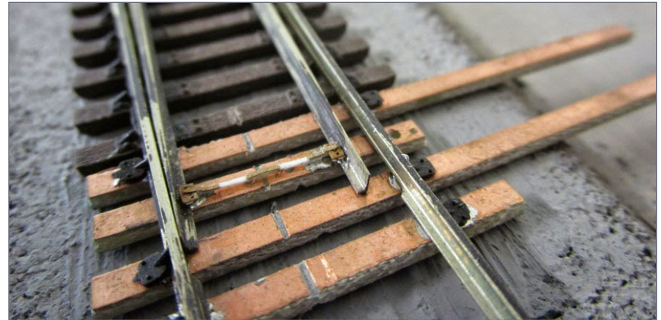
13. Greg used Micro Engineering (ME) turnouts, but replaced the throw bars and headblock ties with copper-clad PC board ties. Greg will add ME and Proto:87 Stores turnout detail to the turnouts to enhance their realism.
