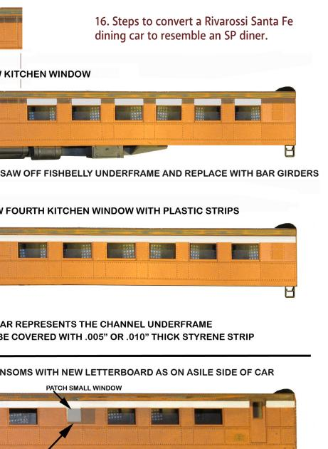
SHER HAD A FOURTH AISLE WINDOW THAT COULD BE CUT IN THE RIVAROSSI SIDE. SHORT BLANK PANEL BETWEEN THE DINING AND AISLE WINDOWS, AND I LEFT THE THREE ORIGINAL AISLE WINDOWS.
