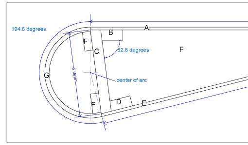
5. A cross-sectional top view of the end of the backdrop shows how the backdrop layers (A) and (E) split and are screwed to the bullnose mounting plate cleats (B) and (D).
