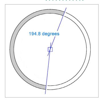
8. Once again I turned to 3rd PlanIt. I drew a pair of concentric circles the same diameter as the inside and the outside of the tube. Then I drew two lines from the circles' center, spaced the needed angle apart. I printed it full size and we stood the tube on end on
