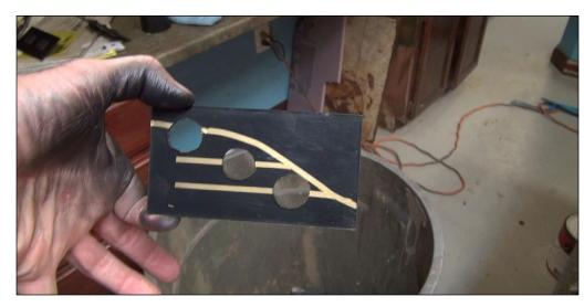
5. When you turn it over, you can see the new track arrangement on the panel in gold. It's ready to reinstall on the foam module.
