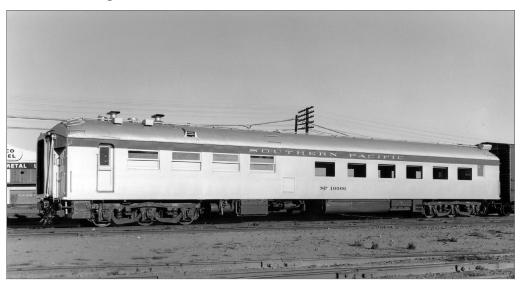
11. Class 77-D-4 dining car, nearly identical to 77-D-3. Kitchen side of car 10006 shown in the mid-1960s in imitation stainless steel with red letterboard paint. *Courtesy Bob's Photos*
