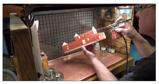
9. Using an airbrush, I painted the main walls with Floquil Tuscan paint. My formula is 25 psi of air pressure, and the paint thinned 50 percent.
