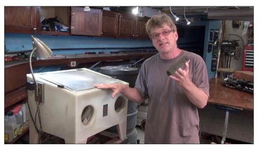
20. For this month's video tool tips, we discuss and demonstrate sandblasting brass models. Most models come with a lacquer clearcoat. When painted over, this can really cover up a lot of details. Sandblasting the model to remove the clear lacquer makes for a smooth finish with all the detail popping out at you.
