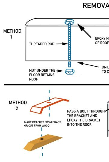
2. Mounting a removable roof for almost any model passenger car.
