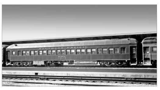
26. SP's arch roof coaches can be simulated by adding a round roof to the Walthers model and removing the fish belly underframe. *Courtesy Bob's photos*
