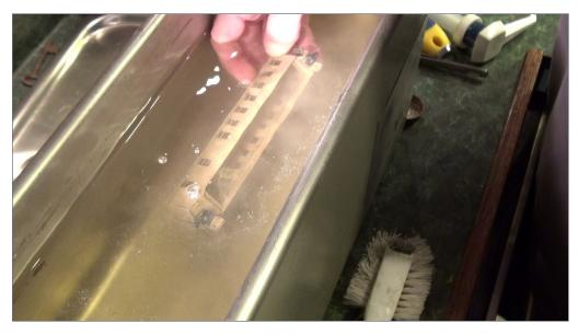
22. After blasting the model, I wash it in water from the sink and brush off the loose sand from the model. No matter how much you wash and brush the model, when you place it in the ultrasonic cleaner a dust cloud forms in the bath as all the dust from every crevice starts to float free. Now you have a clean model ready for paint. You can watch the entire process in this month's video in real time.
