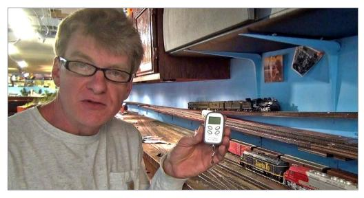
24. I can measure the pulling drag of any given train with this Micro-Mark digital weight scale that allows very fine measurements.
