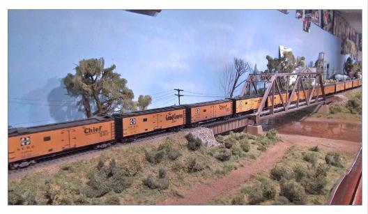
26. My HO scale 62-car reefer train had a pulling drag of over 4.5 ounces. By replacing the trucks with Kato after-market trucks I was able to reduce the drag of the consist of cars to 2.2 ounces – more than half. Trains now run better with fewer coupler separation problems.
