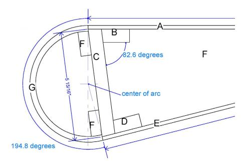
10. Now we needed to figure out how to attach the bullnose to its mounting plate. After much discussion we added two small cleats (F) on each side of the mounting plate's face, indenting them from the backdrop's surface a tad more than the bullnose tube's (G) wall thickness. We ran a large bead of construction adhesive up the edge of the cleats (F), spread the bullnose edges apart and pressed it in place.
