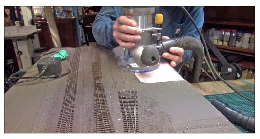
15. Turning my attention to the diorama where the building will sit, I used a router and a hot foam cutter to cut away the foam to the depth of the Plexiglas, making for a flush fit. I then glued the building to the Plexiglas base.
