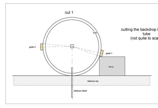
7. My CAD program and a bit of high school geometry showed that we needed to slice a 198.4° segment from the shipping tube. The question was, how? Ripping it on the table saw would most likely result in non-straight edges where it would attach to the bullnose mount. Something that would provide steady support was needed.
