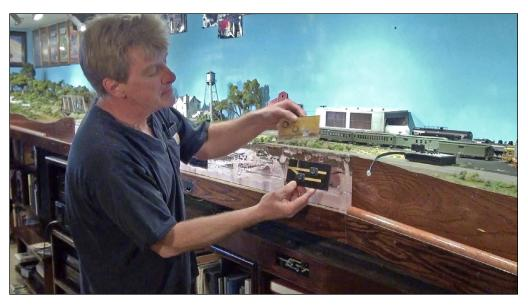
2. I cut a piece of Plexiglas to the size of the new panel and cut holes for the rocker block switches.
