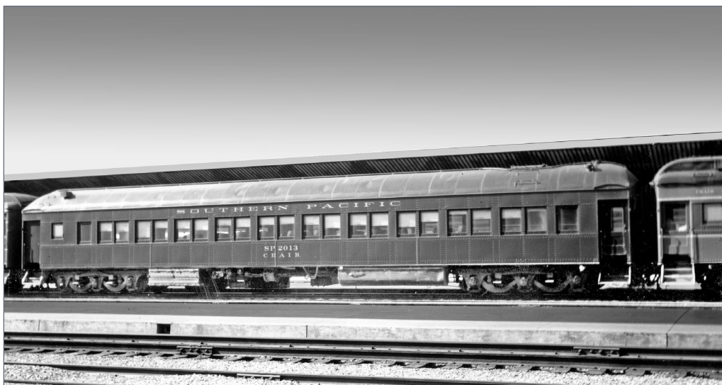
26. SP's arch roof coaches can be simulated by adding a round roof to the Walthers model and removing the fish belly underframe. Courtesy Bob's photos
