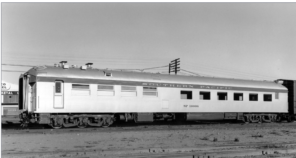
11. Class 77-D-4 dining car, nearly identical to 77-D-3. Kitchen side of car 10006 shown in the mid-1960s in imitation stainless steel with red letterboard paint. Courtesy Bob's Photos
