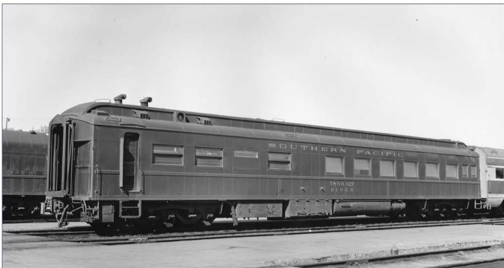
15. Texas & New Orleans RR (SP subsidiary) car 927, kitchen side. Class 77-D-9 with ice air conditioning boxes shown coupled to Texas and Pacific car. Courtesy Bob's photos
