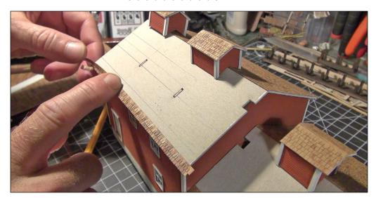
13. Simply peel and stick each row of shingles on to the roof sections. I draw lines on the roof to help keep the rows of shingles even.
