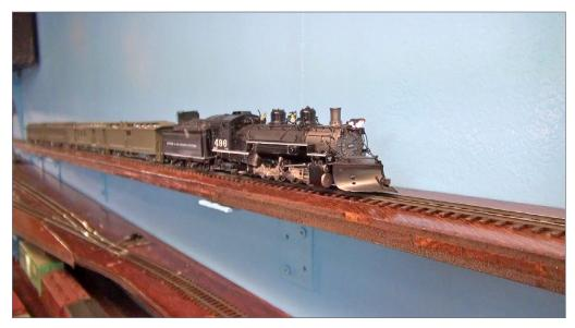
23. I have this K-37 scale brass model that could not pull four older brass passenger cars up a 4 percent grade. The brass trucks from the '60s don't roll very well and have a lot of drag. The solution was to replace the older trucks with free-rolling new Blackstone aftermarket passenger car trucks, reducing the pulling drag from 1.2 ounces to a half-ounce. Now the locomotive can easily pull the train up the 4 percent to the upper town.
