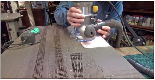
15. Turning my attention to the diorama where the building will sit, I used a router and a hot foam cutter to cut away the foam to the depth of the Plexiglas, making for a flush fit. I then glued the building to the Plexiglas base.
