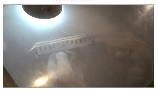
21. Here you see the inside of my North Coast sandblaster. I am using a full-size ceramic gun with 220 grit aluminum oxide. This size is very fine and will not pit the brass. I used about 50 psi of air pressure during this process. A vacuum system sucks the sand out of the air in the booth to allow a clear view of the work.
