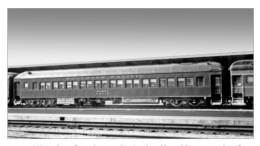
26. SP's arch roof coaches can be simulated by adding a round roof to the Walthers model and removing the fish belly underframe. *Courtesy Bob's photos*
