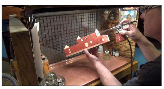
9. Using an airbrush, I painted the main walls with Floquil Tuscan paint. My formula is 25 psi of air pressure, and the paint thinned 50 percent.
