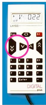
3. Lenz LH100 button control throttle – the down speed controls are circled, the up speed controls are the buttons on the right.
