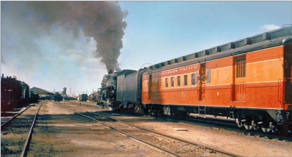
15. Prototype SP 80-BP-60 baggage/RPO cars in service, mid 1950s. Courtesy Bob's Photos
