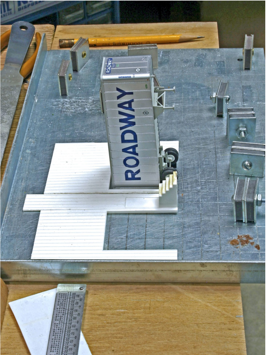
17. Marking out the openings for truck loading bays, using a trailer as a guide.
