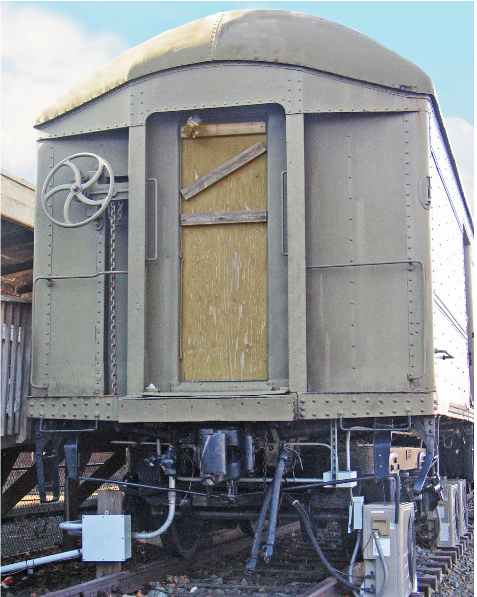
8. Blind end of Lackawanna baggage car, a typical arrangement similar to SP 80-BH-1 cars. The end sheets of the car are flat and are mounted to the inside of the collision posts framing the door.
