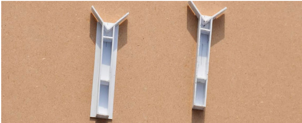
29. To construct the concrete columns, I cut strips of .040" styrene 24" wide and cut to length. I then faced the center section with .030" styrene at a width of 30". I filed the columns and chamfered the corners to represent standard concrete construction practice.
