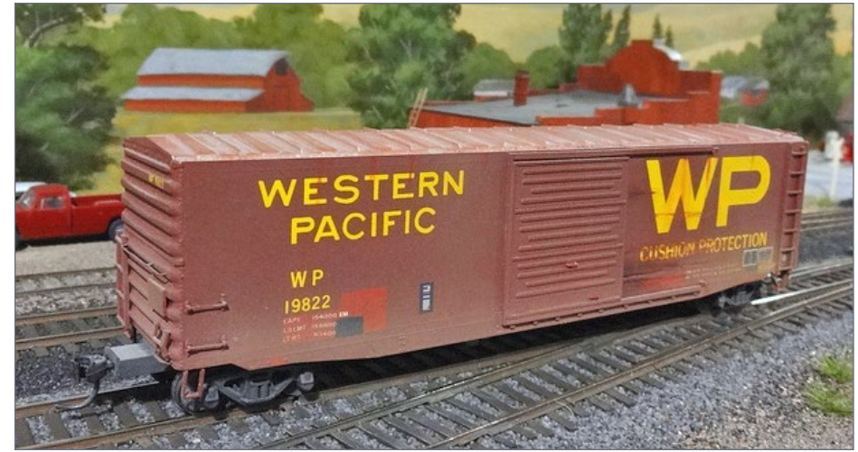
2. This car has not changed ownership, but has multiple patches from repairs and changes to stenciling. The capacity data is white, decaled atop the oxide red patch. Rob Spangler photo
