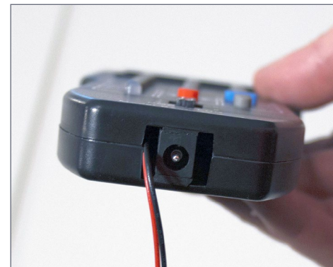
3. Bottom view of the MRC Decoder DR., showing the programming track wires and the socket for the wires from the transformer.
