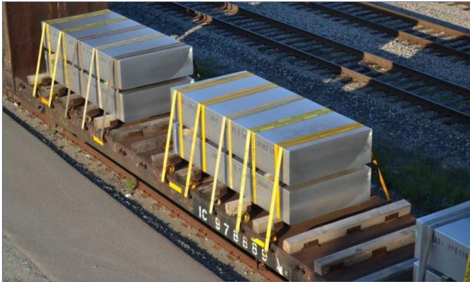
26. This photo shows the position of the tie-down straps. Notice how taut they are.
