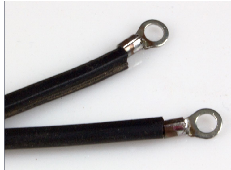
10. Ring terminals for 18 to 22 AWG wire (red sleeve removed) soldered to foot-long 18 AWG drop wires.
