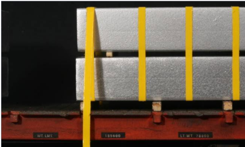
27. When applying the striping tape as tie-down straps, allow any extra to extend below the flatcar.
