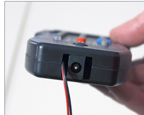
3. Bottom view of the MRC Decoder DR., showing the programming track wires and the socket for the wires from the transformer.
