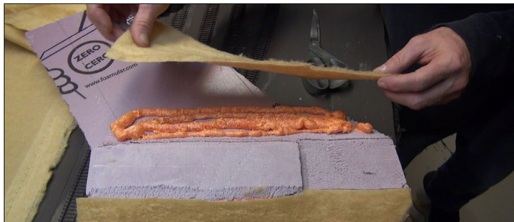
13. Gluing the fake fur to the foam.
