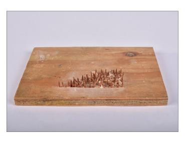
4-5. Scrape the shaped dowel with this nailed block.
