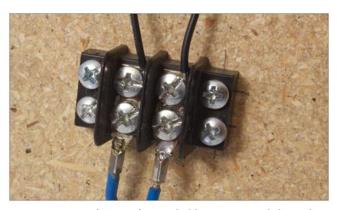
14. Large gauge (16 AWG) stranded bus connected through a barrier terminal strip to a smaller gauge (20 AWG) solid wire.
