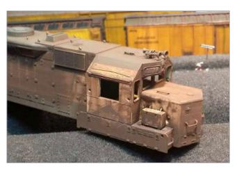
34. After sealing this layer of weathering with Dullcote I again mixed raw sienna and burnt umber, but this time about 50/50 to produce more of a brown-colored older rust. This color needs to
