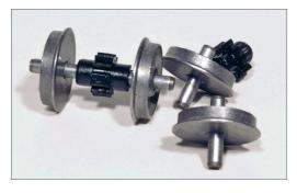
6. Examples of unassembled and reassembled wheel sets. An NMRA standards gauge is used to check wheel gauge before reassembling the truck. The axle gear should be centered on the axle.
