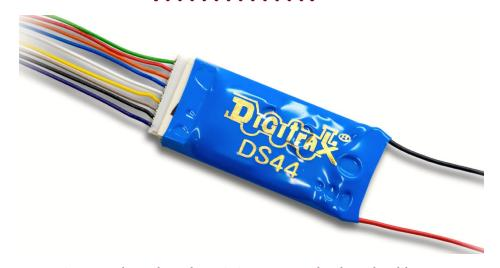
1. Stationary decoder: the Digitrax DS44 looks a lot like an HO mobile decoder, just with more wires. It handles four stall motors. Digitrax photo
