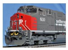
Kato USA plans to deliver new GE C44-9W locomotives decorated for SP and UP in September. Two numbers will be available for each road. Upgrades over previous releases of the ready-to-run model include a redesigned battery box area, the
