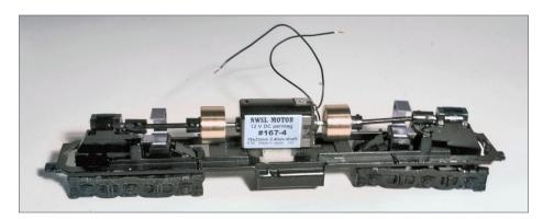
12. Reassembled drive train with replacement motor. Clear silicone adhesive and sealant was used to attach the motor to the frame.
