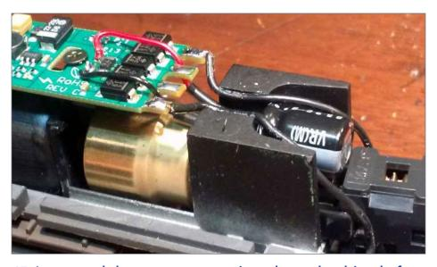
47. I mounted the separate capacitor above the driveshaft and attached its heat-shrink tubing to the metal frame protrusion with a drop of super glue to hold it in place, yet still be removeable. I tucked the truck power leads into the frame as well, leaving a flat surface to mount the speaker. I solder all of my connections for reliability.
