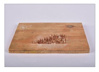
4-5. Scrape the shaped dowel with this nailed block.
