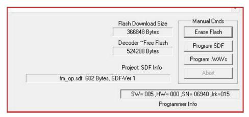
11. Lower right corner screen shot of SoundLoader showing the memory used by the sound project (Flash Download Size). The sound project cannot exceed the memory space available on the decoder. This screenshot was captured after I had erased the flash memory and the decoder's entire flash memory of 524,288 bytes is available (free).
