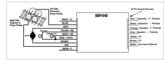
4. Digitrax SDH164D decoder pin configuration. Digitrax instruction manual
