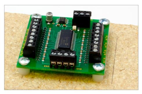
2. NCE Button Board mounted to particle board using #6 x  $^{3}$ /4 screws and nylon standoffs.
