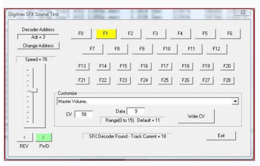
C. Screenshot of the Sound Test function. One benefit of SoundLoader is the ability to test the sounds and functions of the decoder while still on the programming track.
