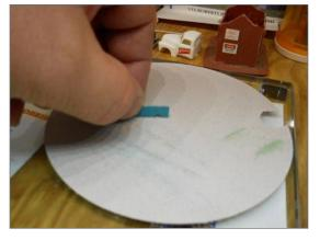
4. Use sandpaper on a self-adhesive orbital sander disk, laid against a piece of glass, to get a totally flat and true surface.
