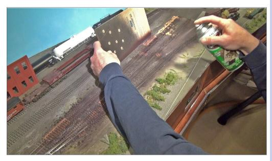
9. Spraying the Rustoleum camo onto the track and foam.
