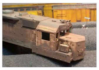
34. After sealing this layer of weathering with Dullcote I again mixed raw sienna and burnt umber. but this time about 50/50 to produce more of a brown-colored older rust. This color needs to
