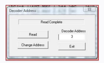
B. Decoder Address screenshot. After selecting Read, Sound-Loader confirms the decoder address is 3. This screen can also be used to change the decoder address.
