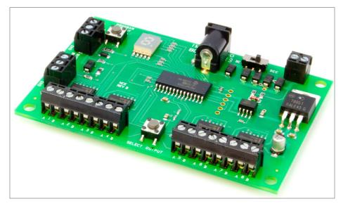
6. NCE's Switch 8 MK2 for eight stall motors includes a jack for external power.
