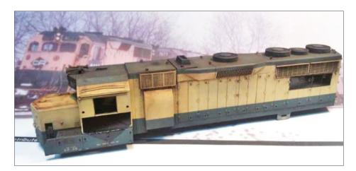
43. Here's the result with the masking tape removed. These patch jobs were carried out by shop forces in a hurry and were done with paint rollers, spray cans, or anything else available that day. Neatness is not a requirement here! Imperfections are visible in almost any prototype photo.
