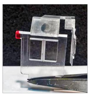
45. I re-used the factory Kato cab glass on this model, but I don't like the way the glass pieces rub against each other while removing or installing it, causing scratches. To work around this I cut the tab off the side window piece (shown in red).
