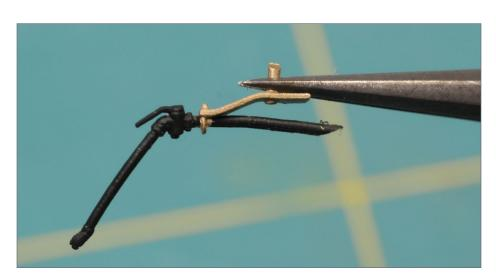
8. A Precision Scale Part 39156 bracket with a Hi-Tech 6038 air hose. I drilled out the hole in the bracket with a #77 drill and then finished up with a #74 drill. Cutting the end of the air hose on an angle helps thread it through the hole.
