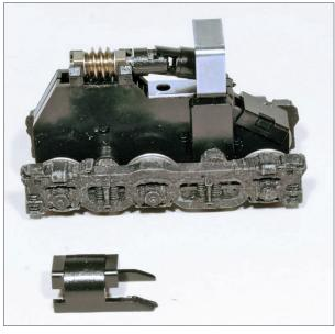
2. Clip holding truck to chassis has been removed, allowing the truck assembly to be removed from the frame.
