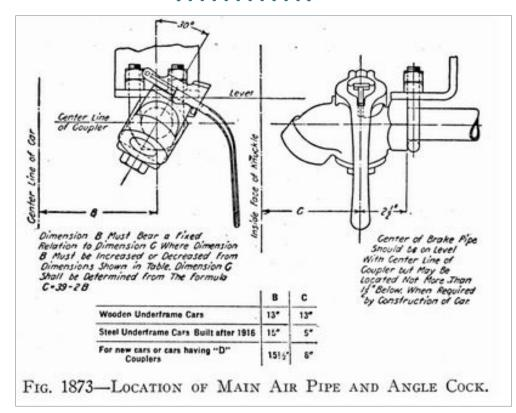
9. This illustration from the 1922 Car Builder's Cyclopedia shows how the angle cock for the air hose is tipped 30 degrees toward the coupler. This American Association of Railroads (AAR) standard makes it easier to connect the air hoses on two adjacent cars.
