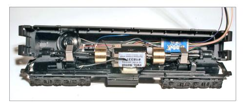
3. Prior to installing the lights, check the positioning of all the components in the hood to ensure adequate clearance for the drivetrain.
