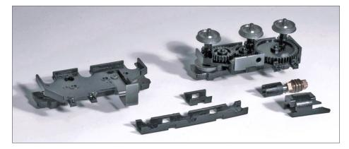
5. All of the truck components have been disassembled and cleaned in preparation for replacing the wheelsets.
