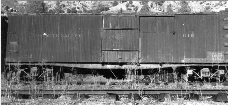
2. YV 610, one of the three ex-SP B50-1/2/4 box cars on the roster, at El Portal. The black side sill is very light, suggesting that it was not repainted by the YV after purchase. The rest of the car was repainted by the YV. The area with the capacity data on the bottom left of the car appears to have been left untouched. Stanley Snook photo
