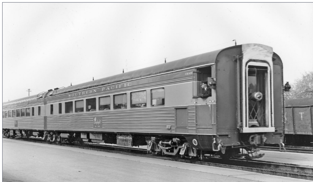
14. SP 2471+2472 articulated chair car pair, class ACW-66+ACM-66, shown in 1955. The retracted staircase in the rotating unit is shown, and at left is the baggage elevator door. Courtesy Bob's Photos
