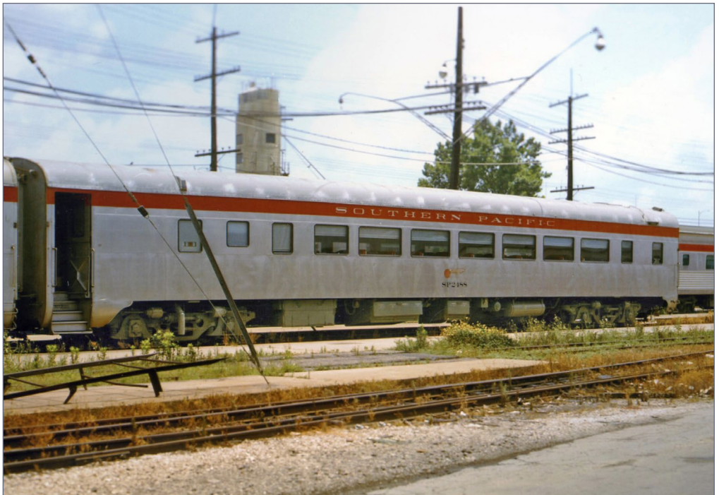
21. Prototype chair car 2488 (class 79-C-2) in 1969 as re-built with flat stainless sides, but with its original triple bolster trucks.
