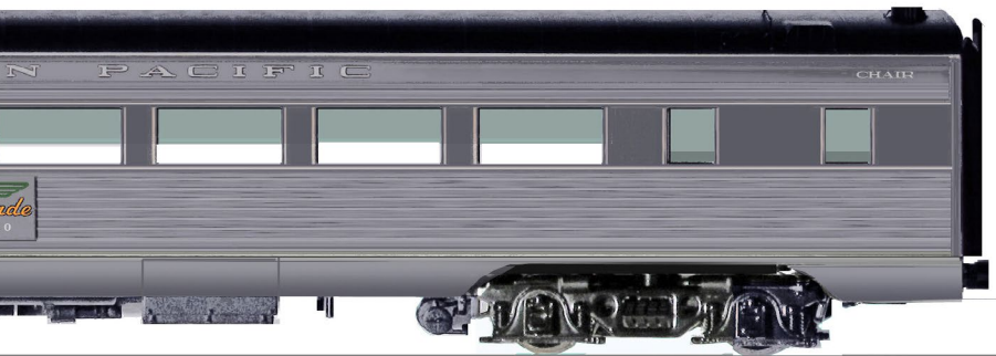
ORIGINAL TRIPLE BOLSTER TRUCKS
