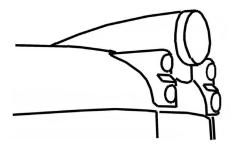
9. Observation car lighting arrays which replaced the single recessed lamp of the original parlor observation cars.
