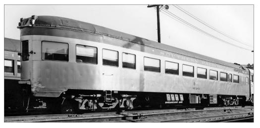
19. Parlor car 2951, class 77-PRO-1 parlor observation in its final configuration shown in San Francisco as of April 1971. The car has late box type rear lighting array, flat stainless steel sides with red letterboard stripe, and Waukesha air conditioning. Propane bottle containers show under the car. This car still has its triple bolster trucks.
