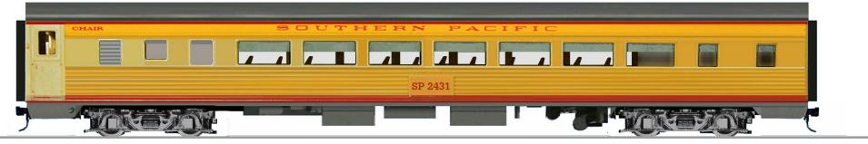
THE RELETTERING OF EQUIPMENT TOOK UNTIL ABOUT 1948, AND DURING THE 1950s SOME CHAIR CARS RECEIVED MORE MODERN TRUCKS REPLACING THE OLD TRIPLE BOLSTER TYPE. (BY THE 1950s THE CENTER SKIRTS WOULD HAVE BEEN REMOVED FROM THESE CARS)
