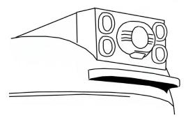
The center flush-mounted light was usually replaced with an oscillating Mars light. Some of the cars, as 2954, 2955 and T&NO car 951 had their Mars light set in a raised fairing while other cars such as 2950, 2951 and 2953 kept their flush mounting for the Mars light.
