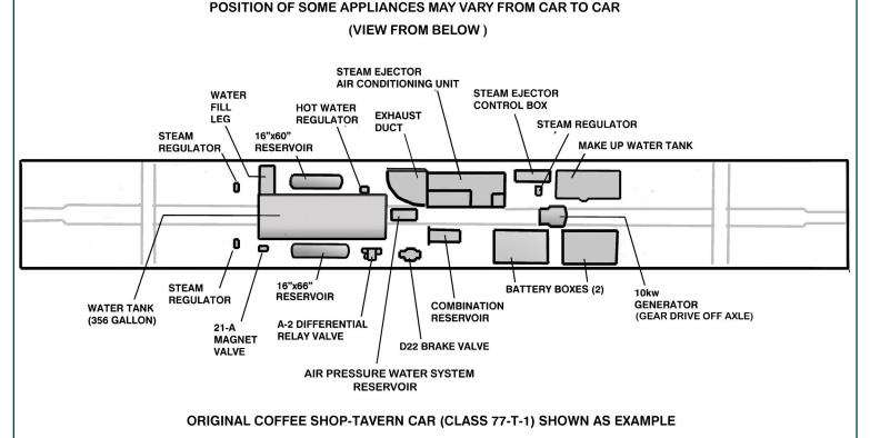
UNDERBODY EQUIPMENT ON DAYLIGHT CAR SHOWING CARRIER-SAFETY STEAM EJECTOR AIR CONDITIONING INSTALLATION
