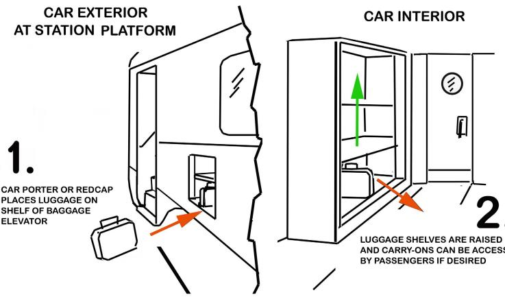
13. Baggage elevators were used to prevent delays at stations. In lowered position they could be accessed from the outside sliding door, and when raised, the carry-on luggage was accessible for passengers in the car.
