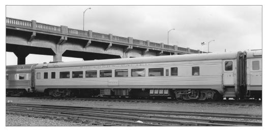
17. Chair car in the later lettering for Overland service, car 2432 in class 77-C-3. The drop-equalizer type trucks are replacements, usually taken from a scrapped sleeping car The car still has its original fluted sides. *Courtesy Bob's Photos*
