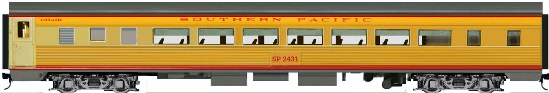
THE RELETTERING OF EQUIPMENT TOOK UNTIL ABOUT 1948, AND DURING THE 1950s SOME CHAIR CARS RECEIVED MORE MODERN TRUCKS REPLACING THE OLD TRIPLE BOLSTER TYPE. (BY THE 1950s THE CENTER SKIRTS WOULD HAVE BEEN REMOVED FROM THESE CARS)
