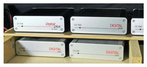
9. On my HO Siskiyou Line, I use centrally-located Lenz LV100 bosters, rated at 3.5 amps each, for my five power districts. However, as I add more sound units to the layout, I'm finding a need to move up to 5 amp boosters. Because I'm using subblock current limit protection wiring, moving to higher amp boosters won't cause any problem.
