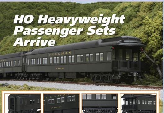
Check out the quality and value found inside the M.T.H. HO heavyweight passenger cars now arriving at your local M.T.H. Authorized Retailer. An intricately detailed, durable ABS body rides atop smooth rolling trucks that won't bog down a locomotive struggling to pull heavy passenger cars. Detailed car interiors, detailed car undercarriage, Kadee couplers and overhead, constant voltage flicker-free LED lighting ensure that these cars won't disappoint.
