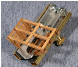
AC-1-1 "Original Right Clamp" m used for Bulkhead Assembly.
