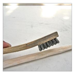
I use a wire brush to add the "bark" effect to my tree trunks. You'll find that the softness of the balsa allows the brush to cut into the wood easily. Take care to avoid warping. One way to minimize warping is to turn the trunk frequently as you add your bark texture.
