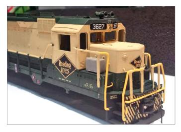
29. After Conrail was created, cab signals were installed on many locomotives to allow them to lead trains in ex-Pennsy cab signal territories. I used a Detail Associates cab
