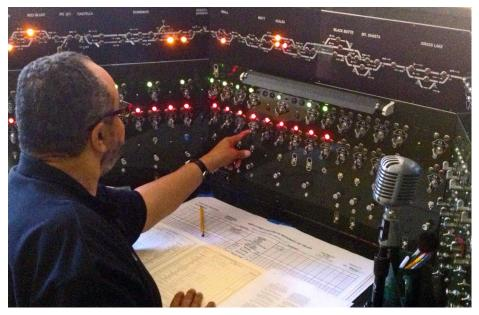
4. This model of the Canyon Dispatch machine is being operated by Otis McGee on his layout. It works through JMRI's PanelPro to control signals and turnouts. Photo courtesy Bob Jacobsen
