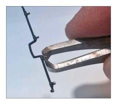
23. I installed the factory uncoupling levers that were painted black, along with the step wells and pilots painted earlier. After a coat of paint, their diameter grew, and they no longer fit into the holes in the pilot. To remedy this I used my sprue nippers to gently grab the mounting pin. I turned the nippers around the mounting
