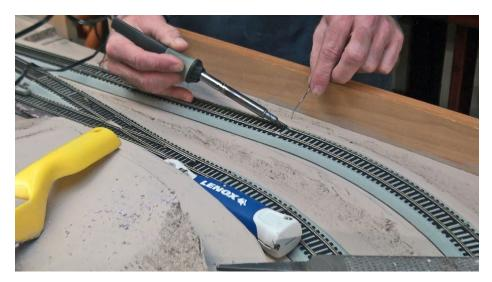
I use resistance soldering to add jumper wires to garden railroad track. It works well on code 250 rail without melting because it produces a great amount of heat in less than a second. The rail quickly gets very hot at the joint, without spreading very much. This tool also works great for fabricating brass models.
