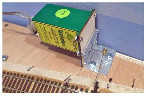
25. Switch machine mounting bracket.
