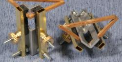
AC-2-2 "Mini Right Clamp"<sup>TM</sup> used for gluing Bulkhead Frames.
