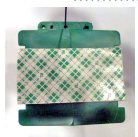
17. Attach the switch machine with double stick tape.
