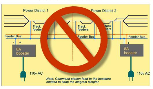
6. Don't be tempted to think of using fewer high amperage boosters. The higher amp boosters generally cost a lot more and they can do some serious damage in the smaller scales (S scale and below) when equipment derails and you get a short. High amperage boosters should be limited to the larger scales like O and G scale. This is a common best practice, but there may be some exceptions. See the text for details.
