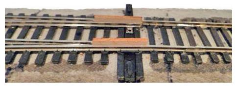
29. Place strip wood between the point and stock rail on each side.
