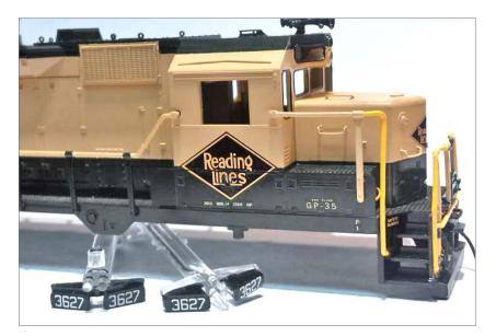
26. I made sure to paint the areas around and behind the number boards so no light bleeds through. I followed up with two more coats of gloss after decaling to hide any edges. In this photo you can also see that I've outlined the number board and window gaskets with a black Sharpie marker. After weathering and Dullcoat, it will look great.
