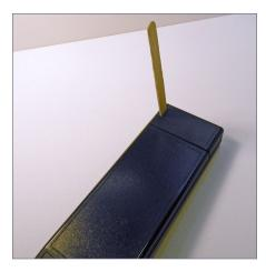
Put the battery cover back on the throttle and test-fit it. The Popsicle stick should slide into the slot and go between the positive terminal on the battery and the electrical contact, disconnecting the power in the process. You shouldn't have to force it; it should slide into place.
