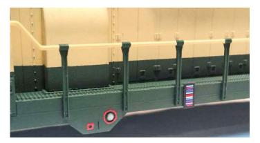
30. The ACI placard glued to the side sill, and the Fuel Filler and Emergency Fuel Cutoff button outlined in red.
