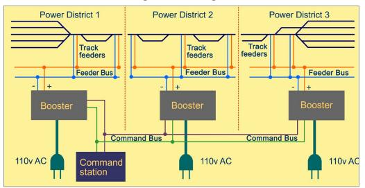
3. Better is to break up your layout into power districts, with each district powered by its own booster. This article details how to do this using DCC bus wiring best practices.
