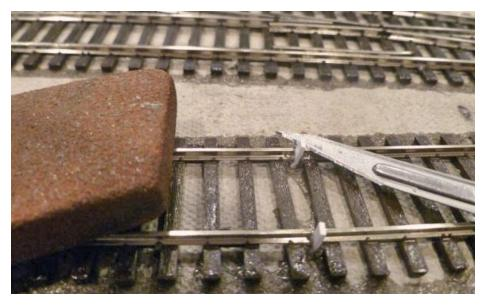
7. Trimming the top and sides of the styrene strip.
