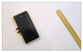
Take the battery cover, and mark where the positive electrical contact lines up. Make it wide enough for the popsicle stick.
