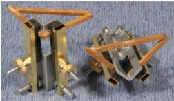
AC-2-2 "Mini Right Clamp" m used for gluing Bulkhead Frames.
