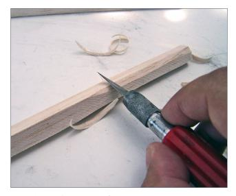
Using a sharp blade, cut the balsa sticks to their appropriate heights. For full-grown HO scale pine trees, cut your trunks 8 to 10 inches tall. Once cut to size, take your knife and slowly start tapering the balsa
