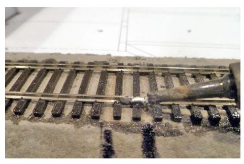
10. Soldering the feeder wire to the rail.
