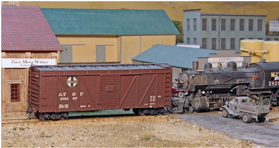
8. The distinctive Santa Fe raised-roof rebuilds of classes Bx-12 and -13 are true signature cars, being unlike any other railroad's boxcar. This model is from Westerfield kit no. 4751.
