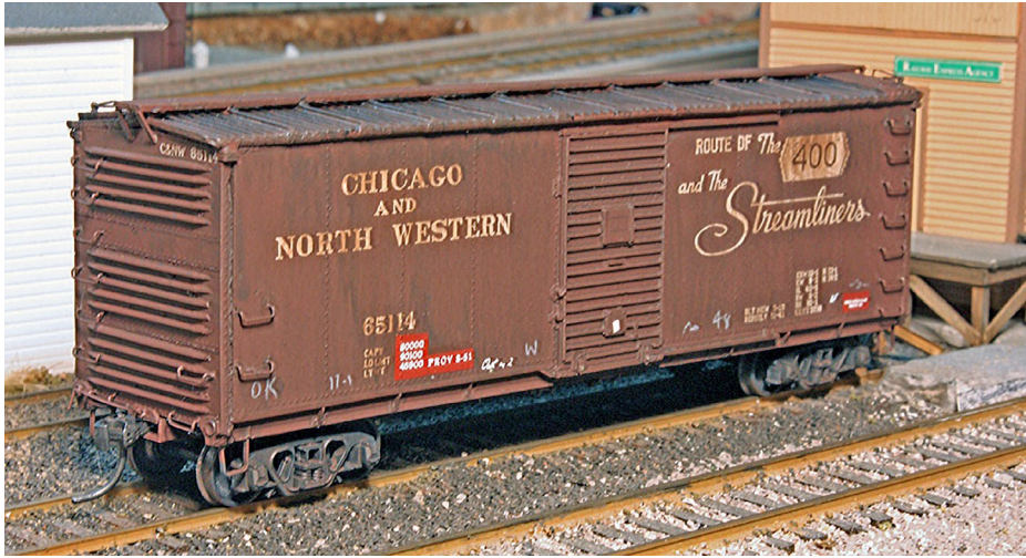
15. This model depicts one of C&NW's rebuilt USRA double-sheathed boxcars, with extended height indicated by the smooth added panel in the corrugated end. It was built from the second kit ever produced by Sunshine Models (kit 2.1) by Dennis Williams, and lettered and weathered by me.
