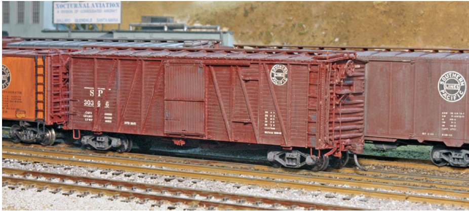
11. Southern Pacific's class B-50-14 cars were built in large numbers, but were being scrapped rapidly after 1950. This photo shows a model of one of these cars with a retrofitted Dreadnaught end, a change made for most -14s in the 1930s. It was built from Sunshine resin kit 17.18.
