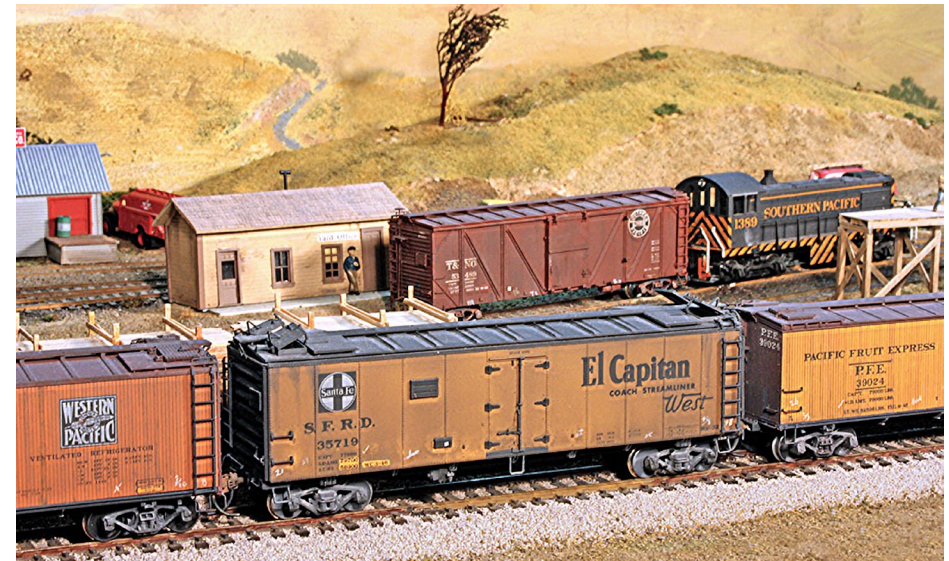
10. A representative of 18,000 refrigerator cars operating under SFRD reporting marks, this model of class RR-32 shows the inward-opening ice hatches standard in SFRD practice until the 1950s (they were later reversed to accommodate icing machines). It was built from an InterMountain kit by Richard Hendrickson.
