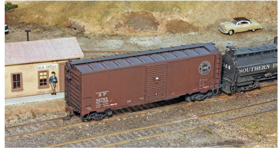
12. This Innovative Model Works kit represents SP class B-50-21, which were 2,000 of the 5,244 cars built like this for SP, with the distinctive W-corner-post ends.
