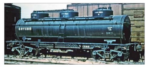
8. The John H. Grace & Co. owned GRYX 815 when it was photographed in the 1950s. It was built in March 1927 by the Pennsylvania Tank Car Co., a subsidiary of the Petroleum Iron Works. PTC was located right next door to the Standard Tank Car Co. in Sharon PA and installed tanks built by STC on its own underframes. Chuck Yungkurth collection
