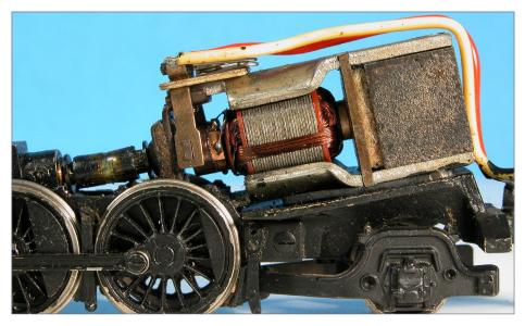
2. Older, inefficient, open-frame 3-pole motor. Note also the aged piece of tubing used in the drive line. Mark Schutzer photo
