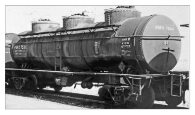
13. Formerly Associated Oil Company AOX 600, this threecompartment 6,000 gallon car was built by the Pennsylvania Tank Car Co. in the early 1920s using a tank supplied by the Standard Tank Car Co. By the time this photo was taken in Avon, CA in June 1972, Phillips Petroleum has acquired the Associated tank car fleet and renumbered the cars under PSPX reporting marks. Robert A. Campbell photo
