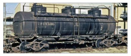
11. This 6,000 gallon three compartment car, built by General American in the mid-1920s, is seen here in the 1970s with elaborate handrails added to the dome running boards and lots of rust showing. DRDX was the reporting mark for the Duredo Co., a tank car lessor which first appeared in the late 1940s and specialized in refurbishing older second-hand cars. Duredo was a subsidiary of Chicago-based John H. Grace & Co. Lloyd Keyser photo
