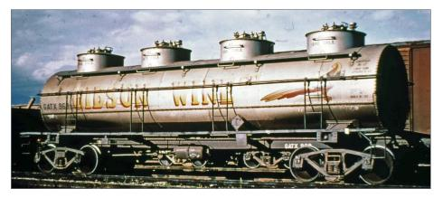
26. Four-compartment wine tank cars were usually of about 8,000 gallons total capacity. GATX 969, built in 1937, was on lease to the Gibson Wine Co. in the 1950s with colorful Gibson stenciling on its aluminum painted tank. Jim Gerstley collection courtesy of Dan Smith
