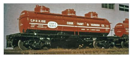
12. American Car & Foundry built this three- compartment 6,000 gallon tank car in May 1927 for the Cook Paint and Varnish Co. Note that, though freshly painted in the 1950s, this car still had its 5-27 reweigh date; tank cars were not required to be reweighed periodically, like other freight cars, because the shippers were charged by volume, not weight.
