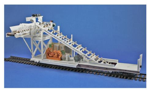
30. Diesel generator, and equipment in place.
