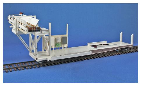
28. Machine deck with transfer conveyor added.
