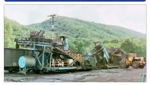
2. Photo of a prototype machine from the left front. The coal is loaded into the receiving hopper with a front end loader.
