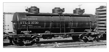
21. American Car and Foundry also built this 6,000 gallon threecompartment tank car for Union Tank Line in August
