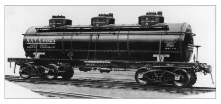
20. This American Car & Foundry builder's portrait shows a three-compartment 6,000 gallon car built on an AC&F Type 27 underframe in April 1937 for North American Tank Line. Mechanical equipment included AB air brakes and Barber Stabilized S-2 trucks with spring planks. Hawkins-Wider-Long collection
