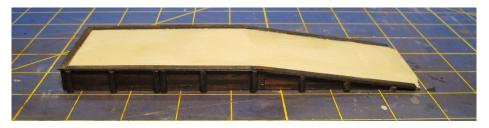
19. The dock assembly with the top chord in place on top of the dowels. I painted the Hydrocal as a color test. Next I reapplied Hydrocal to the top of deck to bring it up to the level of the top chord, and then sanded everything smooth.
