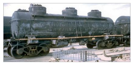
19. The number is illegible on this 6,000 gallon three-compartment General American car because it was in the process of being sandblasted and repainted at GATC's Colton CA maintenance and repair yard. A new wood running board had also just been installed. This car had formerly been in the service of the Crosby Naval Stores Co. of Pickayune, MS, a supplier of turpentine and other products made from pine sap.
