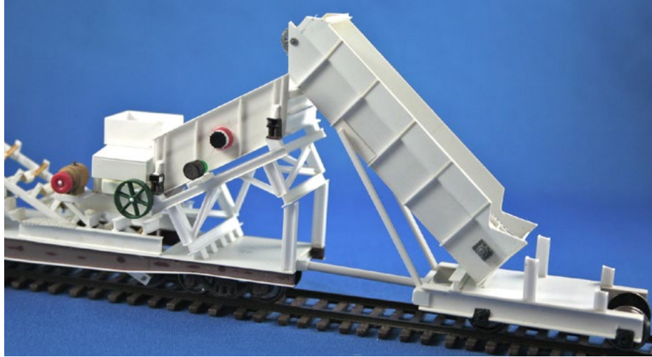
33. The trough conveyor has been added and dumps into the shaker screen. The receiving hopper has not yet been added on the far right.
