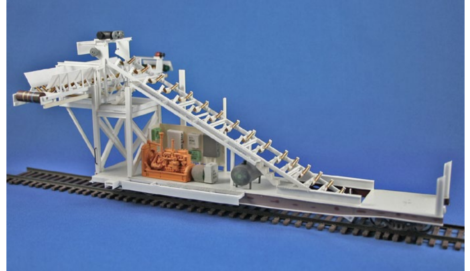
30. Diesel generator, and equipment in place.
