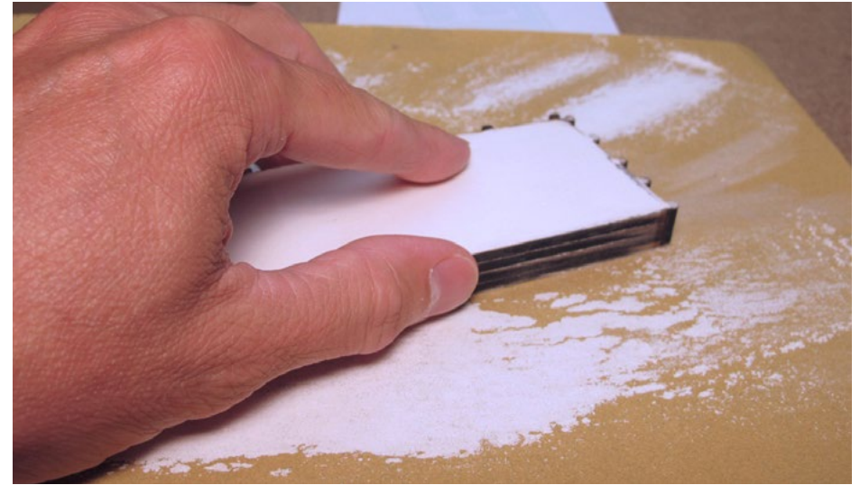
16. Sanding the Hydrocal smooth on top.
