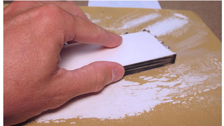
16. Sanding the Hydrocal smooth on top.
