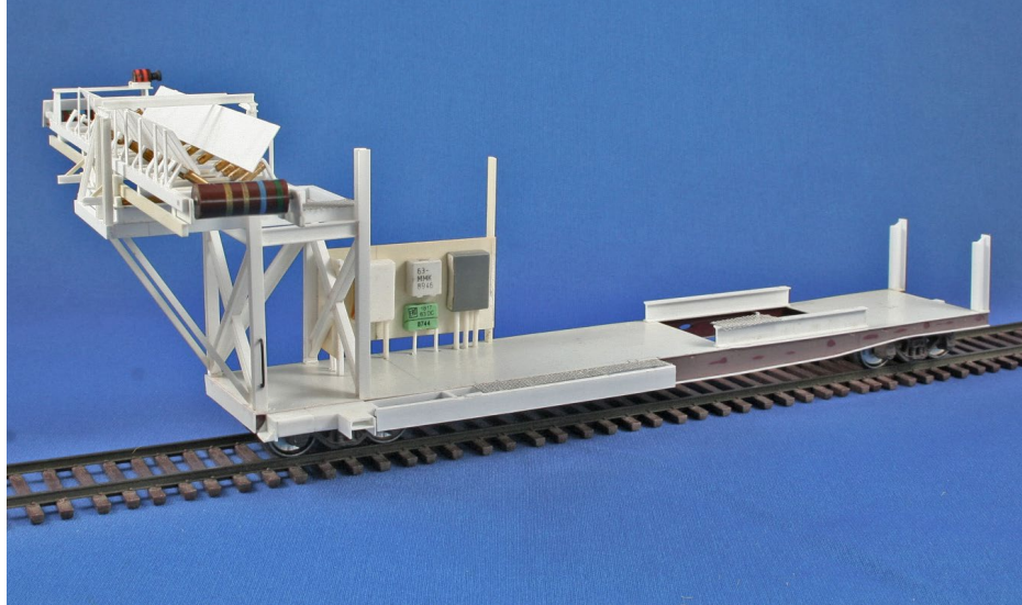
28. Machine deck with transfer conveyor added.
