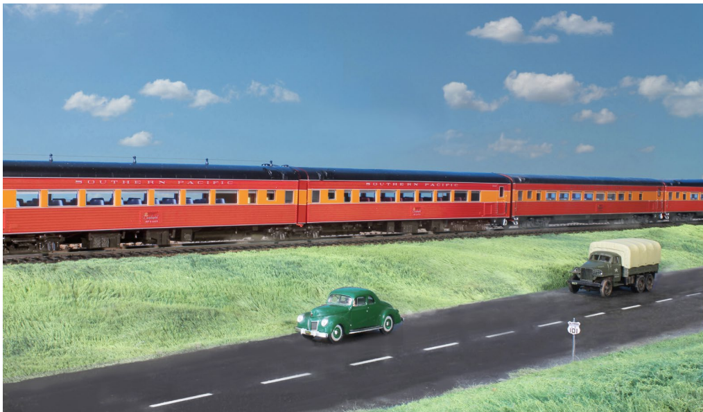
14 {top} and 15 (bottom). The Daylight's triple-unit articulated food service cars with full coffee shop and full diner bracketing the smaller kitchen car at center.
