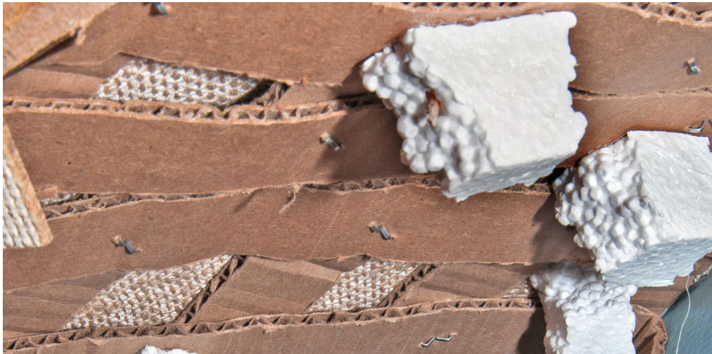
15. Beaded foam plastic blocks hot-glued to the underside of the hardshell will hold the trees in place.
