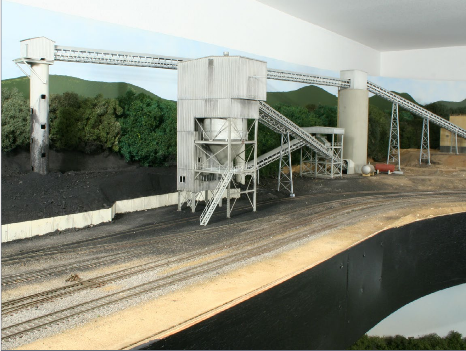
18. Coal stacker, fast loader, transfer building, concrete storage silo, conveyors, and main preparation building.
