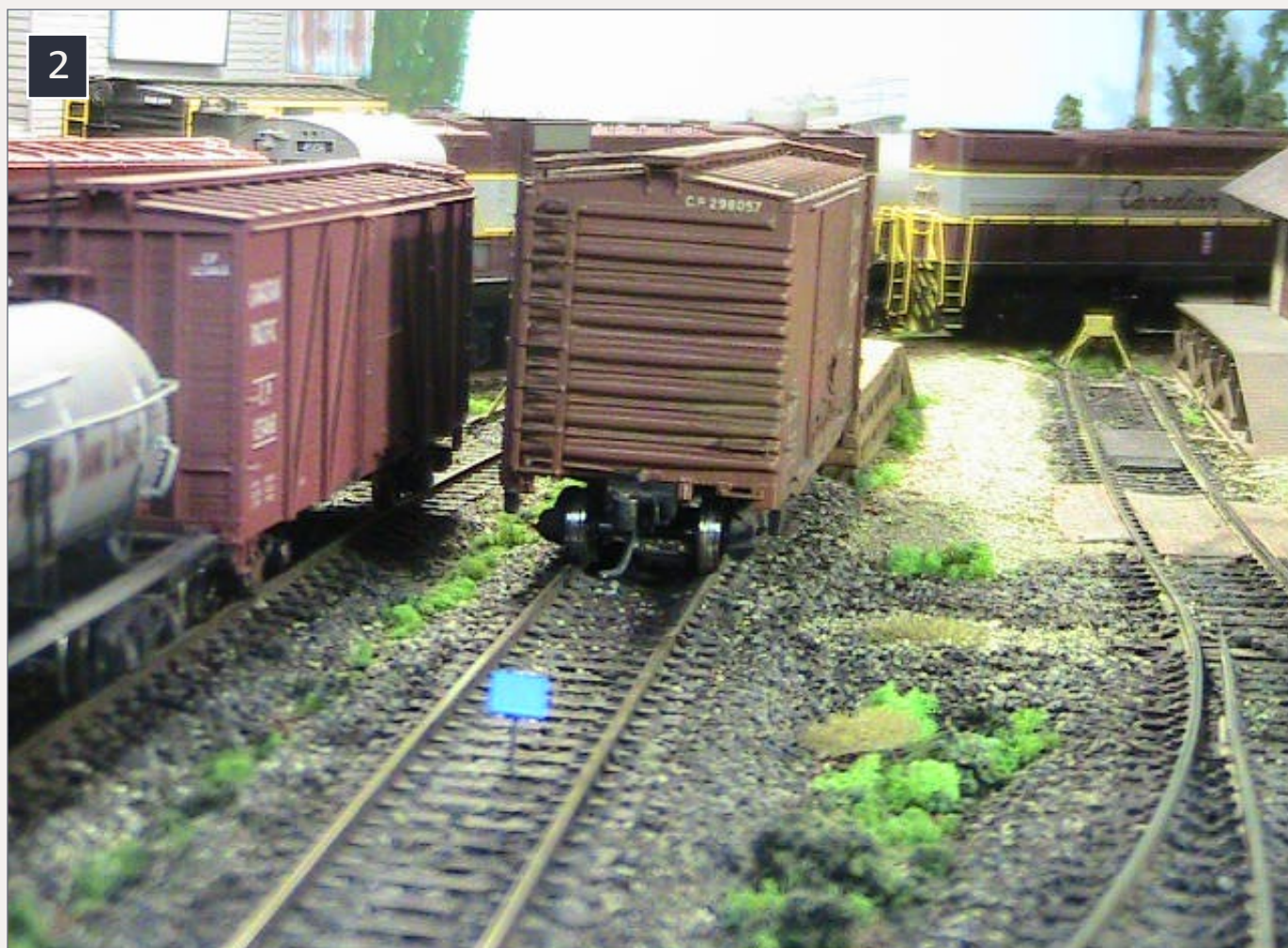
2. Simulated tie-mounted blue flag on team track.
