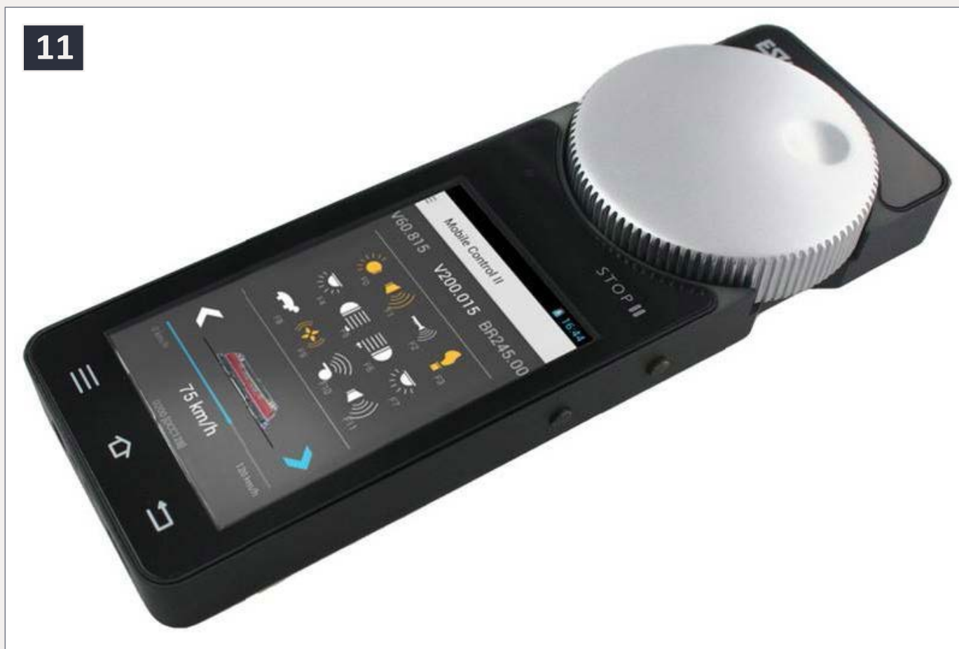
11. ESU Mobile Control II Android throttle. ESU photo.
