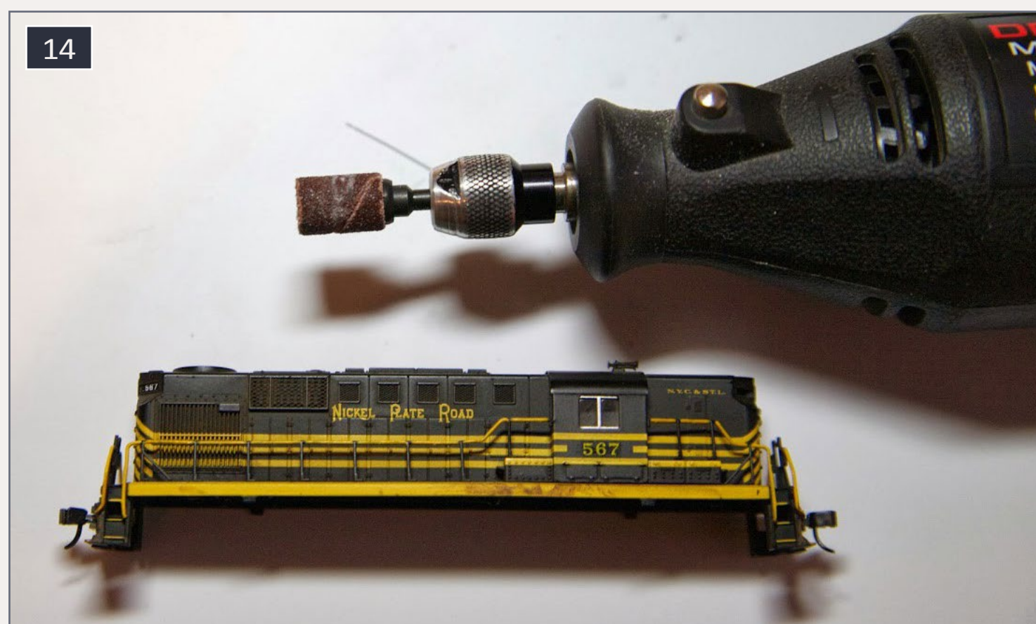
14. A drum sander is used to widen the inside of the shell.
