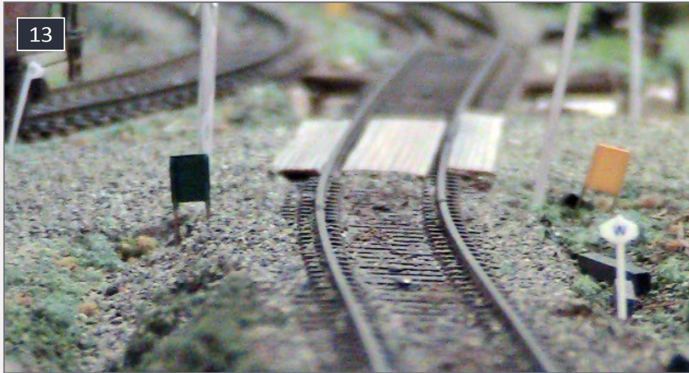
13. Model slow order, yellow flag and opposite direction resume speed green flag.
