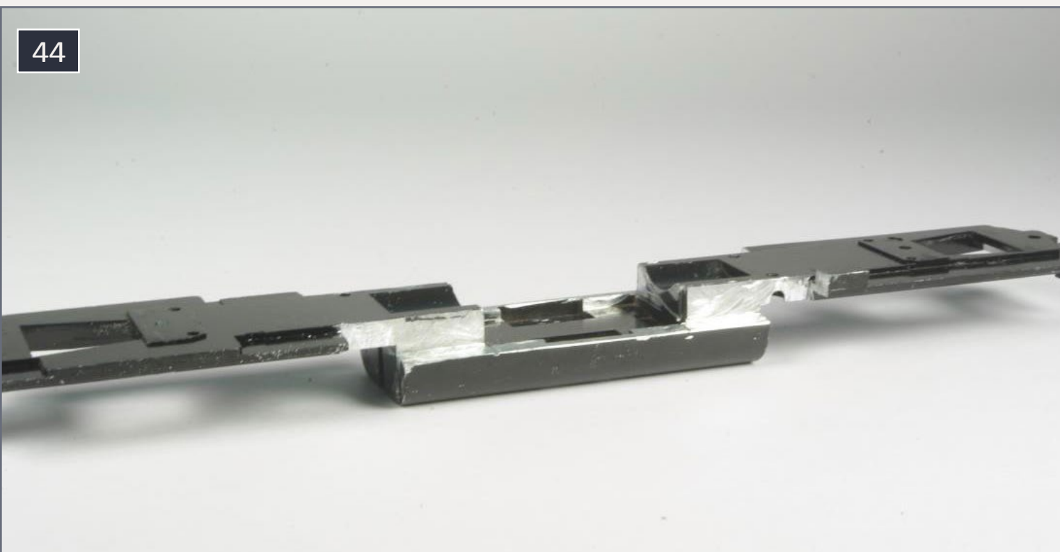
44. The frame after all cuts and milling.
