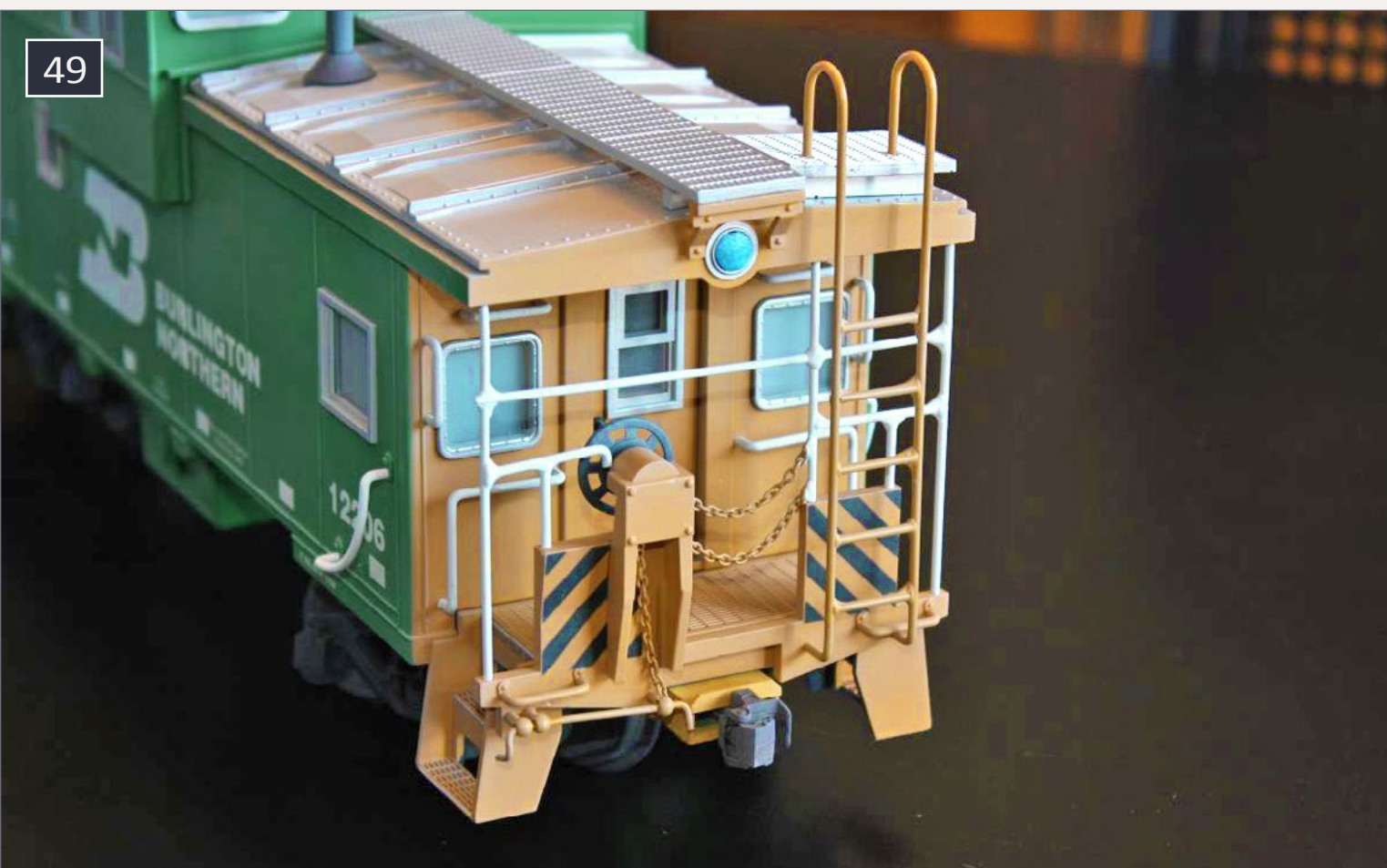
49. End rails and grab irons painted white. I placed tape over the EOT lens during the weathering stage.
