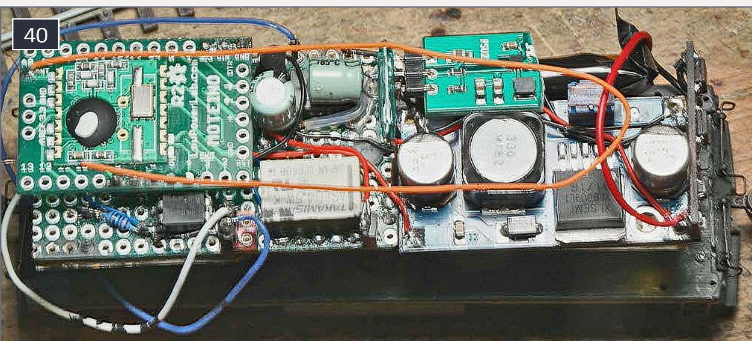
40. High power version with switching regulator.
