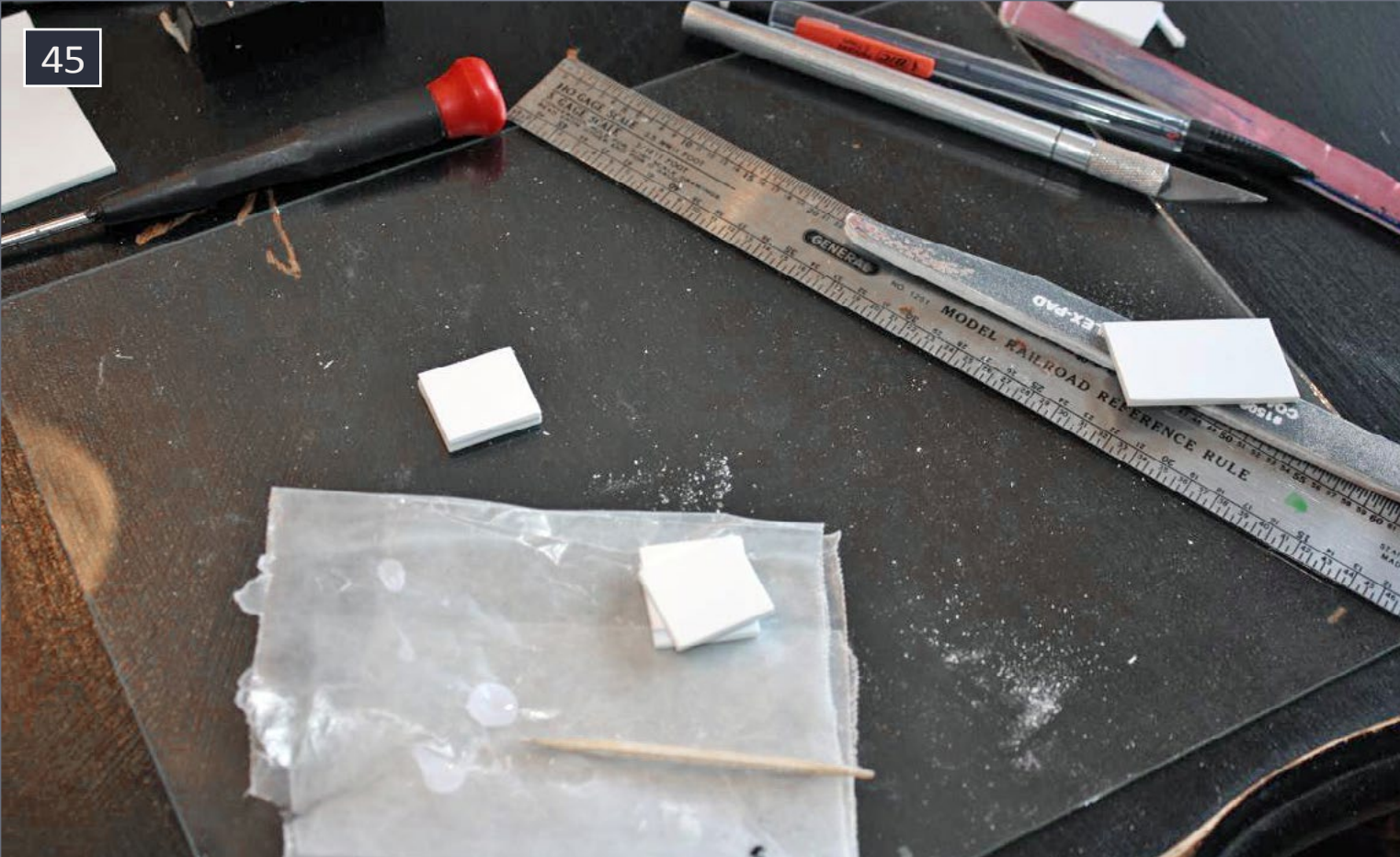
45. Building the coupler mounting box from styrene.
