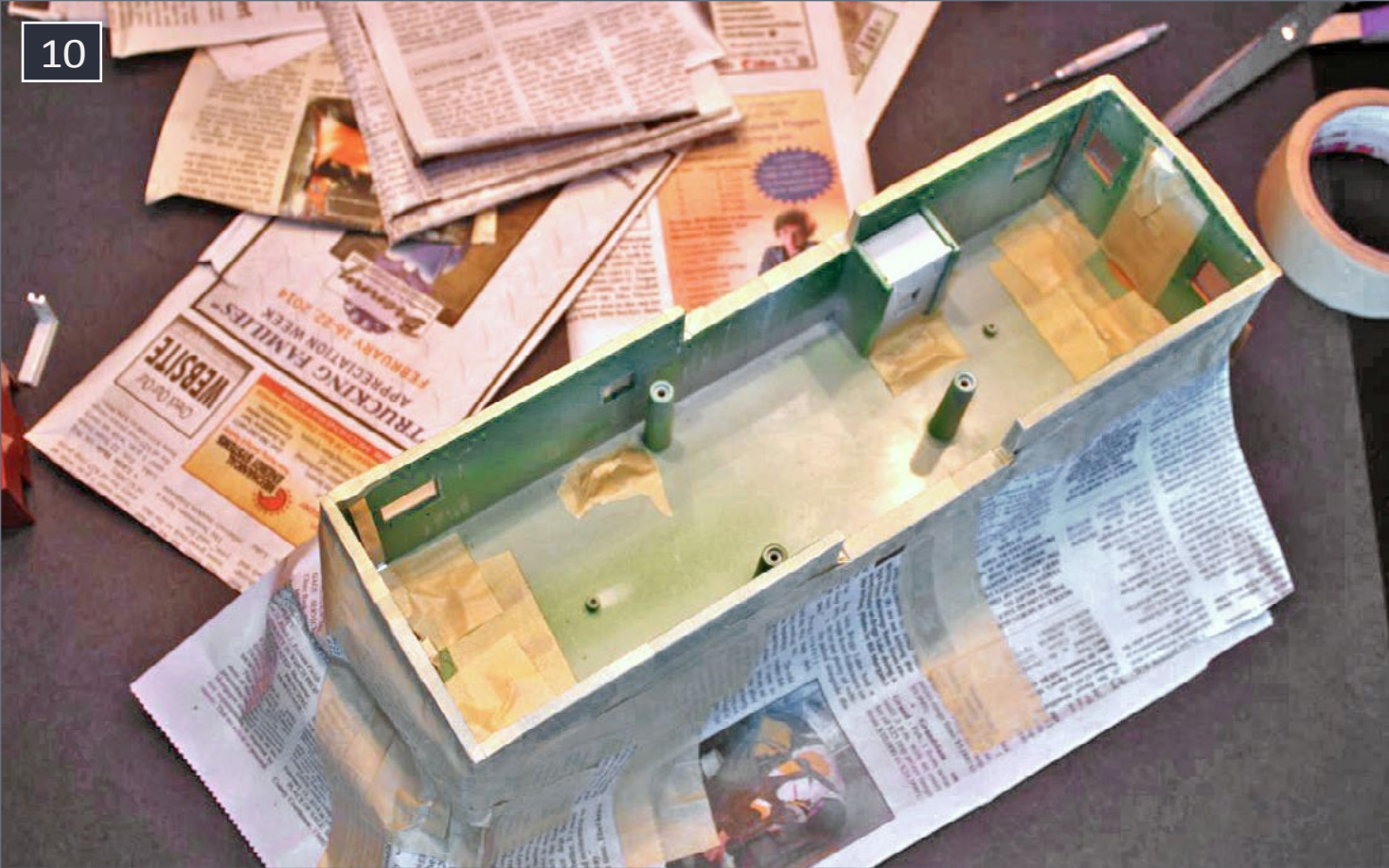
10. Getting the interior ready for painting. I wiped the interior with window cleaner and paper towels, and masked with tape and newspaper.
