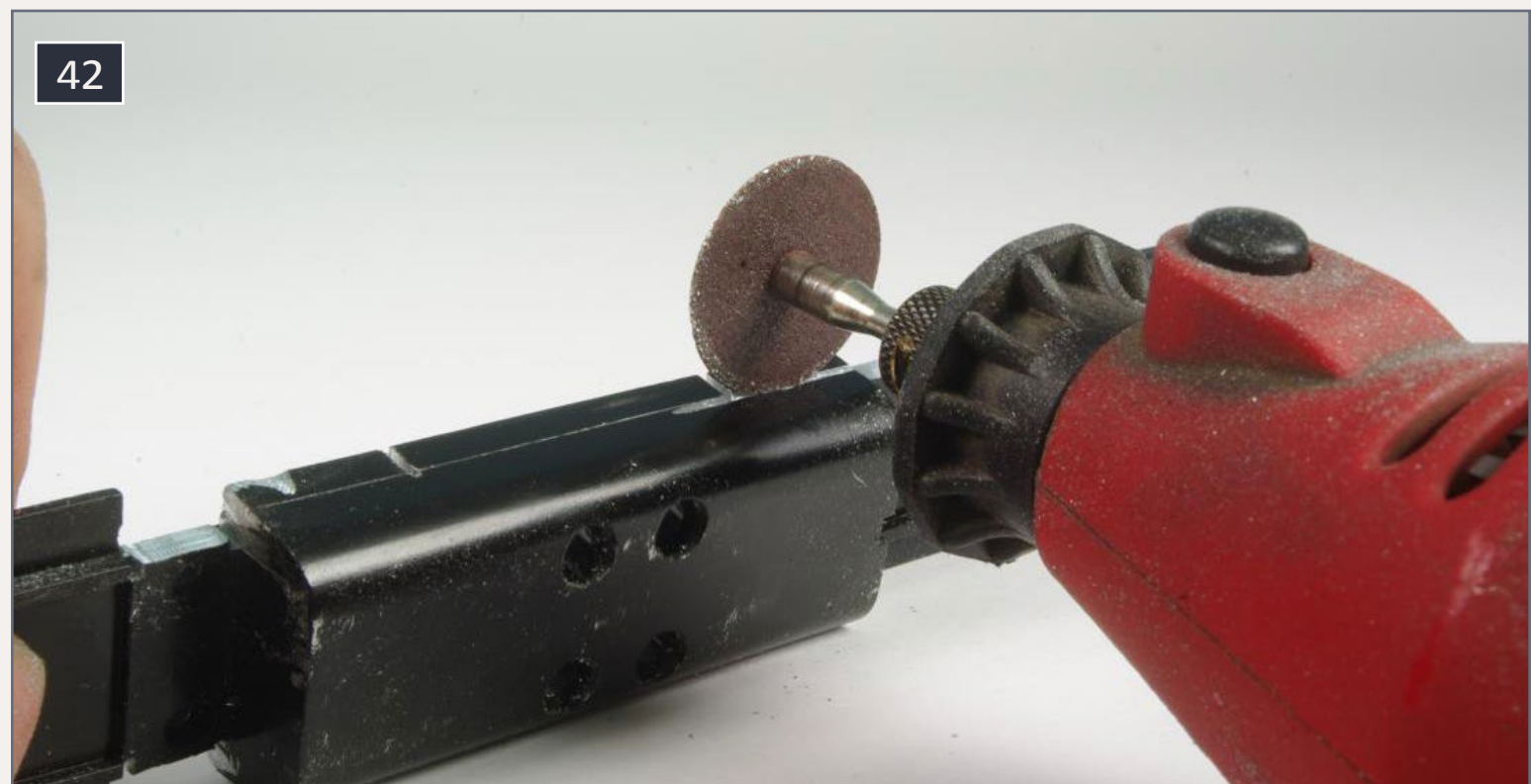
42. Making the horizontal cut to the fuel tank.
