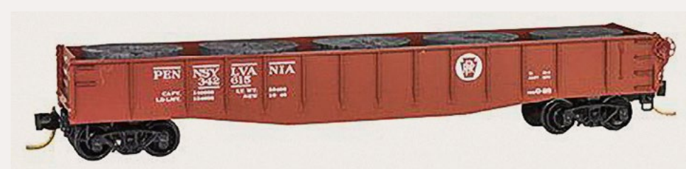
is a PRR 50' steel gondola with fishbelly sides and drop ends.
