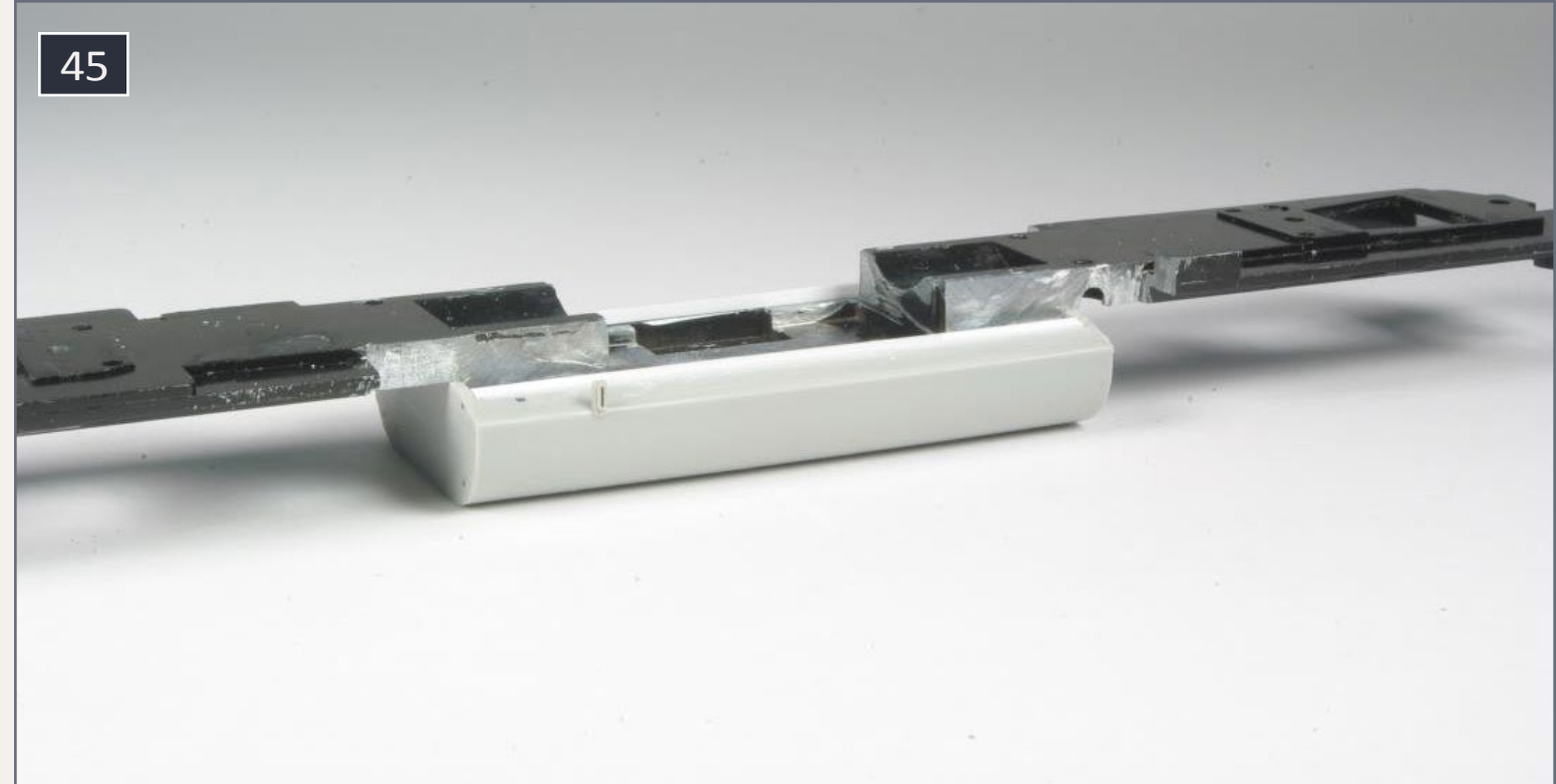
45. Fuel tank installed, styrene strip added.
