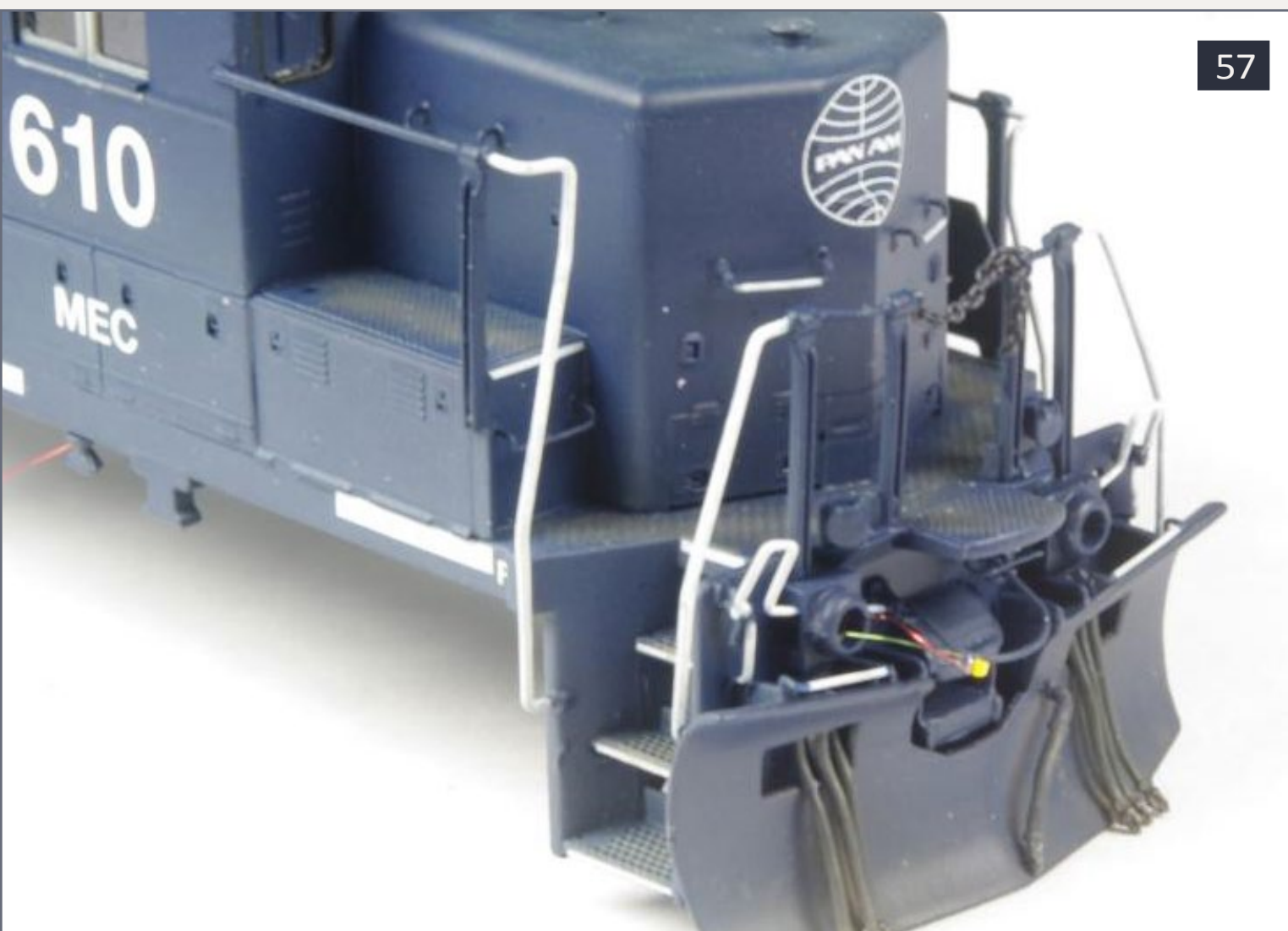
57. Installing nano-LEDs in ditch lights.
