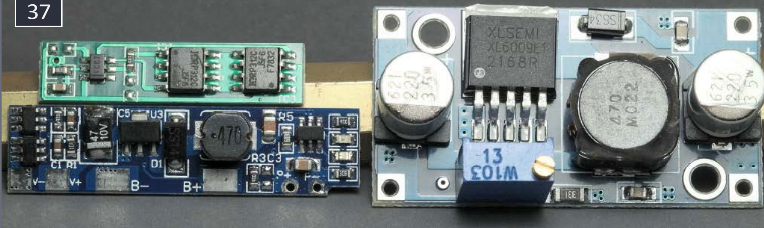
37. Battery manager (on left) and DC-DC converter.
