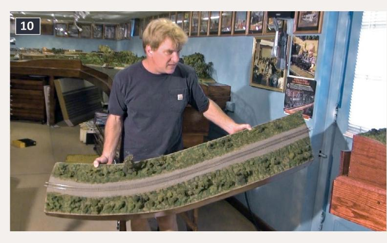
10. The removed sections has a safe place under the layout for storage and can be dropped into place at a moment's notice. Replace the pins and the rail joiners to have trains running in minutes.
