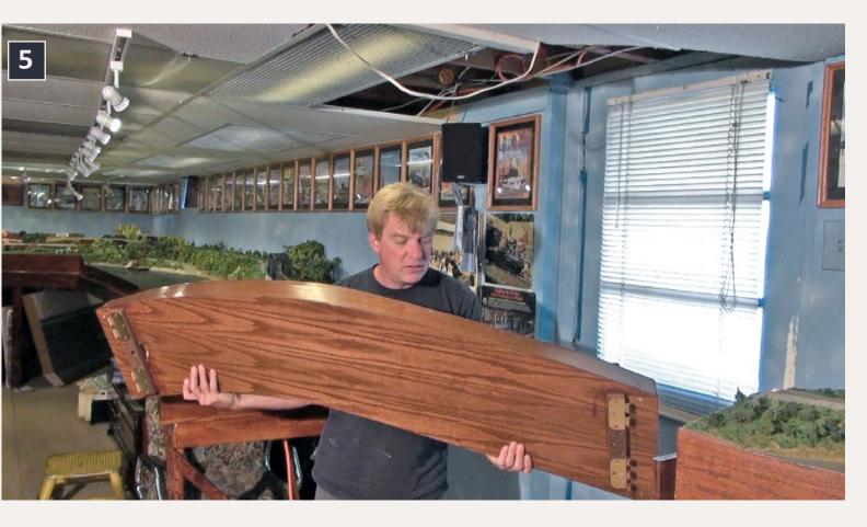
5. The liftout sits on top of mounted door hinges. This maintains the same alignment every time you install it, so the rail will match to the other segments. The door hinge pins hold everything tight when installed. To remove the section, pull the pins.
