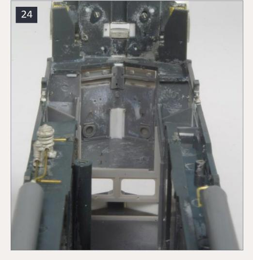
24. Inside of short hood built up with styrene.
