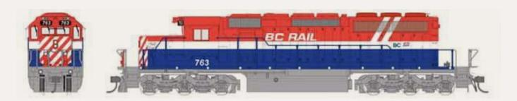
**Bowser** (bowser-trains.com) is producing a GMD version of a SD40-2 diesel locomotive. Rather than being a variation on a standard US production locomotive, Bowser developed the model as a Canadian-built GMD. Features include GMD-style steps, unique grab irons, an electric bell, special snow shields, an offset sill, and three operating class lights. It will be available for standard DC operation as well as with ESU LokSound Select for DCC.
