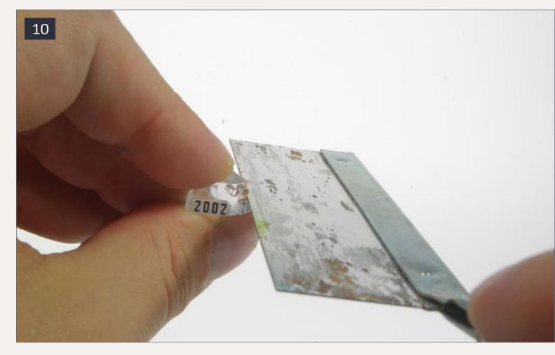
10. Cutting the rear headlight and number board casting.
