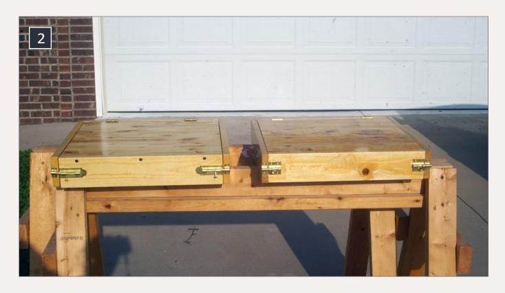
2. This is the workbench when closed. It's simply a box, 17½" deep, 19½" wide, and 3½" tall. The barrel bolts keep it closed, and also prevent the lid from closing too far and potentially crushing the contents. Attaching the box front to the lid leaves a convenient opening so you're not working down inside the box, while still having the other three sides to keep tools and parts from falling off.
