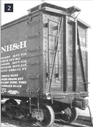
1. 36' Single-sheathed wood car with vertical steel bracing manufactured by Fowler Car Co. circa 1909.
