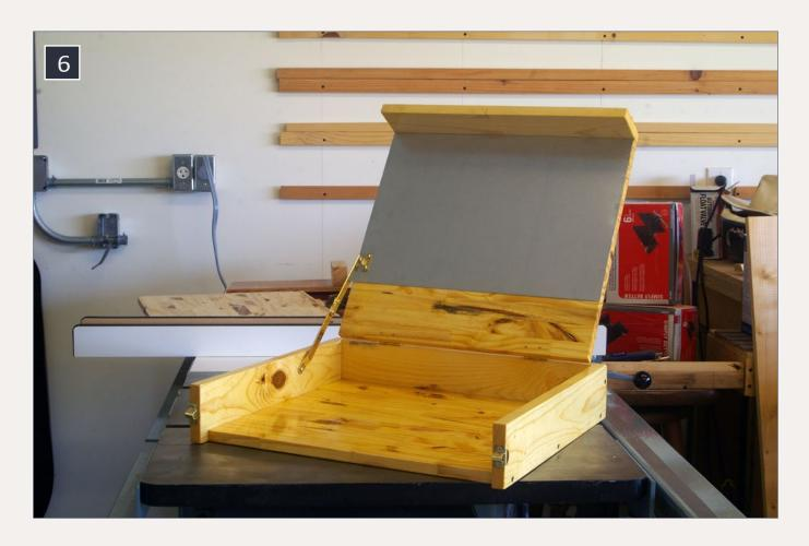
6. For the first workbench, I mounted the folding support bracket 5½" forward from the back edge of the top. Although it works, the top opens just far enough to make me worry the workbench could tip over backward. For the second one, I mounted the bracket ¼" farther forward, and you can see the resulting change in the angle.
