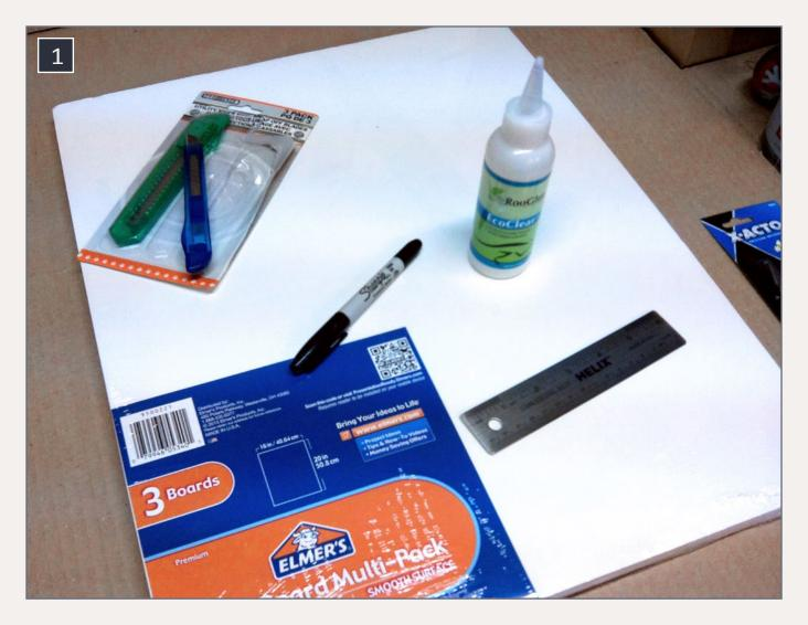
1. Shown are the basic materials necessary: some foam board and glue. A pen helps you mark where you will cut, a simple retracting knife does the cutting, and a straight-edge keeps the cut nice and straight.
