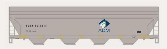
Center Flow covered hoppers. Introduced by ACF in the 1960s, the rounded body of the Center Flow design provided structural strength as well as an inducement to gravity unloading.
