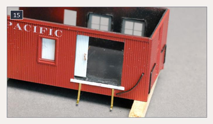
15. A cargo door was cut into the side of the caboose, and a pair of brass strip step supports were added just below the door, which later was swapped to an outside-hung version.
