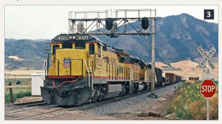
3. A Union Pacific freight rolls under a signal bridge on the nine-mile stretch of two main tracks at Blaser, ID in 1990. The bridge carries signals for traffic in both directions on both tracks. Josef Brugger photo.
