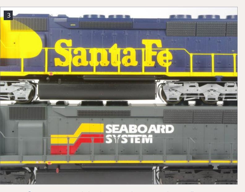
3. Comparison of the blower duct lengths on Proto 2000 SD45s.
