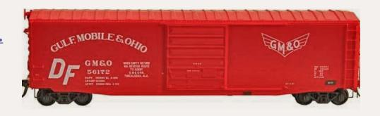
GM&O 50' boxcar with 9' Creco six-panel doors. The HO scale ready-to-run model is based on a 1961 prototype that was repainted in January 1969. Note that the car has a full height ladder on the right but no running board.
