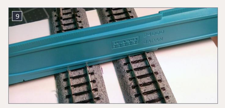
9. With the first track in place, use the Kato rerailer to position a second track – if you're going to have any double track – at exact the right position.
