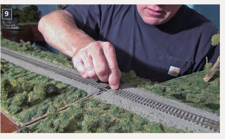
9. The section is made up of foam sheets cut to the contour of the main line curve, with six inches of scenery on each side of the track. The ¼-inch plywood is oak. It's wrapped around the foam and glued in place to form the curved sides and flat bottom. Everything is stained, and finished with polyurethane.
