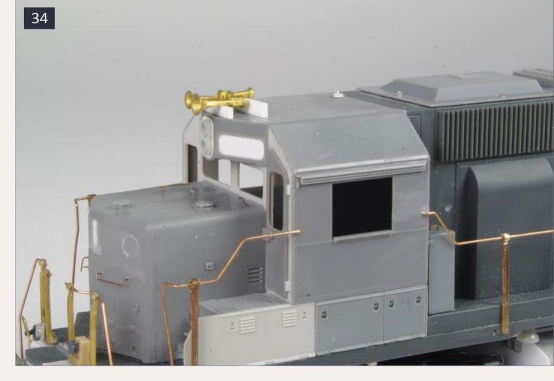
34. Using pieces of styrene to hold the horn in place while the glue dries.
