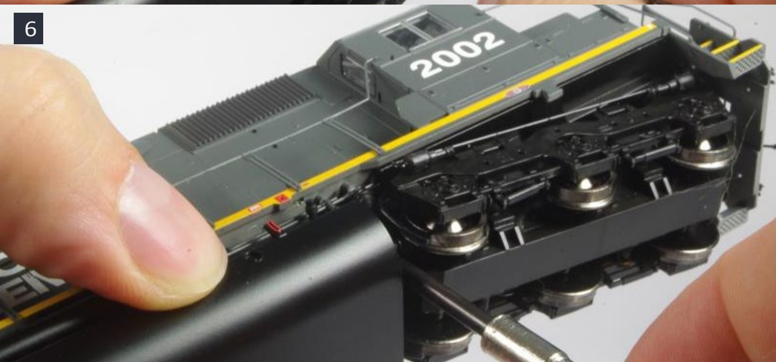
5-6. Removing the rear and front screws which secure the shell to the frame.
