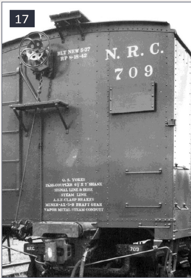
17. Flat steel end fabricated with three vertical panels on express car built by Pullman-Standard in 1937.
