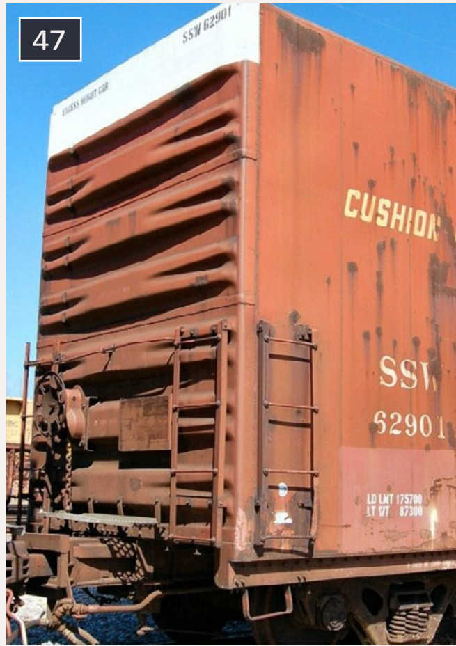
47. The 2/2/3 ends on this Cotton Belt car built in 1979 feature split or bifurcated ribs.
