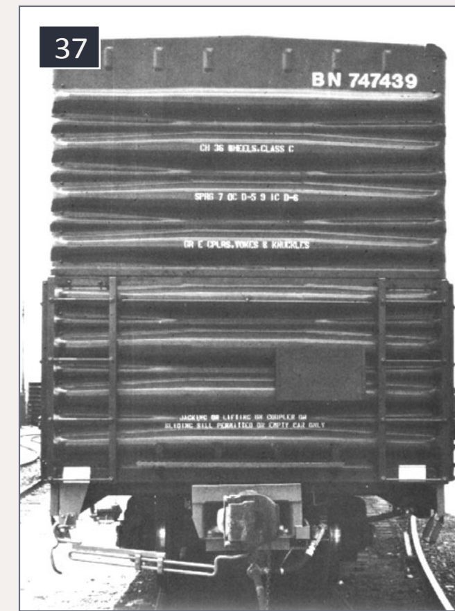
37. Improved Dreadnaught end on car built by Pacific Car & Foundry. Note non-tapered top rib and six small vertical indentations in the hat section.
