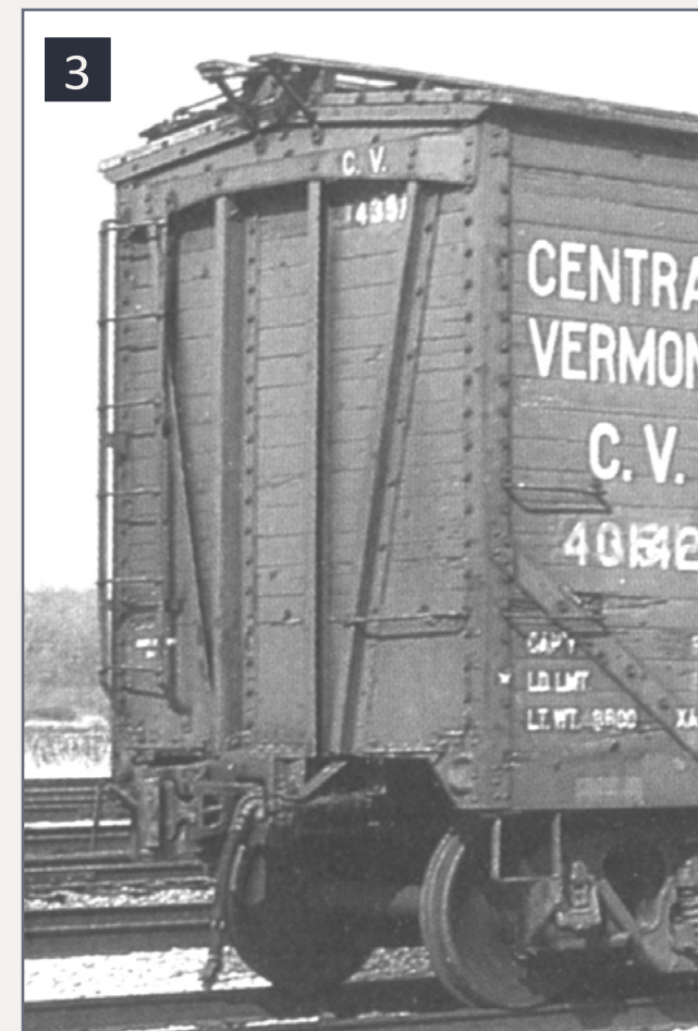
3. Single-sheathed wood car built in 1925 with steel end bracing in a 'V' pattern. Note the protective shield over top of steel bracing.
