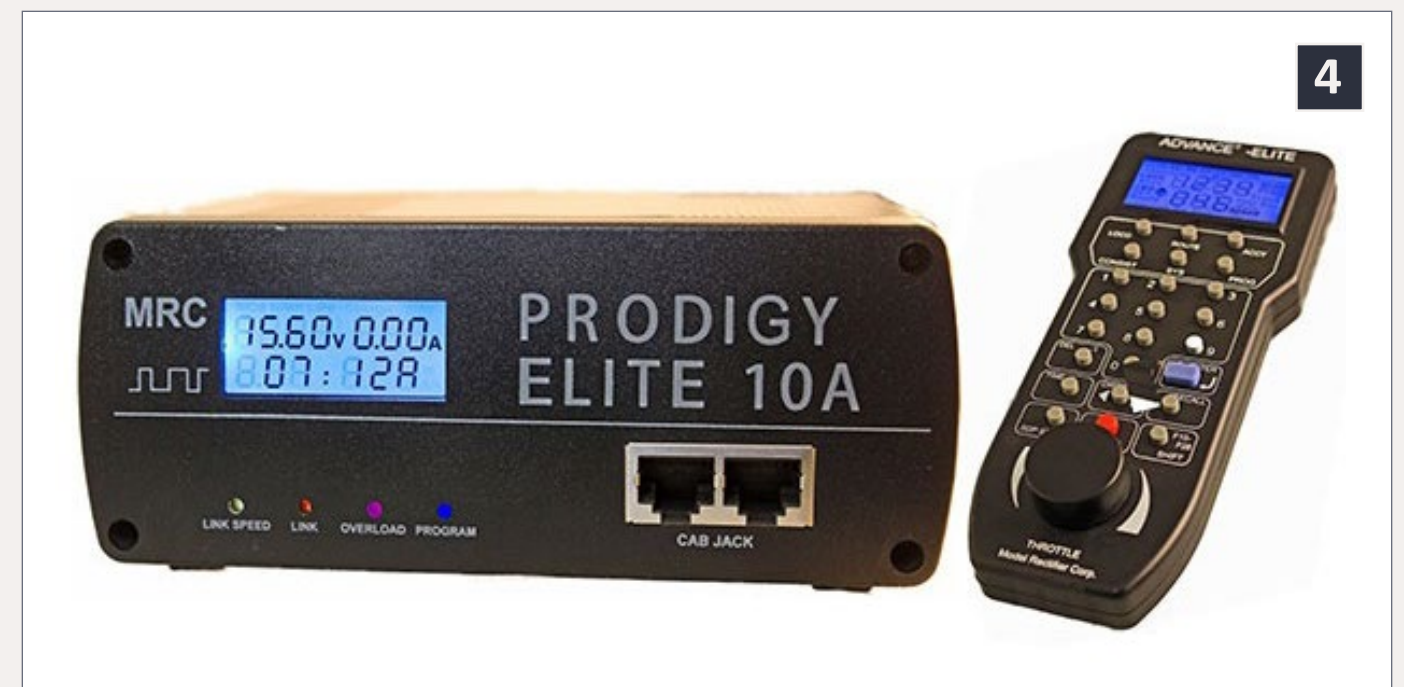
4. MRC Prodigy Elite 1 to 10 amp system. MRC photo.
