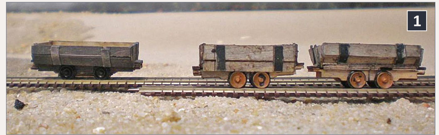
1. Two BTS mine cars that have been modified to represent the smaller 2½ ton cars used at mines on the East Broad Top next to an unmodified car for size comparison.
