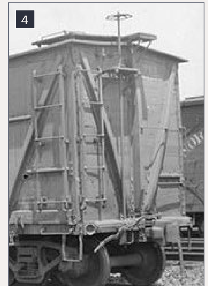
4. Distinctive 'V' braces with a single vertical brace in the center of the end.
