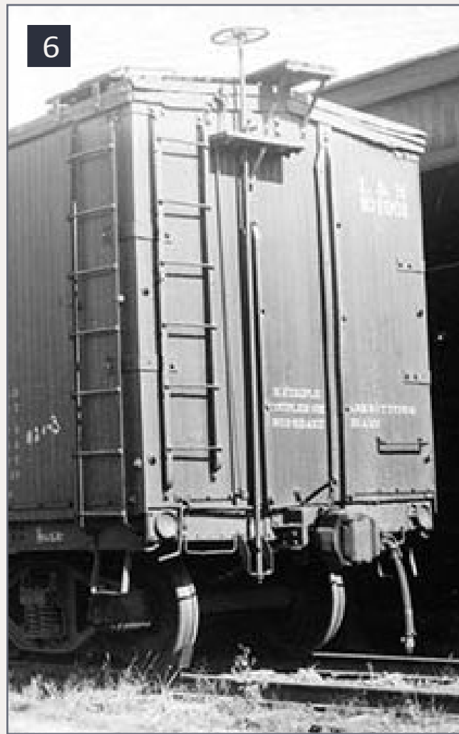
6. Double-sheathed wood car with unique vertical braces.
